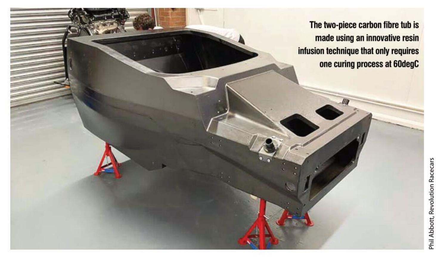
'Ours is the first time the infusion technique has been used on a crash box,' notes Abbott. 'We had to do a lot of pretesting of components, and then crash the complete structure and measure it to get the required result. It wasn't a long process, it was swift, and we were very close the first time.
