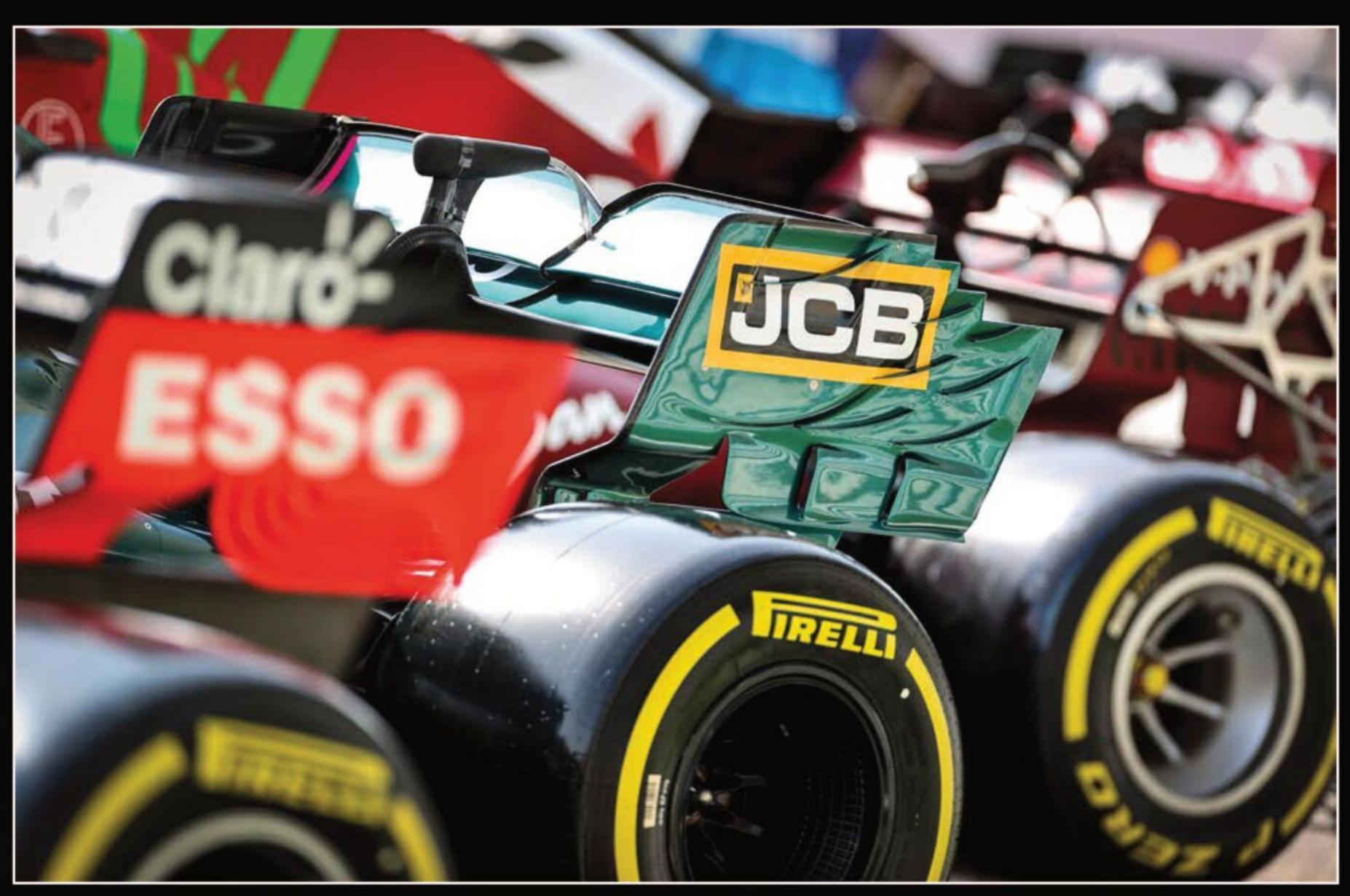
Pirelli had to make changes to sidewall construction for its latest generation of tyres for Formula 1, and each tyre is now heavier than those used in 2020
