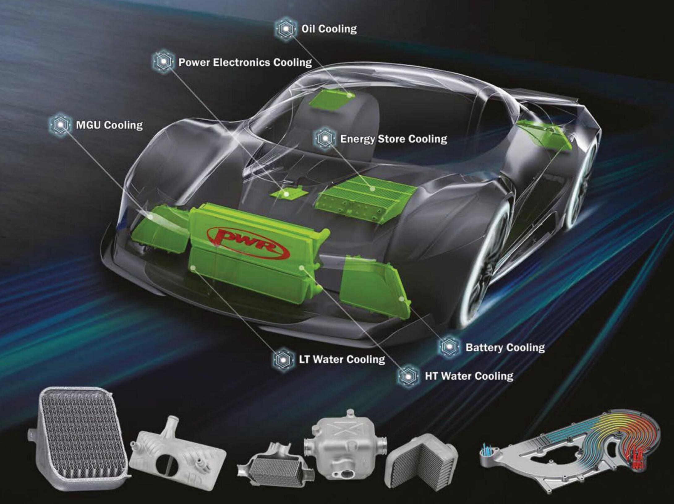
PWR has partnered with VELO3D using their Sapphire machine technology and unique "SupportFree" processes enabling class leading thin wall capabilities and high quality surfaces without porosity. PWR manufacture higher quality internal channels, flow paths, and high aspect ratio walls for new designs that optimize heat transfer.
