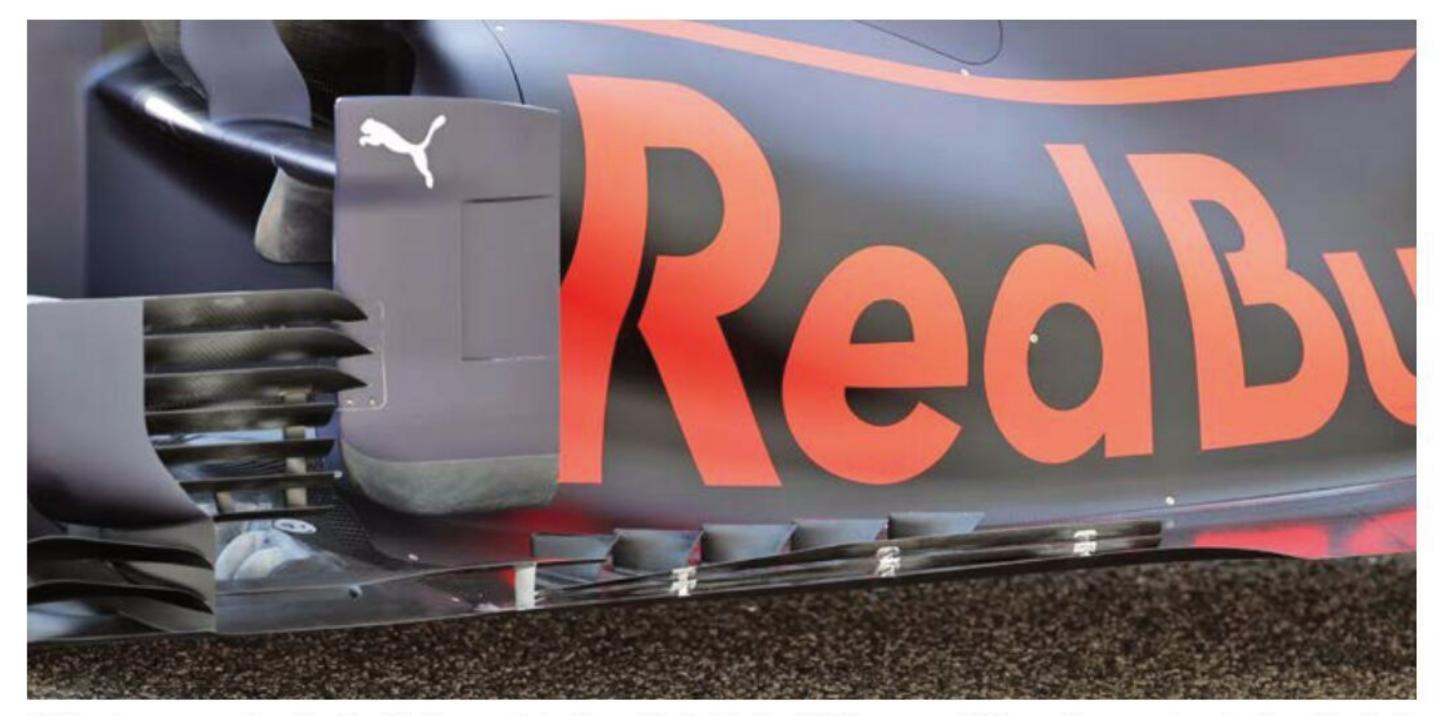
High-rake cars, such as the Red Bull, seem to be less affected by the 2021 aero restrictions. Car was clear leader at the test
