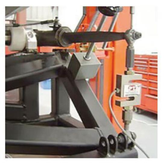
Figure 5: Anti-roll bar stiffness test bench with moveable arm (thanks to an adjustable rod length) on the left and measurement of the force on the right
