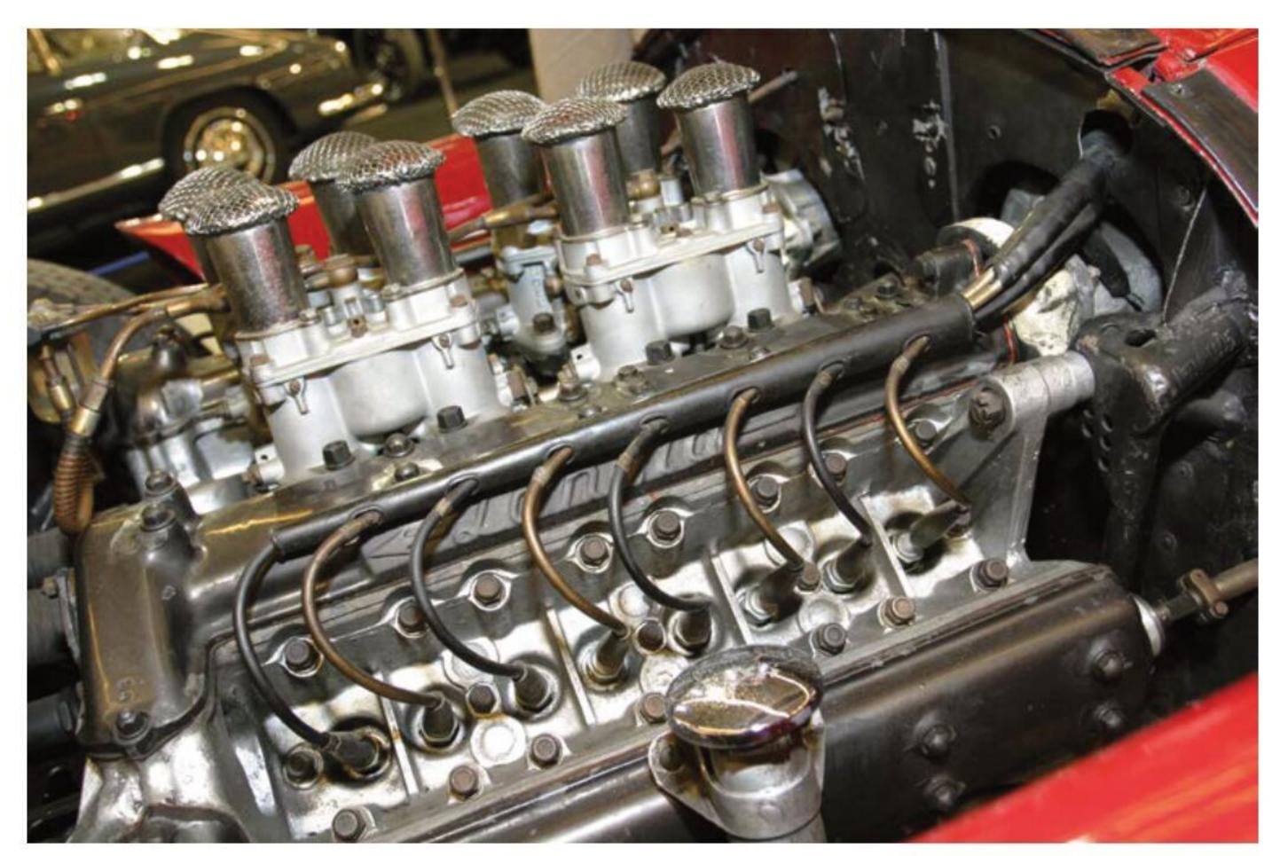
It featured a 90-degree bank angle, gear-driven dual overhead cams, four 40mm Solex carburettors and twin-spark ignition
