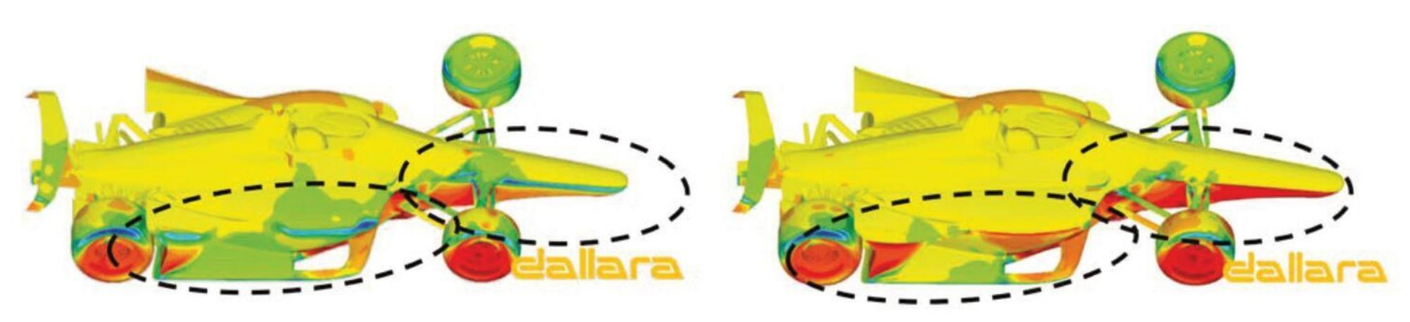
Figure 12: Effect of stability wickers on the leeward flip scenario. With no reduction in performance, these simple additions were deemed a resounding success
