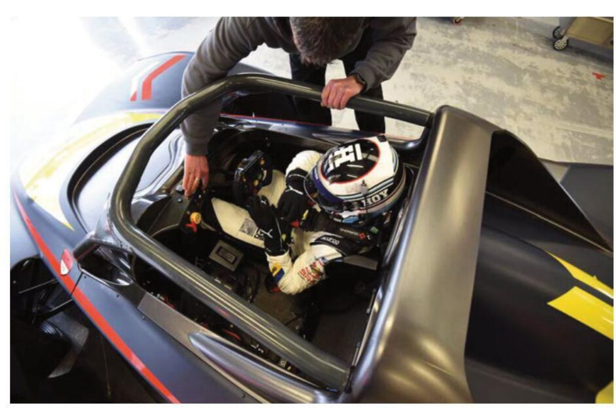
A unique double halo concept was developed for additional safety and object intrusion protection
