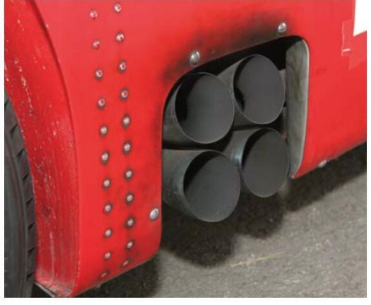
The Ferrari-modified cars featured this new, dual quad, open stub exhaust, which made the V8 engine sound absolutely brutal
