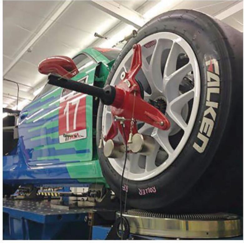
Figure 6: Measuring anti-roll bar stiffness on a K&C test bench
