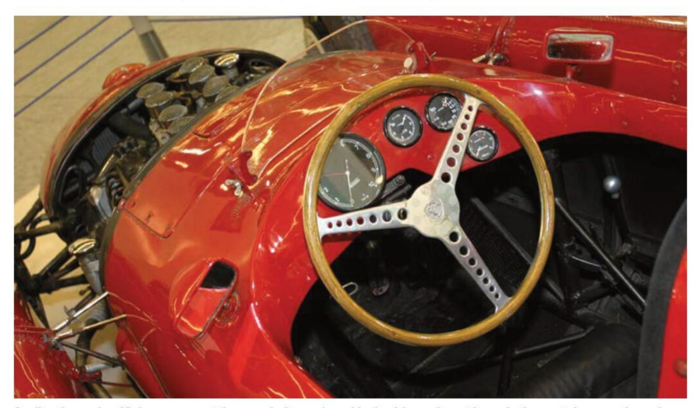
Angling the engine 12 degrees meant the propshaft ran alongside the driver, who sat lower in the car to improve the c of g
