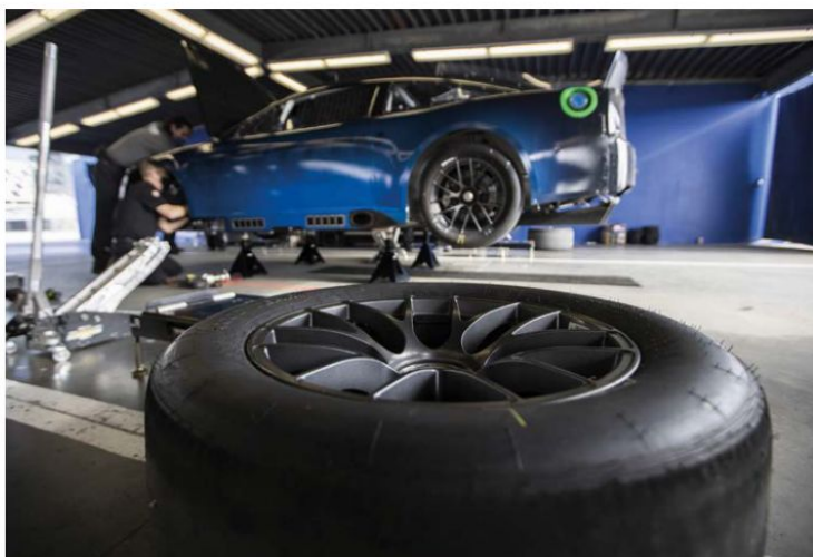
Wheel size has increased from the traditional 15 to 18in, changing the way the Goodyear rubber will perform on all types of circuit
