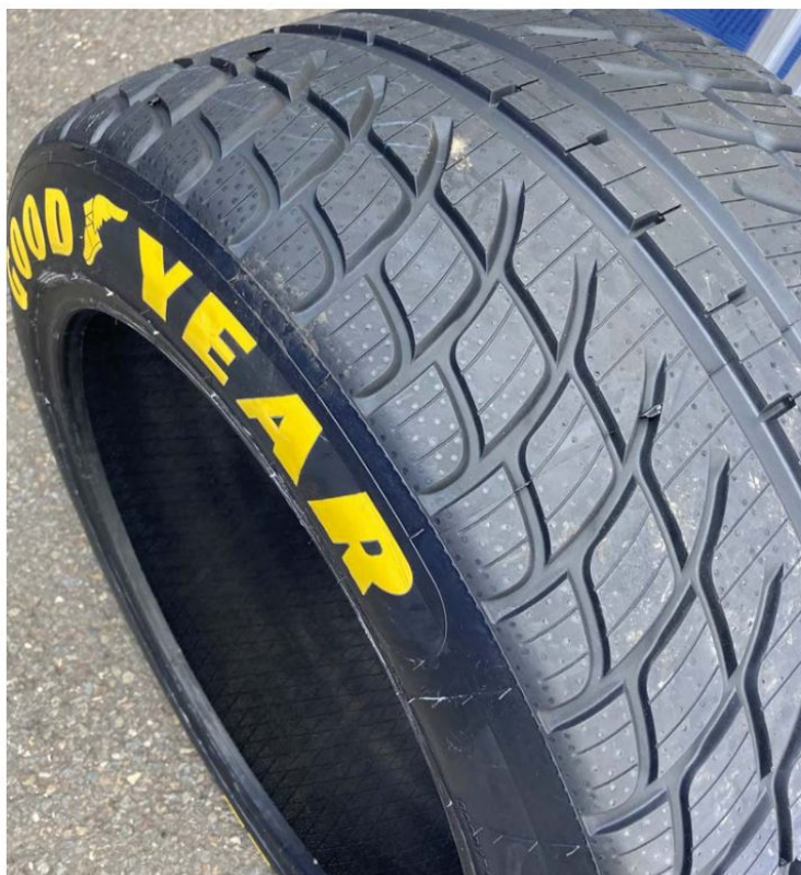
Goodyear's new wet construction features moulded tread technology, where previously the grooves were hand cut into the tyres
