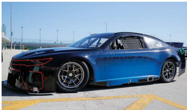
New composite body shape is symmetrical, unlike previous generations, and was designed in CAD simulation
