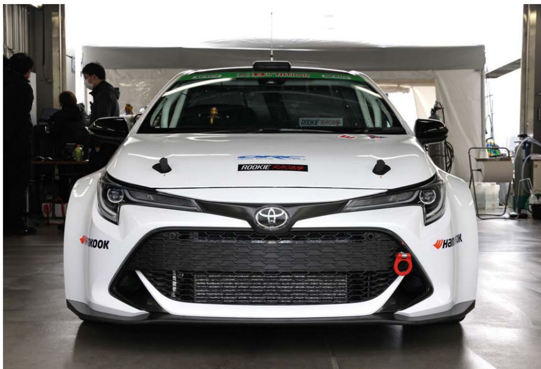
Car has Toyota's four-wheel-drive system and one of the company's 1.7-litre, three-cylinder, turbocharged engines and uses hydrogen fuel from the Hydrogen Energy Research Field in Fukushima
