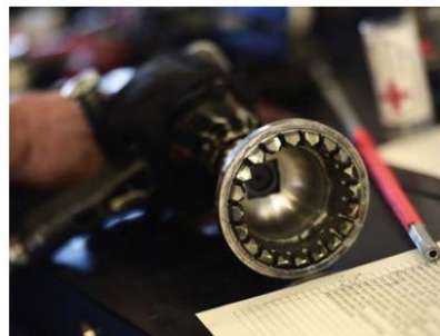
One of the minor detail changes for 2022 is the switch to a single, centrally-mounted lug nut to hold the 18 x 12in wheels in place
