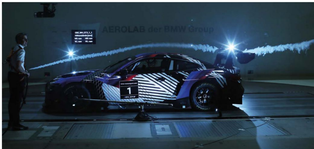
Both downforce and drag have been improved over the outgoing M6, making the car more efficient overall, but also with a view to being more manageable in the hands of amateur drivers
