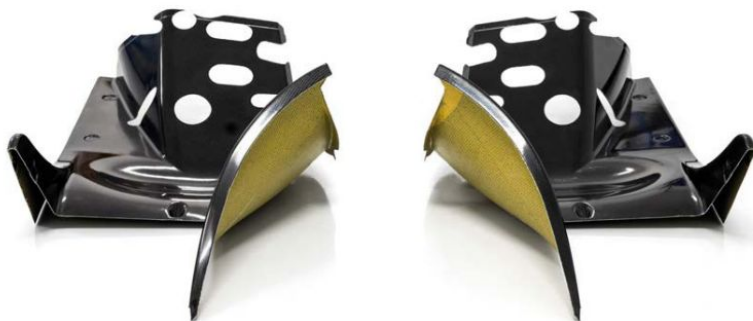
An example of carbon Kevlar construction body panels on the Brabham BT62 C. Carbon provides the strength, Kevlar the resilience
