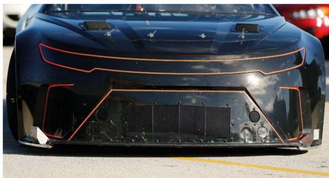
Cars are lower and wider than Gen-6, but ride 2in higher. Aero details include a carbon undertray and stepped splitter
