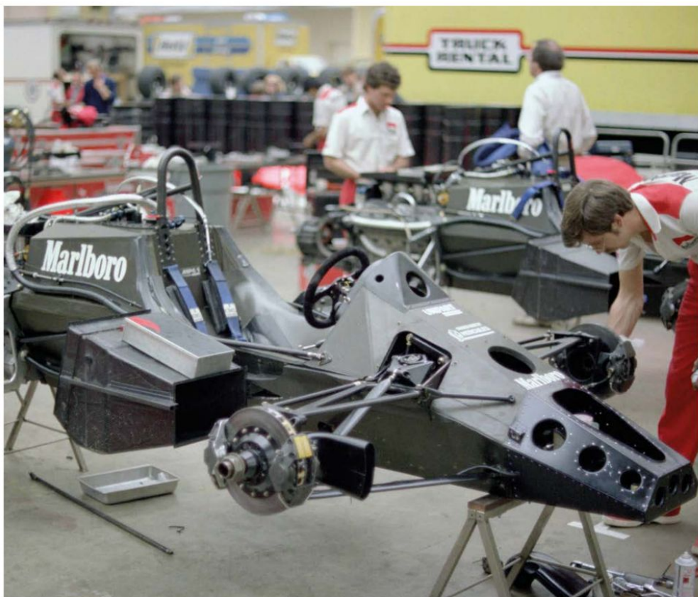
Where it all began. The McLaren MP4 of 1981 was the first racer to successfully use carbon chassis construction, although it took an aerospace technology company to bring the radical ideas of its designers, John Barnard and John Webb, to life
