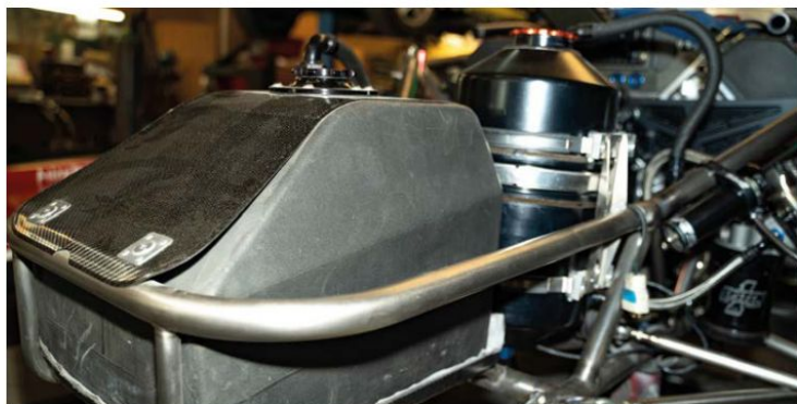
A recent rule change allows the front chassis section to now be fabricated from titanium tube, bolted to the chromoly frame rails
