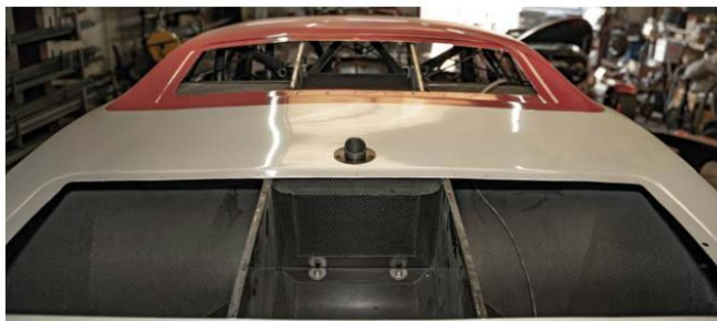
Carbon and Kevlar bodywork is attached at the rear to carbon honeycomb spines, optimised through FEA analysis
