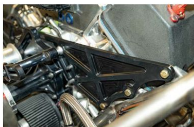
New FEA-designed engine support plate is pocket milled for weight loss
