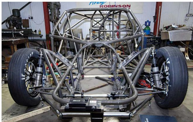
Old car chassis showing previous front suspension support arrangement, which was later found to be flexing fore and aft
