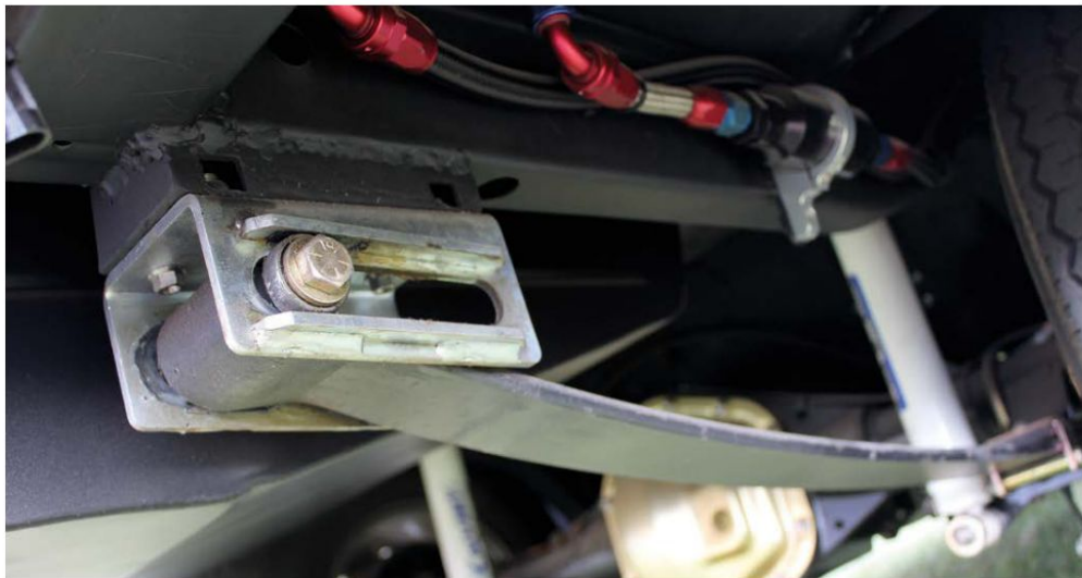
Leaf spring slider shackles are designed to offer a more consistent spring rate and eliminate any potential bind with regular shackles. Note this system is using a monoleaf spring
