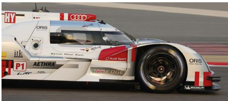
Various approaches have been taken to hybrid powertrains. The Audi R18 used the front axle to deploy and harvest kinetic energy
