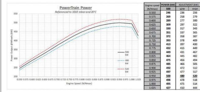
Figure 1: LMH power curve provided by the rule book (sum of power measured at each driveshaft)
