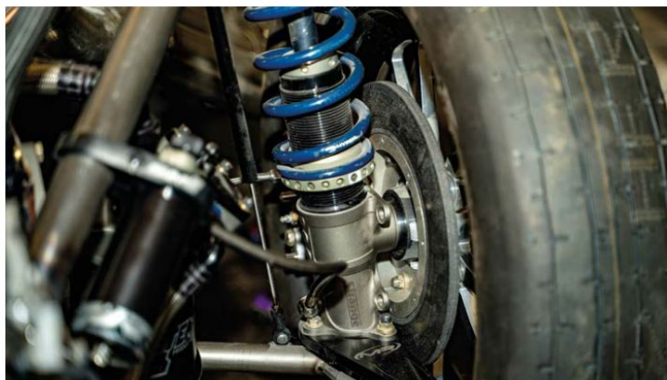
Coilover front suspension use Strange Engineering bodies and Penske internals, with double the stroke of previous iterations
