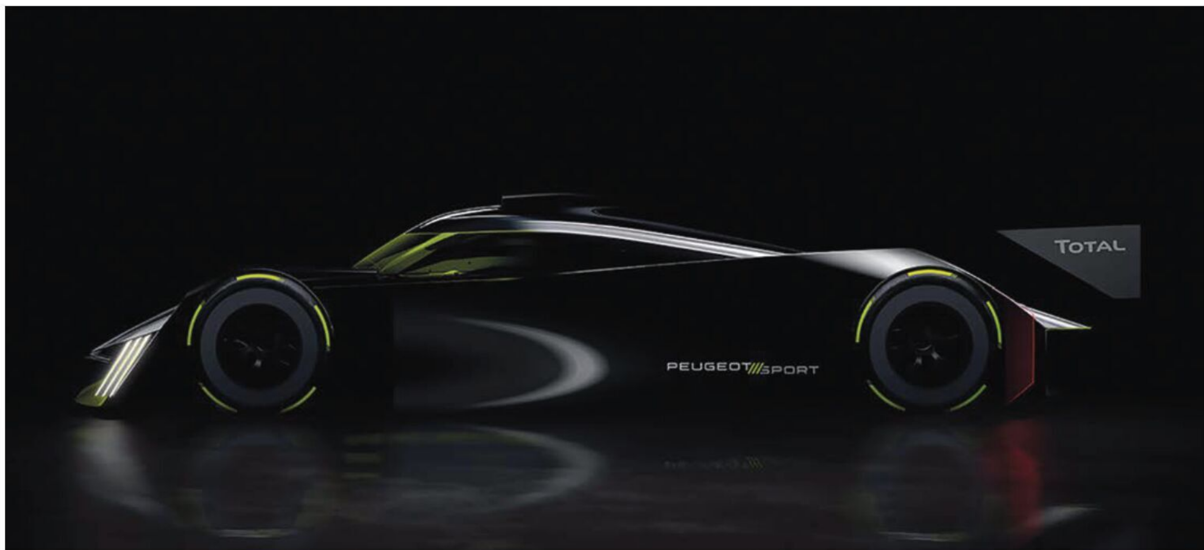
The concept car displayed has no rear downforce generator, though the finished racecar is likely to have a flap at the back to help trim and balance the car as the race team seeks to control the ground effect and maintain optimum downforce in all conditions
