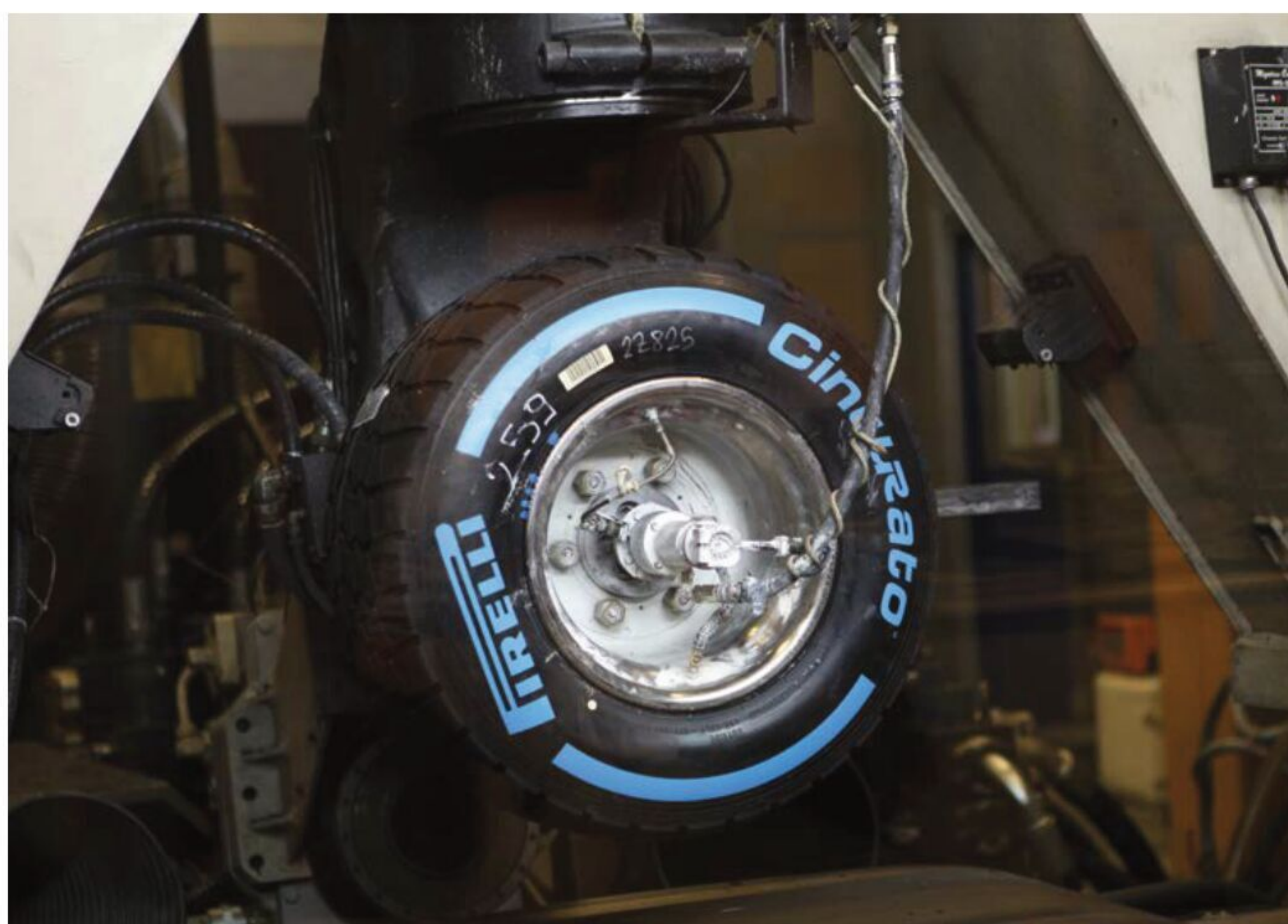
The new tyres started as finite element models and, only when approved by the FIA and the teams, did they become physical tyres
