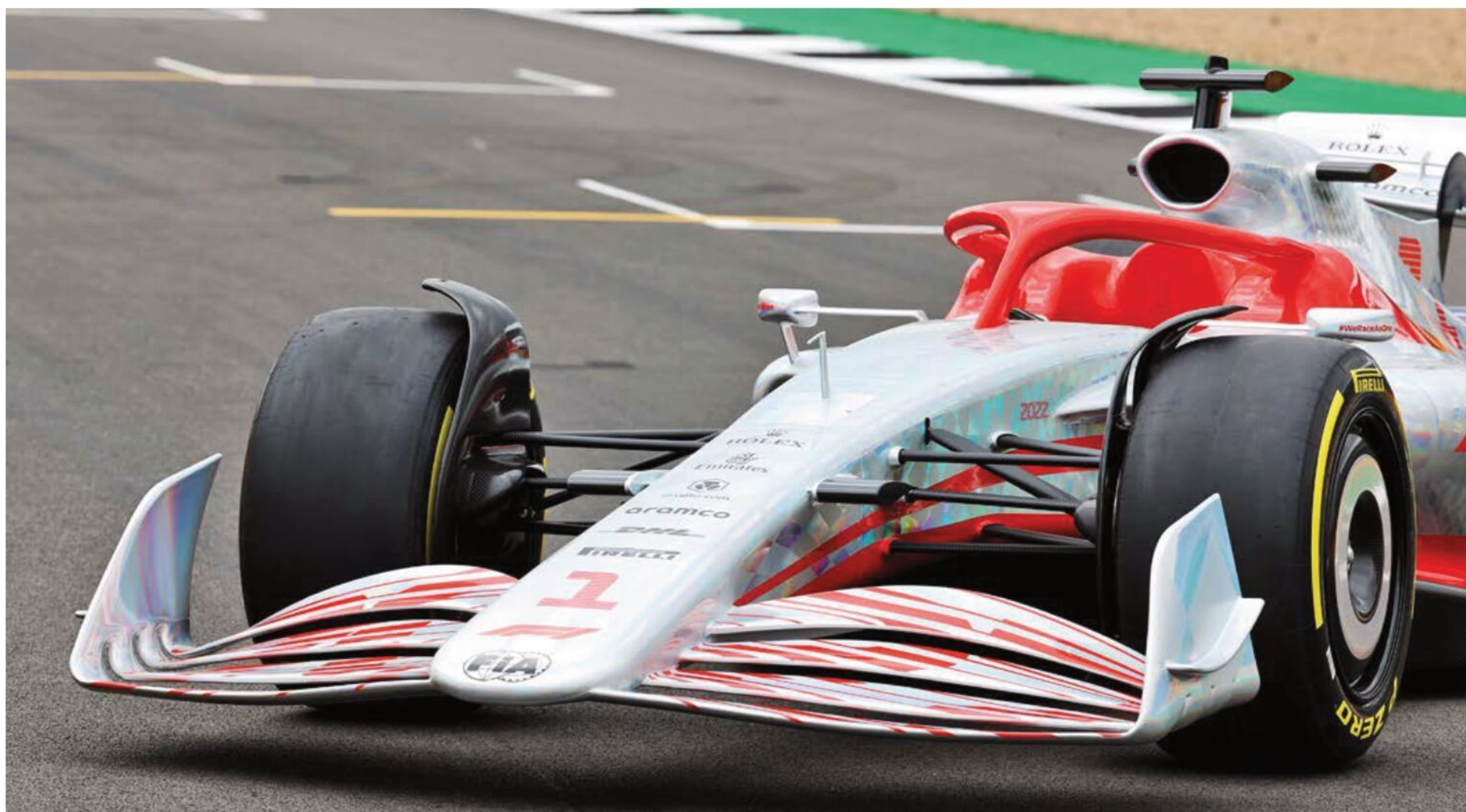
The increased diameter of the new 18in tyres (up from 660mm to 720mm) has broad design implications, as does the increased distance between the brakes and the rim of the larger wheels
