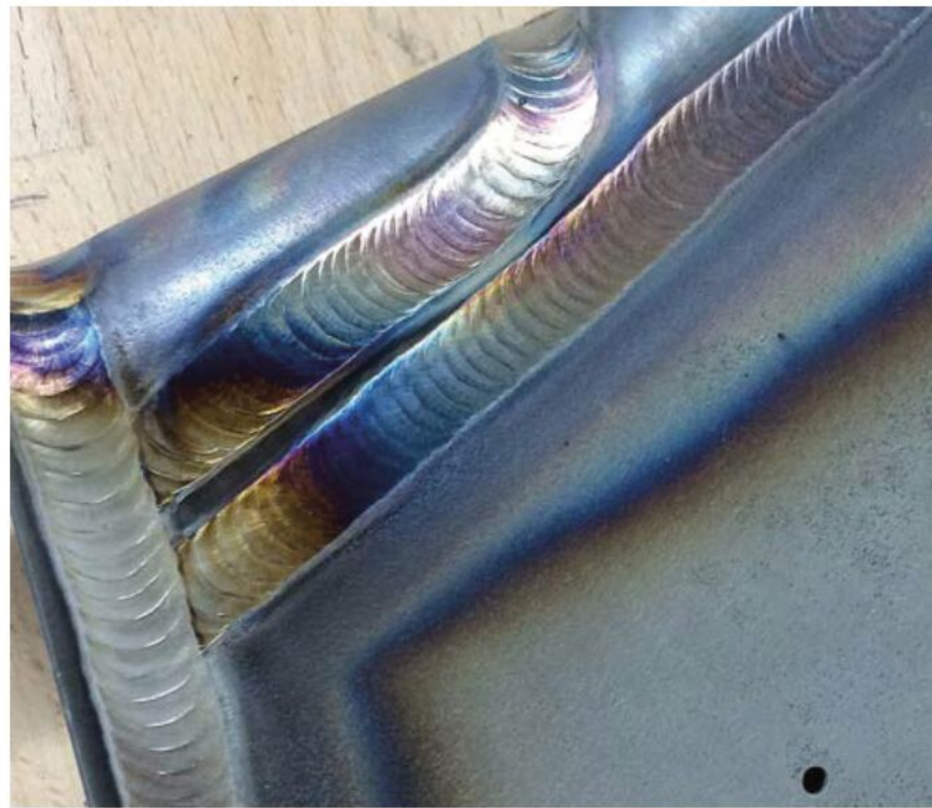
Instagram-worthy (!) detail of TIG welding on a wishbone from a Dakar racer. It is made of extremely heavy duty 15CDV6 steel with over 3mm material thickness
