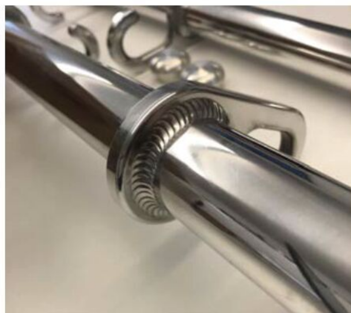
More F1 pit equipment. This is part of a TIG-welded assembly designed to lift the chassis when the rear end of the racecar is removed
