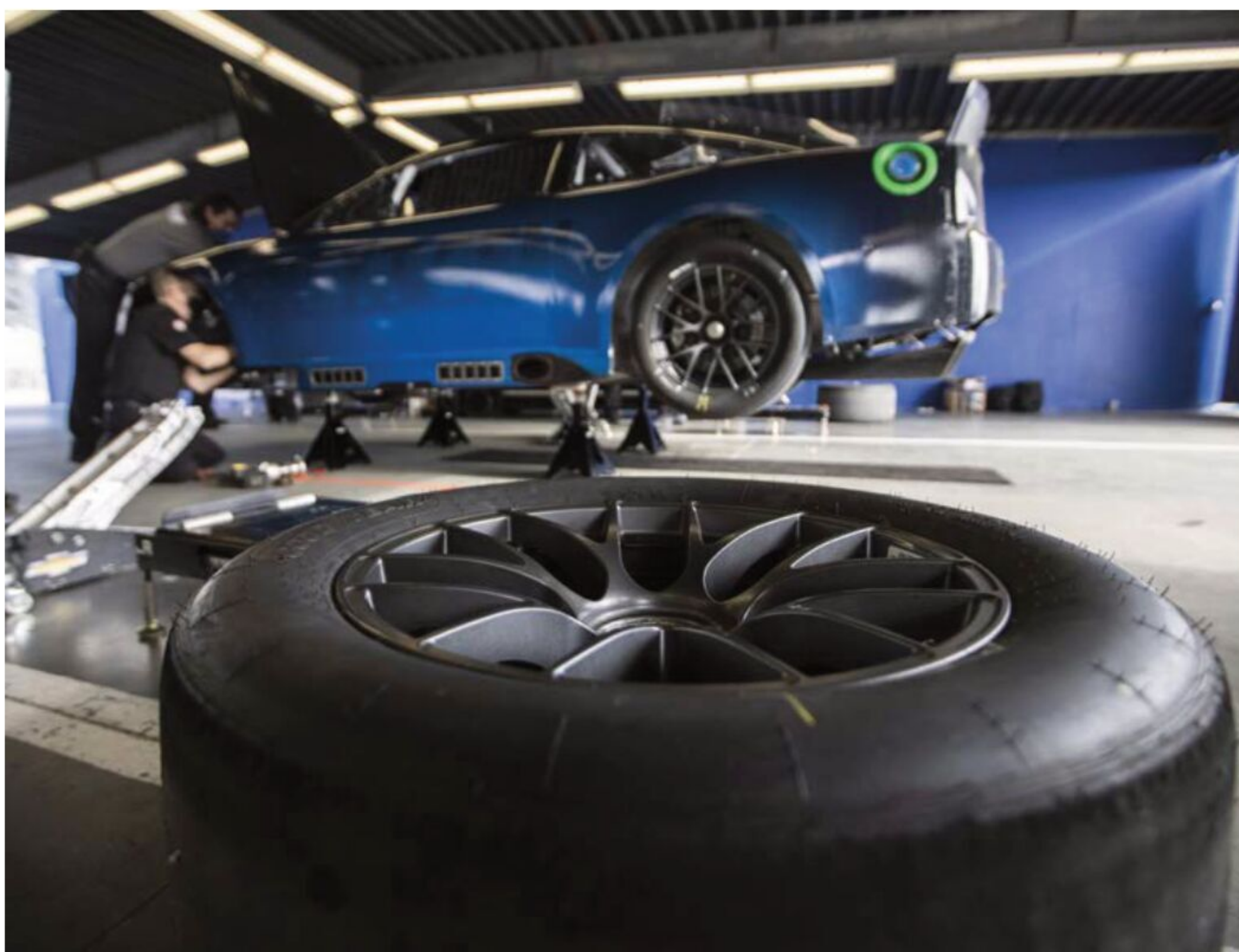
Gone are the old, traditional 15in steels on the Gen-7 NASCAR, replaced with wider, lighter, 18in aluminium racing wheels
