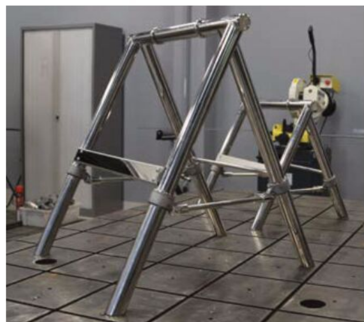
A motorsport fabricator will often be called upon to make pieces of pit equipment, such as these polished stainless steel chassis stands
