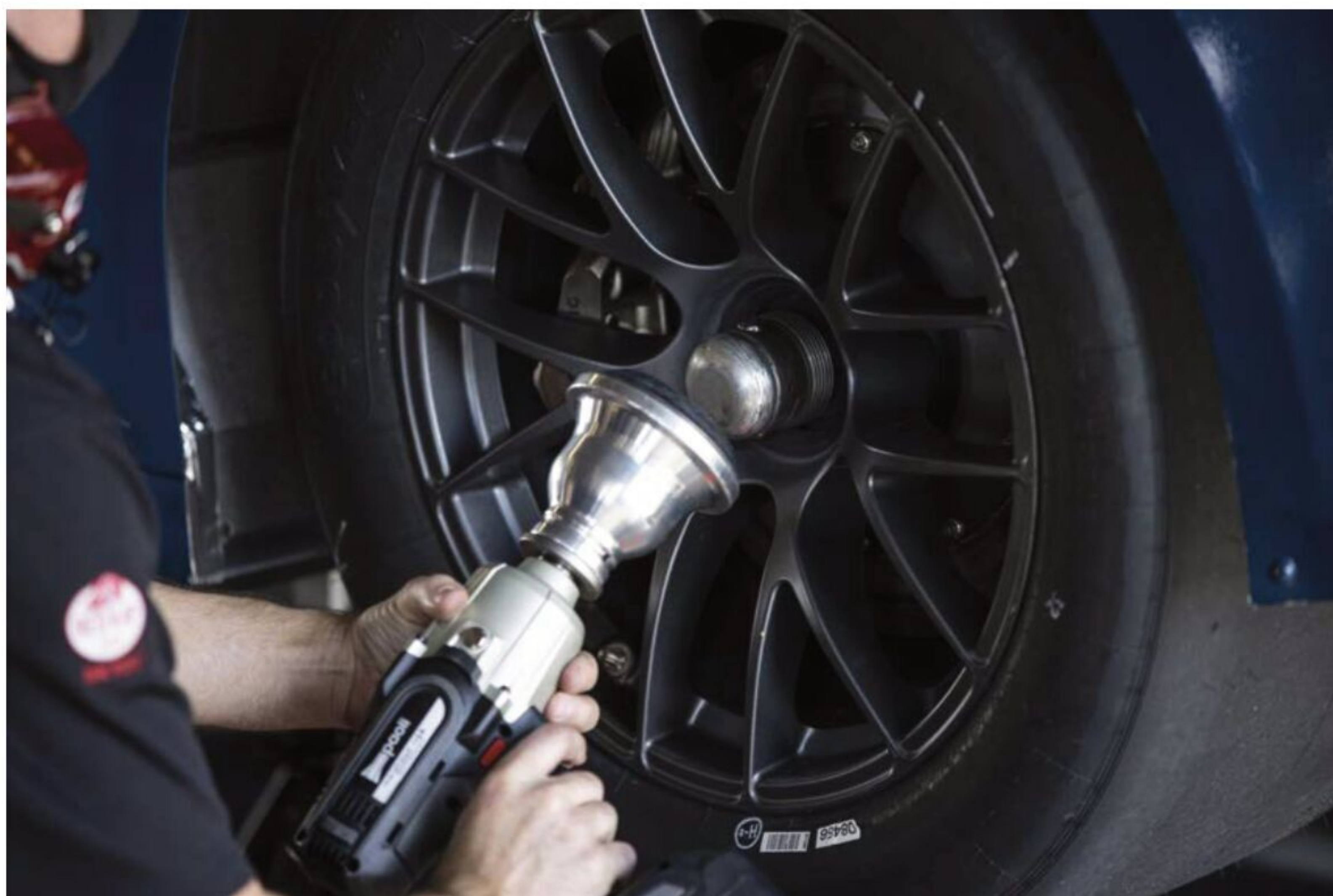
New single centre lock wheel bolt will speed up tyre changes, but there is no increase in the target for tyre longevity, which remains at one fuel stint
