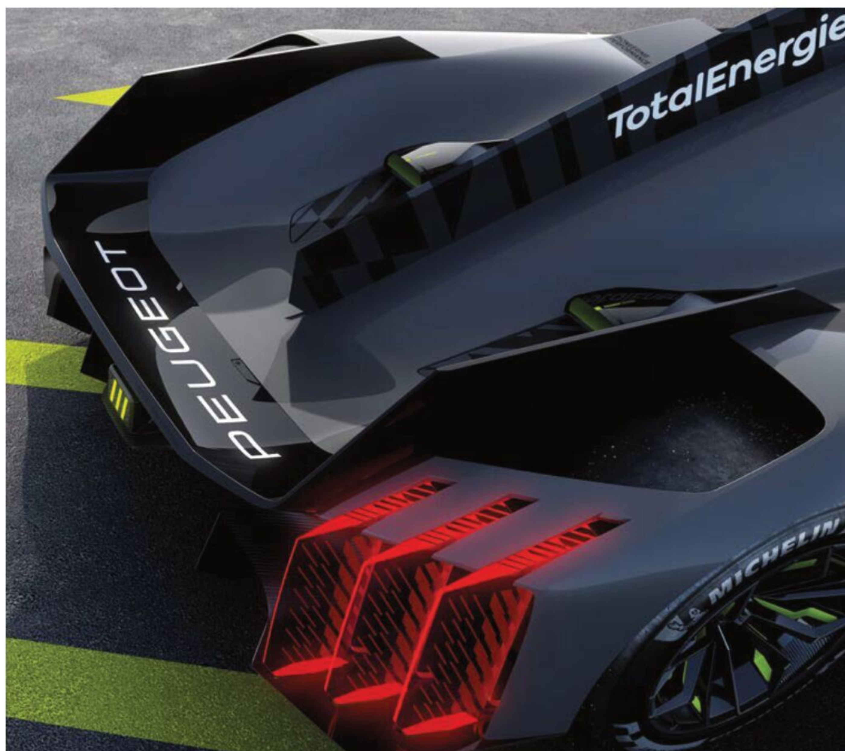
The concept car displayed has no rear downforce generator, though the finished racecar is likely to have a flap at the back to help trim and balance the car as the race team seeks to control the ground effect and maintain optimum downforce in all conditions
