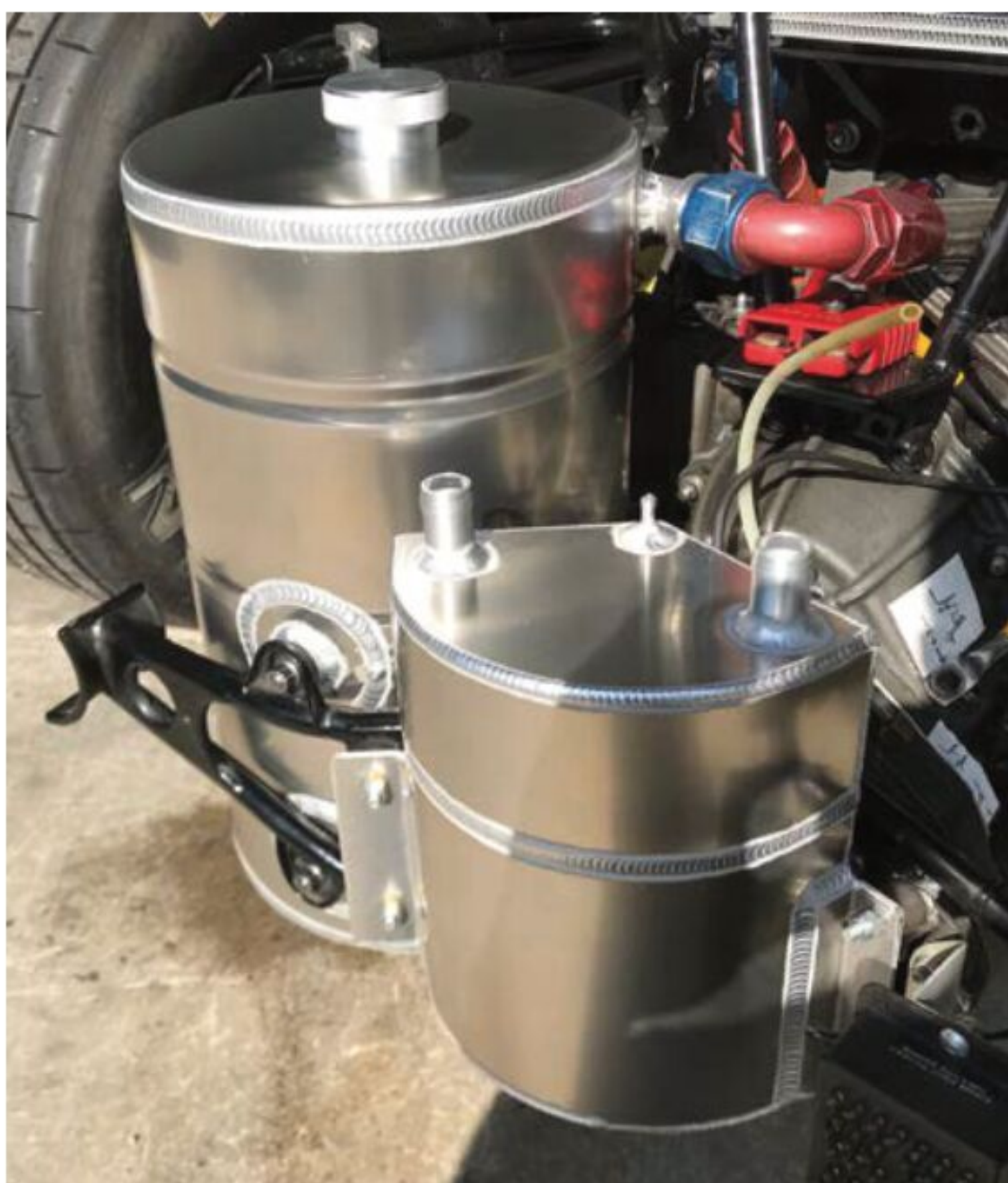
Old school fabrication is a major part of historic race preparation. This is Lofthouse's work on a 1970 McLaren M14a oil tank and breather pot
