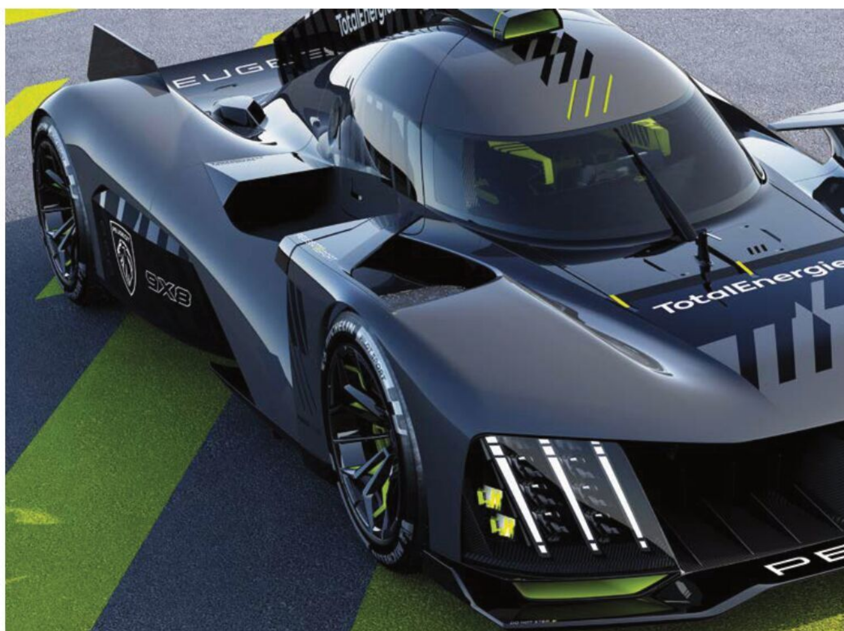
Large scoops behind the cockpit serve for cooling purposes, although debris ingress is a primary concern for the design team
