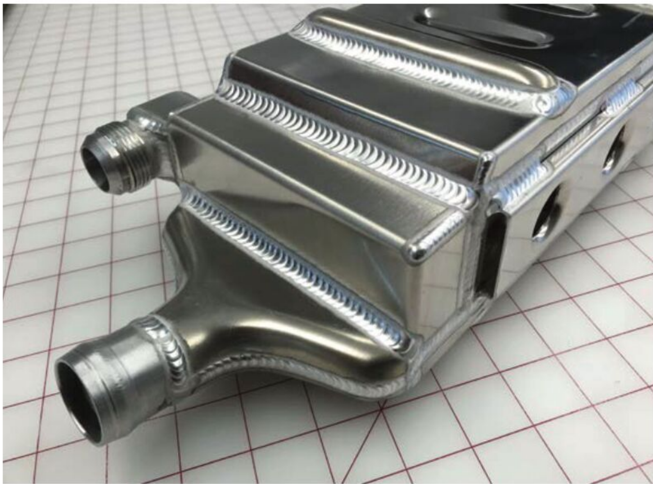
A fabricated Williams FW07 oil / water heat exchanger, which is identical in every respect to the original. It features an internal oil cooler core with water jacket
