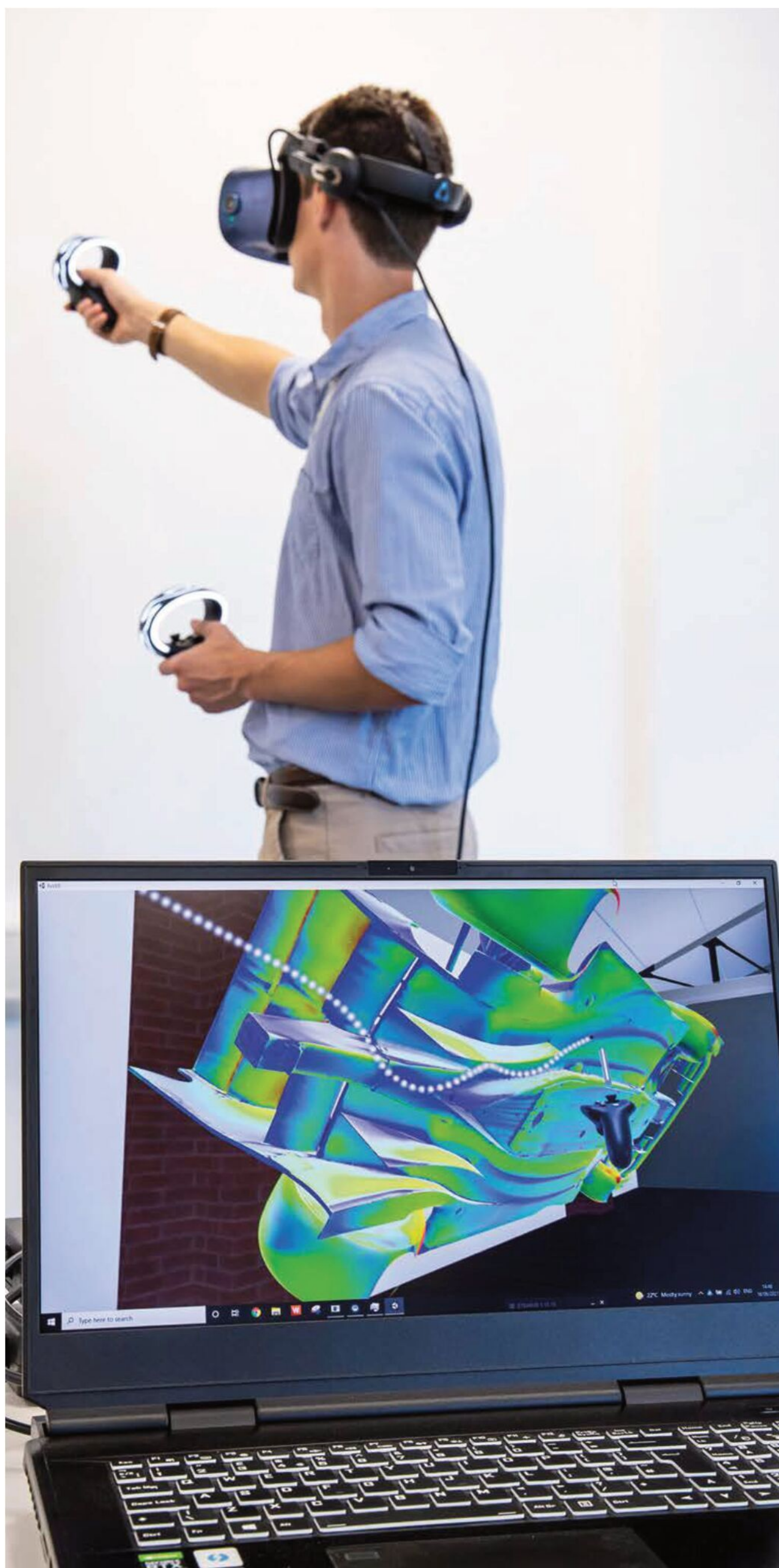
Turning on the virtual smoke machine, we can see flows along the underside of the car, with the model hovering above our head
