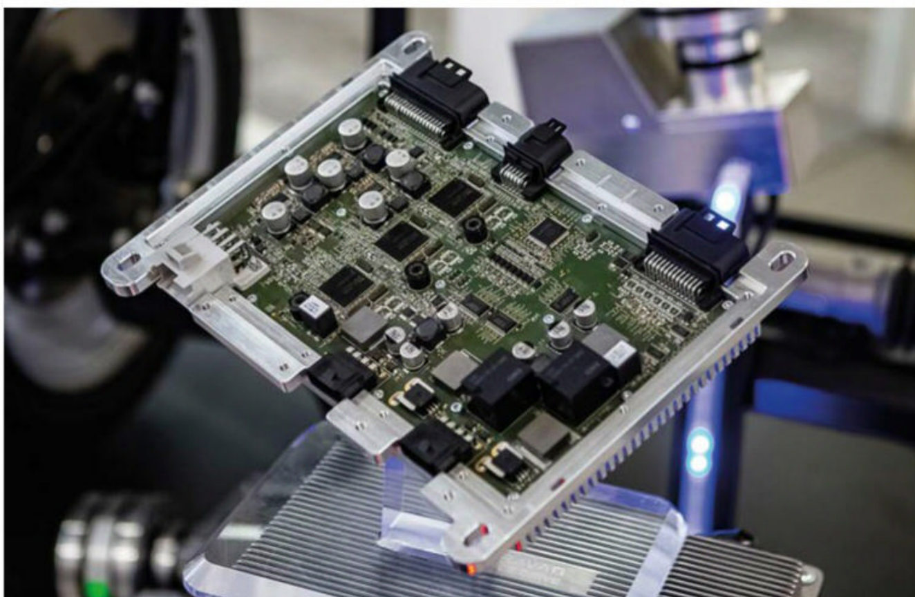
Schaeffler's Space Drive is a key part of the DTM Electric concept, allowing the car's steering to be entirely controlled by electronics
