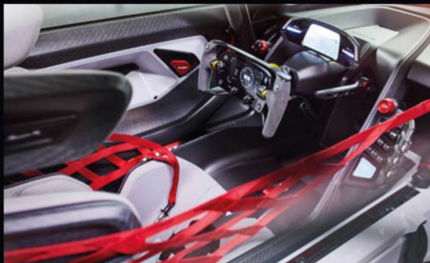
The seat, steering wheel, controls and 'screen all lie on the same axis for driver comfort
