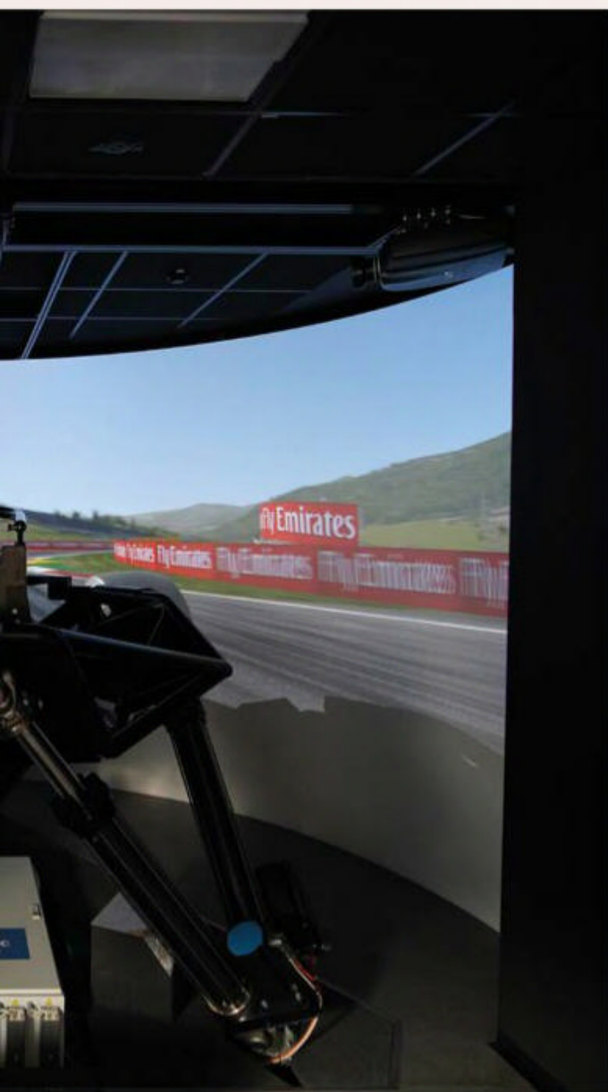
(Left) AVL's simulator is supported by market-leading software that allows for highly complex calculations to take place. The simulator itself can be wirelessly connected to a physical car in another building or another town. It is versatile enough to develop tyres and different concepts of cars, crucial in terms of accurately balancing GT3 cars for the DTM
