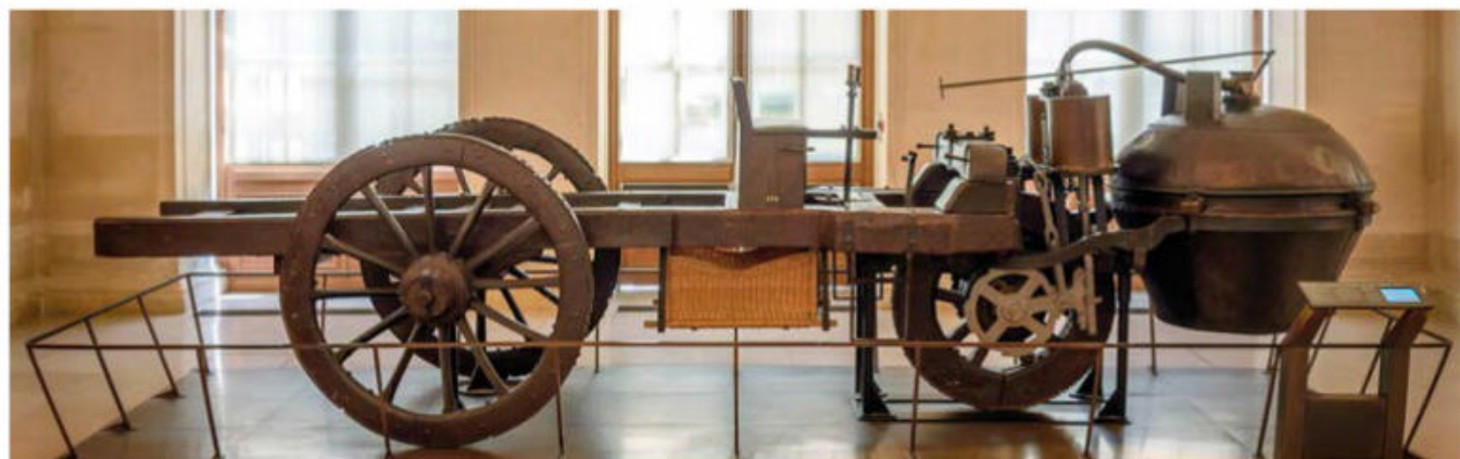
The earliest in-wheel motor, Nicolas Cugnot's 1769 Fardier à vapeur , used a ratchet to convert reciprocating motion into rotary motion
