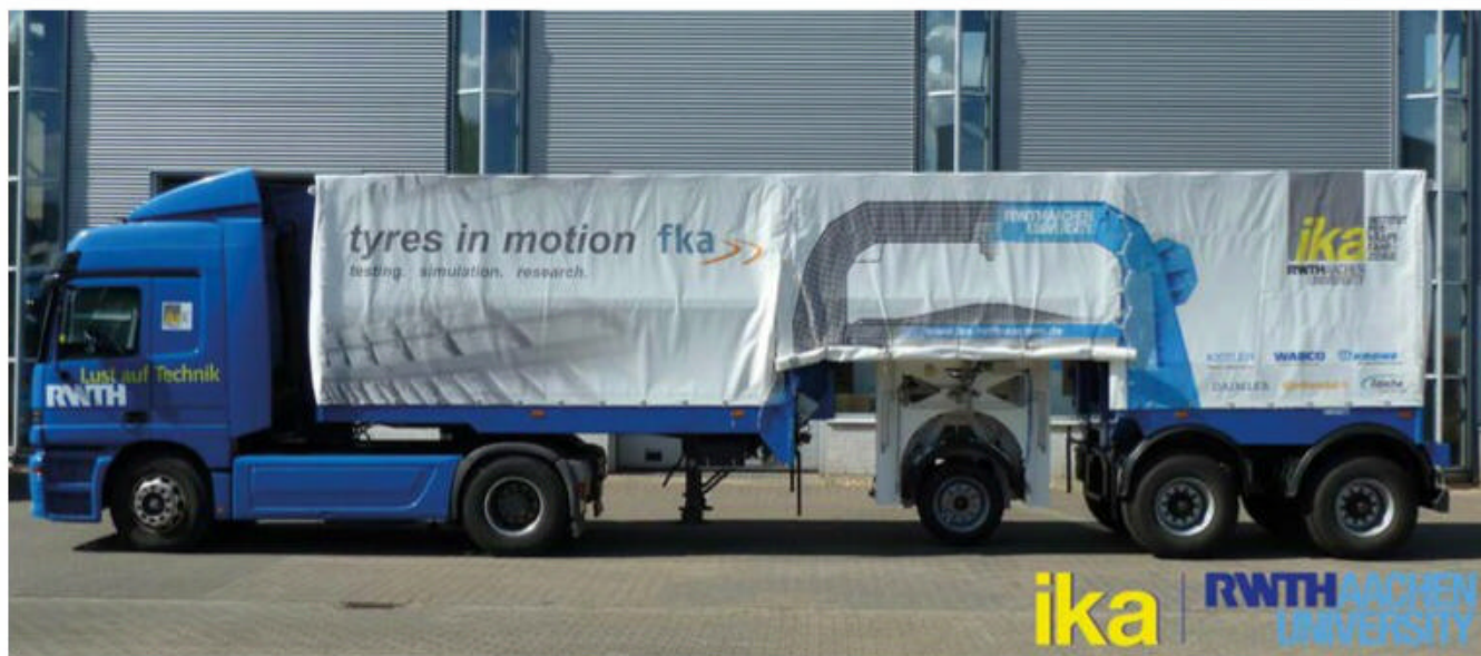
Fig 3: Example of outdoor tyre testing equipment where the tyre rolls on an actual road surface, seen here on this articulated truck rig from the Institute for Automotive Engineering (ika) at RWTH Aachen University. Both methods have their advantages
