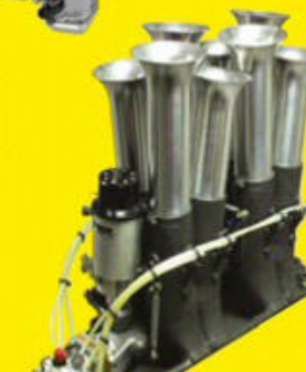
Kinsler GT Porsche ITB's. We partnered with Ed Pink Racing Engines to design "Direct To Head" ITB package.
