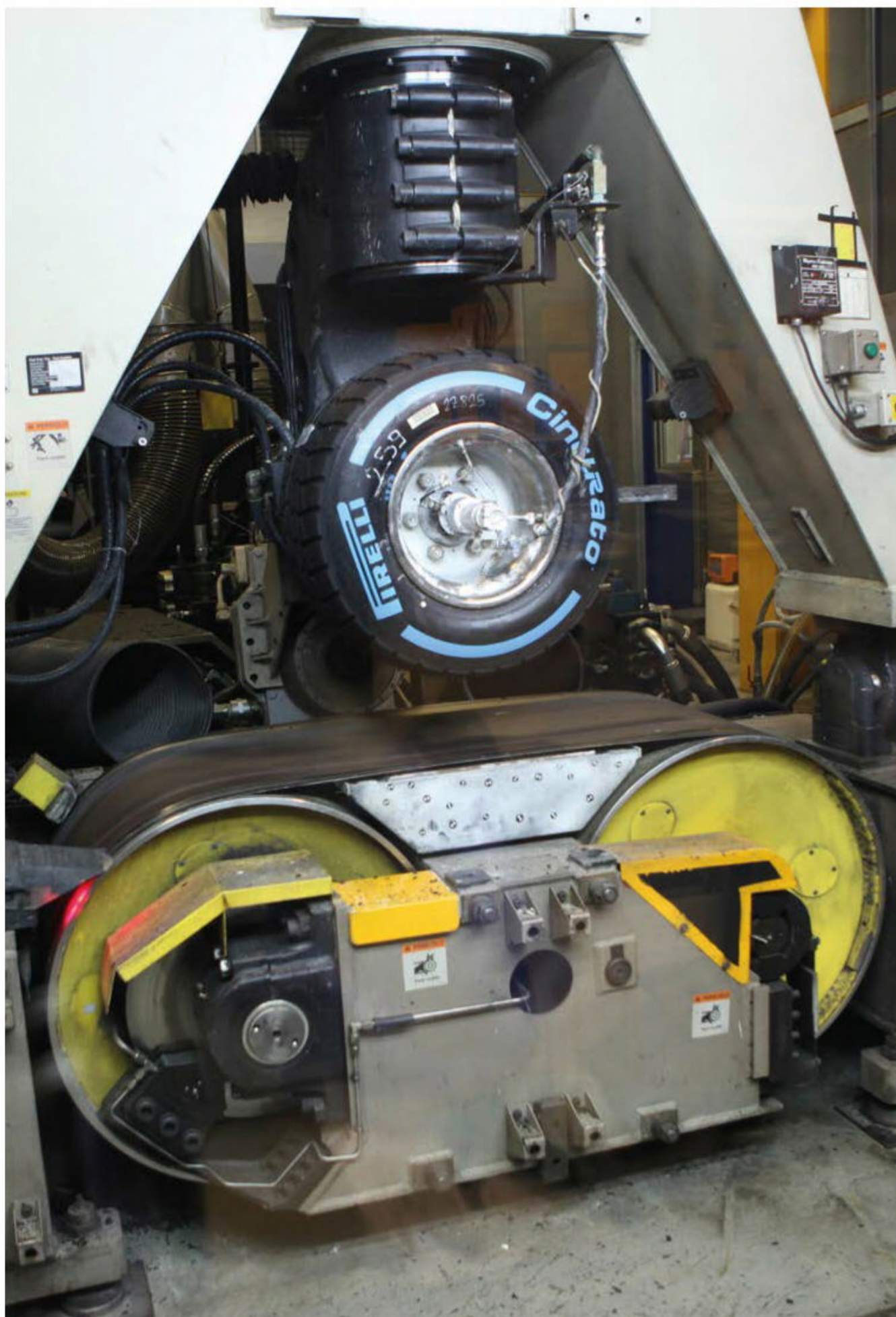
Fig 2: Example of an F&M (force and moment) indoor tyre testing machine, where the simulated 'road' moves beneath the tyre
