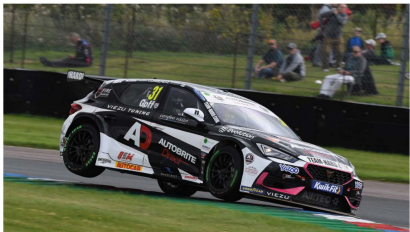
Some assumptions are perfectly reasonable. For an engine-over-drive-wheels car, for example, we know that the outside wheel at the non-driven end will take all, or nearly all, the load in a corner
