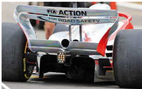
The 2022 rear wing enables flow to roll off the top of the wing tips and narrows the expansion of dirty air from the back of the car
