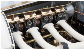
Four valves per cylinder was a technological development borrowed from Peugeot, but Daimler engineers chose to use just one cam
