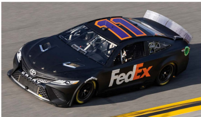
The lower roof line and swooping rear window suits all three of the main manufacturer models, as does the much shorter rear deck section. The result is all three retain a strong brand identity
