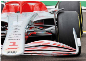
The 2022 regulations abolish the element-less 250mm section across the centre of the front wing in favour of wing elements that connect directly to the nose
