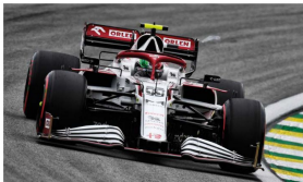
Rear wing tip vortices, seen here being shed from the left tip of the Alfa Romeo, have a huge influence on the size and shape of the dirty air shed from the 2021 cars. These won't be a factor in 2022, and the hope is that the racing will be correspondingly closer
