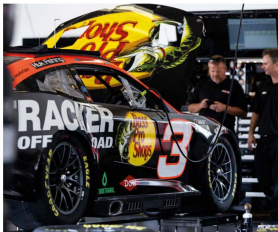
Early on track testing showed unacceptable heat ingress into the cockpits, so a raft of change were made to improve driver cooling
