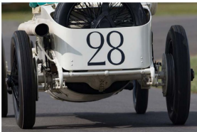
Using rear brakes only may seem foolhardy, but it helped win the race as the all-wheel braking Peugeot wore its tyres much faster
