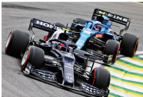
The 2021 cars are particularly sensitive to dirty air and drivers comment on how difficult they are to manage in following scenarios
