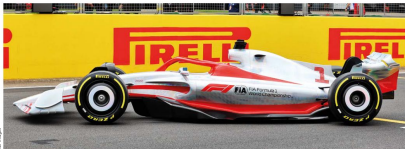
The 2022 car's downforce will predominantly come from a carved underfloor with tunnels that take advantage of Bernoulli's principle to interact with the track surface
