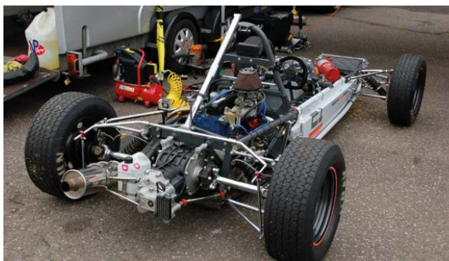
A typically pristine Historic Formula Ford. Note the very basic spaceframe, outboard suspension, large rear anti-roll bar and Hewland gearbox. The latter part is becoming harder to find these days, and therefore more expensive
