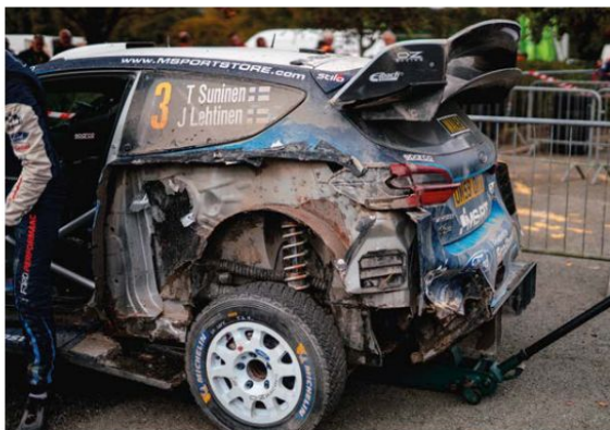
Rally cars are often damaged so, as well as being functional, aero devices have to be very robust, too
