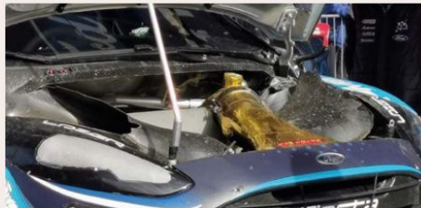
Pipes feed vented air out through adjustable bonnet vents in the M-Sport Fiesta...
