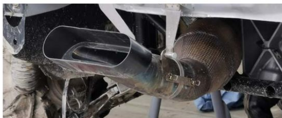
To ensure diffusers still worked at low speed, fuel was injected off throttle to keep the turbo spinning
