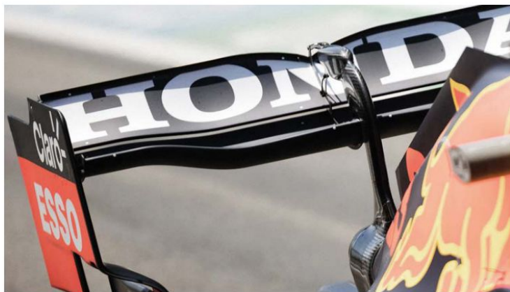
The wing's single pillar design was initially a weight saving exercise, but revisions made to appease the FIA ended up adding weight
