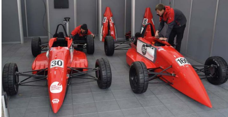
These days, FF1600s feature wide-track suspension and a pointy-nosed aero approach that's very much focused on low drag. Pictured is a Ray GR19 (left) and Ray GR14
