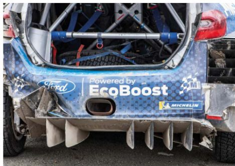
Post 2017, bounding boxes for areas such as the rear diffuser were used to their max
