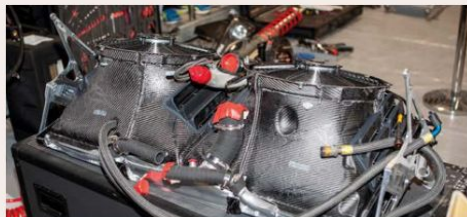
...while in the Toyota, two fans draw air into the engine bay through the intercooler
