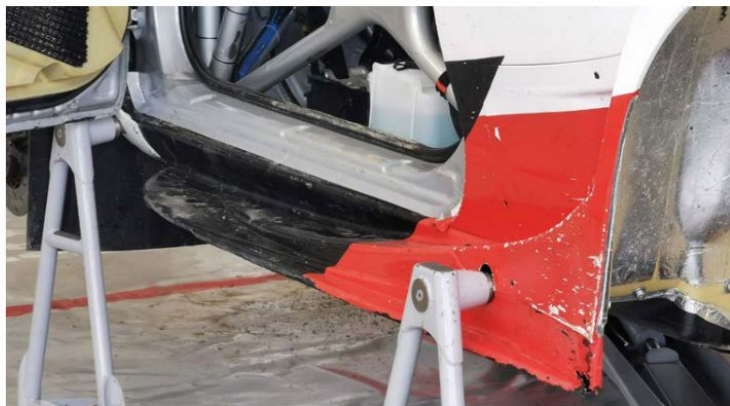
The sills on the Toyota WRC saw significant detail improvements over the years, many aimed at strengthening them against impact
