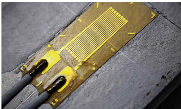
Strain gauge mounted to a measured component. In terms of a racecar, this is usually an aerodynamic or suspension component
