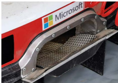
Borrowing from circuit racing practice, the Yaris WRC had an exhaust blown diffuser
