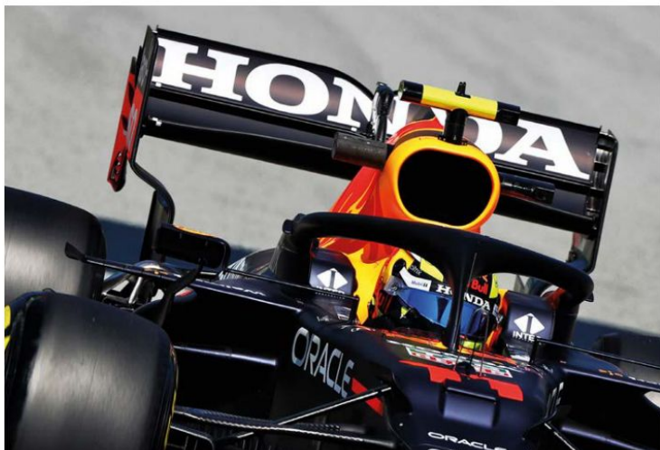
The controversial rear wing introduced at the Spanish Grand Prix, which appeared to change shape under high downforce load
