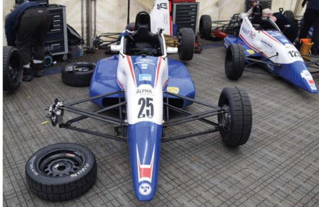
Australian constructor, Spectrum, has had success at home, in the UK with Kevin Mills Racing and in North America. Note the Avon ACB10 treaded tyres, which are used for both dry and wet running
