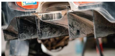
Exhaust-blown diffusers proved very successful, but are now outlawed by regulation
