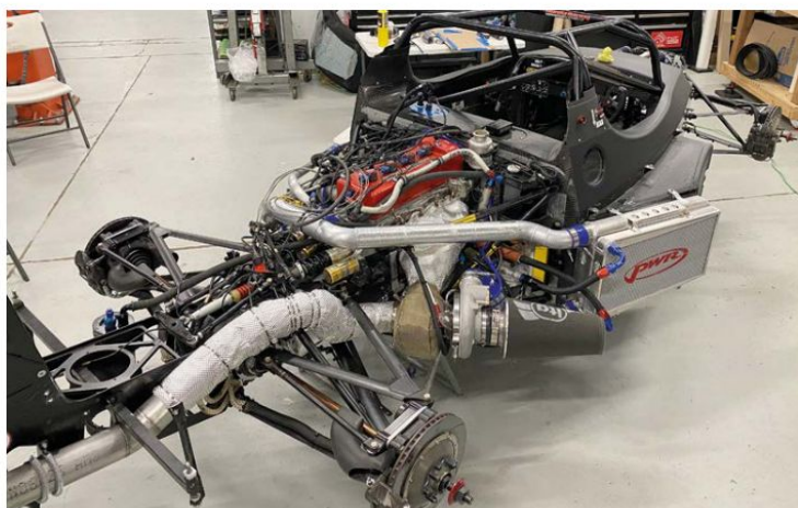
After the 2019 attempt, the Honda K20a engine was further developed by Mountune USA and fitted with a custom Borg Warner turbo
