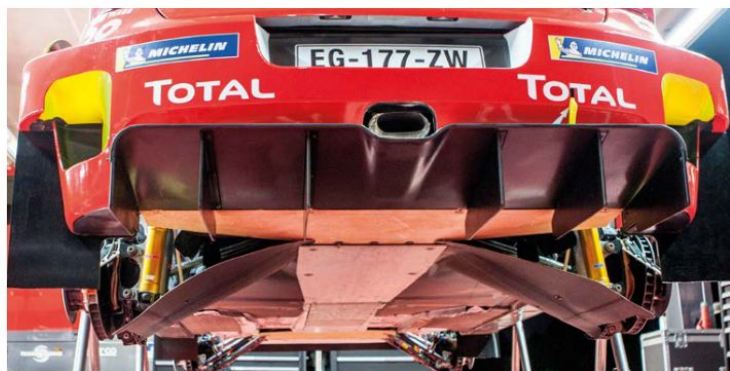
Adapting circuit race technology to a motorsport category that takes place on all manner of terrain, and where the competing cars' proximity to it varies wildly, added greatly to the technical challenge of engineering an aero device like the Citroën WRC's underbody
