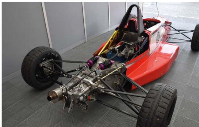
Modern Ray from the rear, showing where the steel spaceframe meets the lightweight aluminium bellhousing that carries the rear suspension and gearbox
