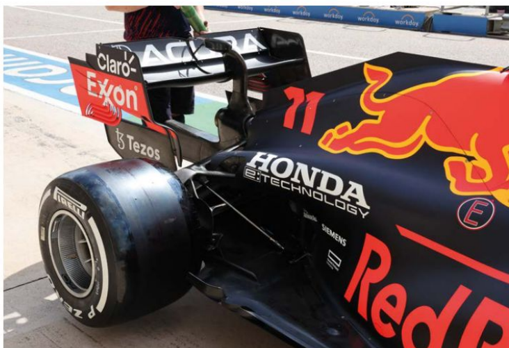
Rear diffuser and brake duct development was key throughout the year, often seeing design iterations on a race-by-race basis
