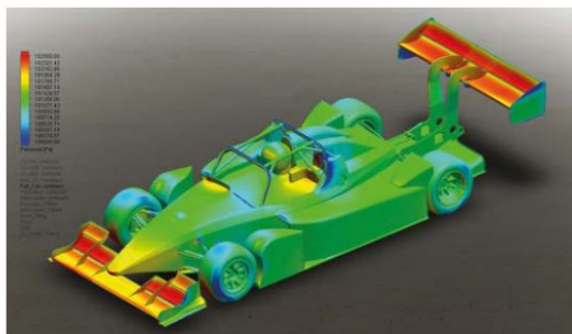
Figure 8: Pressure plots with conventional intercooler siting in the sidepods
