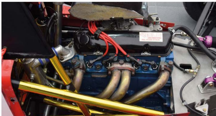
The faithful 1600cc Kent crossflow engine has been powering Formula Fords for over 50 years. New blocks are now cast in the US
