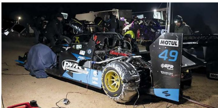
Car's carbon rear bodywork has been cut away to make space for extensive intercooler and turbo plumbing
