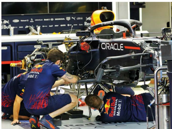
The reduced dimensions and cooling needs of the RA621 PU allowed even tighter packaging under the bodywork and engine cover
