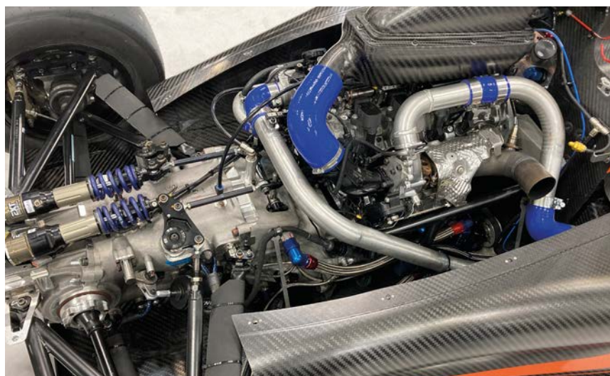
An all-new, and significantly lighter, SADEV gearbox has been designed specifically for the car, with the gear clusters sited ahead of the rear axle centreline to further improve driver safety in the case of a nose-to-tail accident
