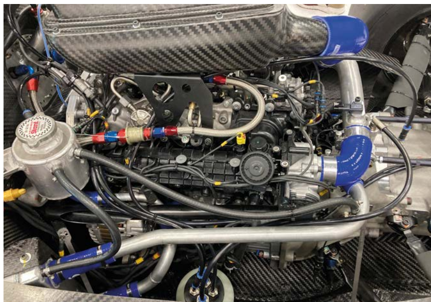
1.3-litre, four-cylinder, turbocharged engine has been prepared by ORECA and produces between 160 and 180bhp, but the chassis has been built to take anything up to a 300bhp power unit for use in different global formulae
