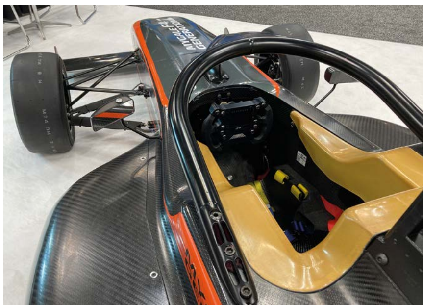
Three seat size options are offered, and a space between the seat and monocoque improves side-impact protection
