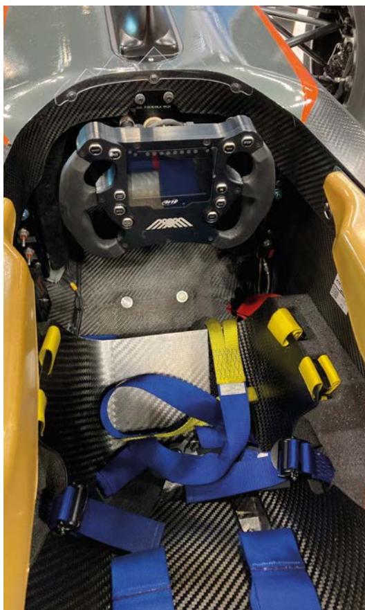
By regulation, the pedals and the drivers' feet are now contained within a longer monocoque with an anti-intrusion panel at the front
