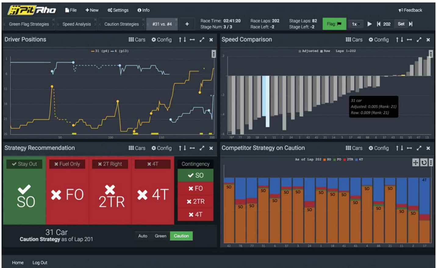
Machine learning can be used in many different ways in racecar engineering. This example data screen shows speed comparisons, suggested strategies and predicted competitor strategy
