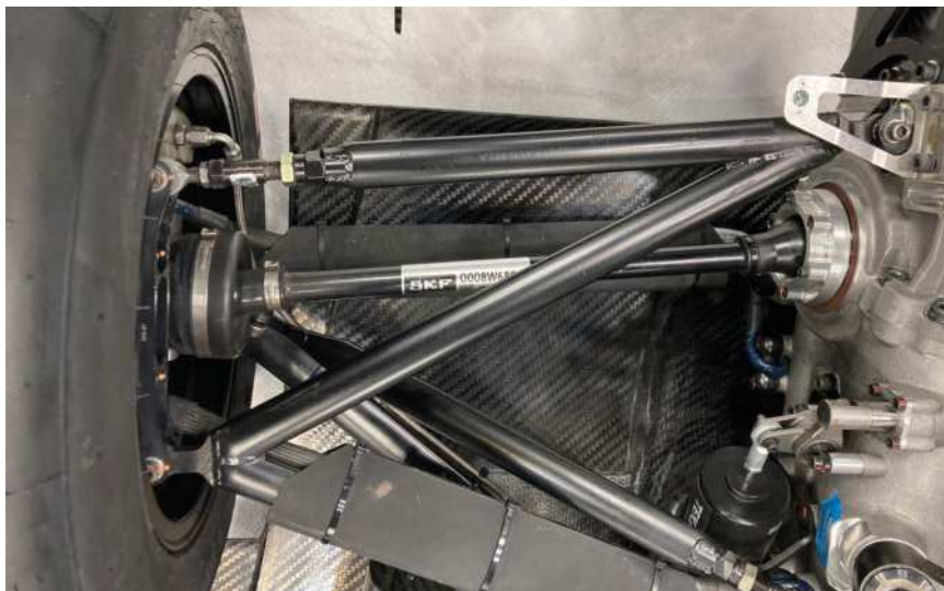
The car's double wishbone rear suspension was re-designed to pass the new rear impact crash test
