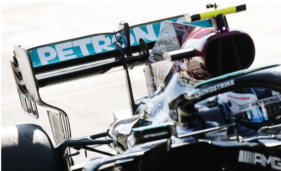
When it was suggested the front wing of the W12 was flexing more than it should, the FIA intervened. Datum point stickers and cameras monitor wing displacement during the investigation, but no further action was taken
