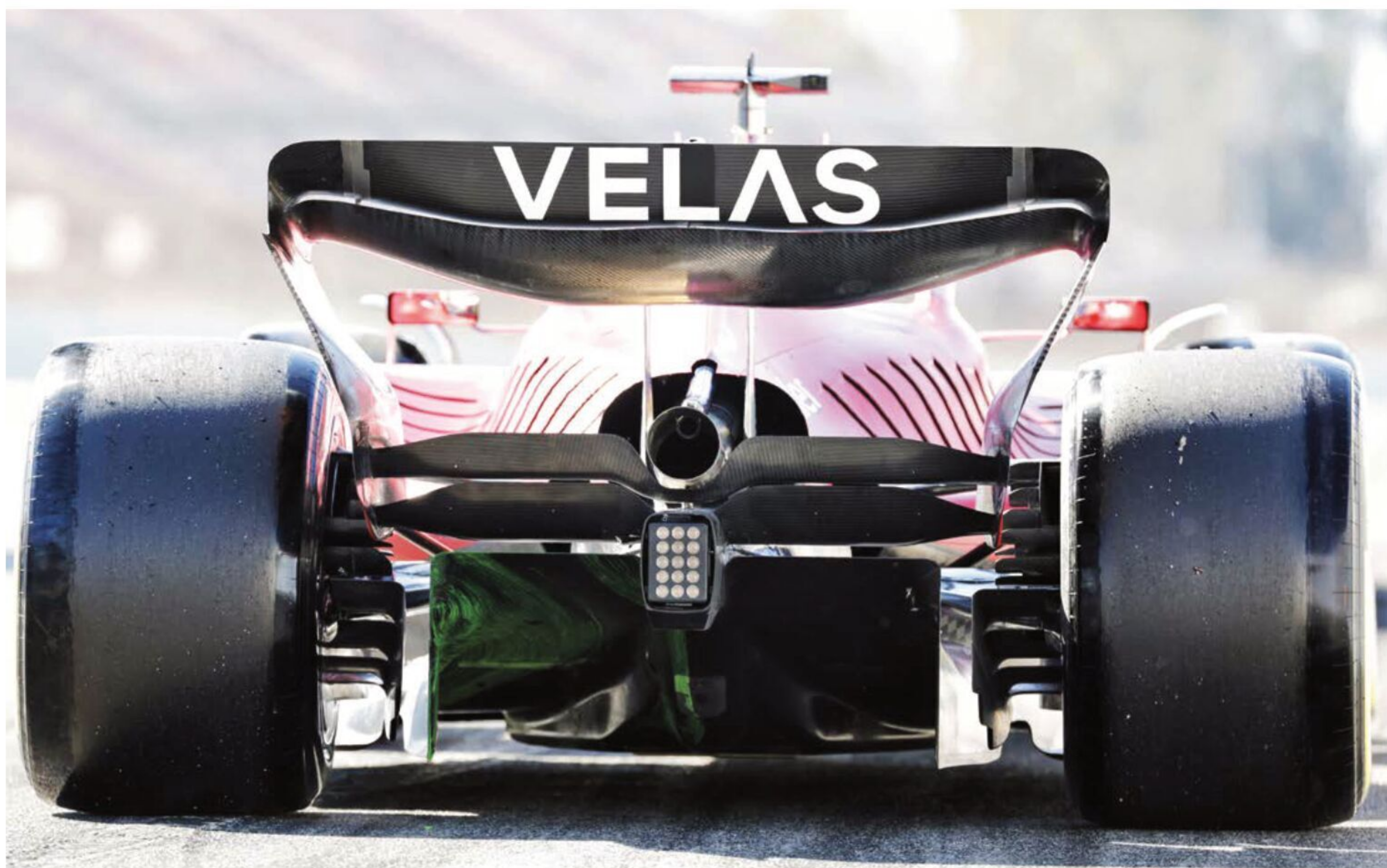
Flow vis in the tunnels under the Ferrari F1-75 evident as the team worked through its test programme. Diffuser geometry is tightly prescribed by the rule set, so there is little variation there
