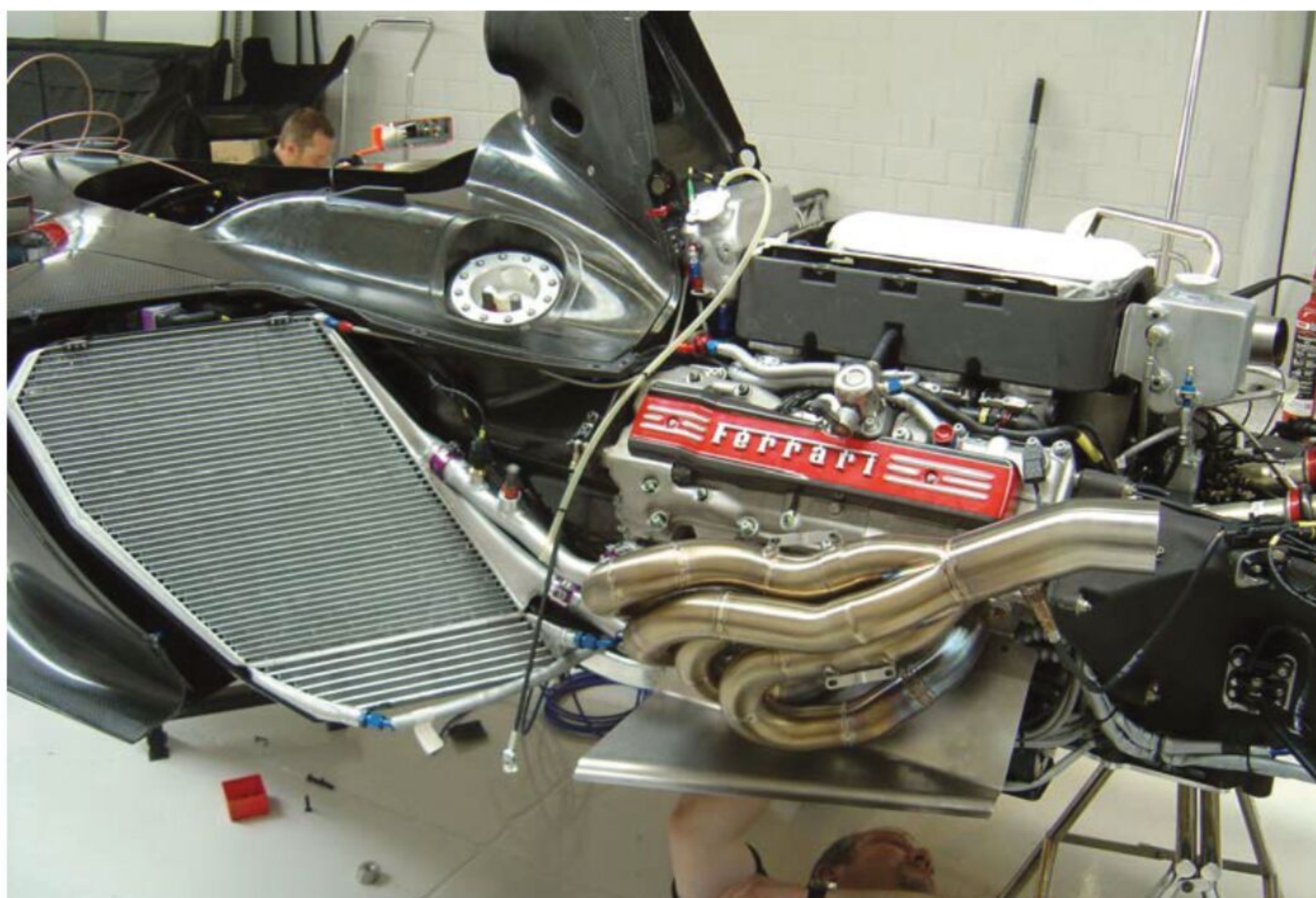
The engine was a 600bhp, roadgoing V8 from Ferrari’s F430 model. Its 160kg weight caused some problems with balance
