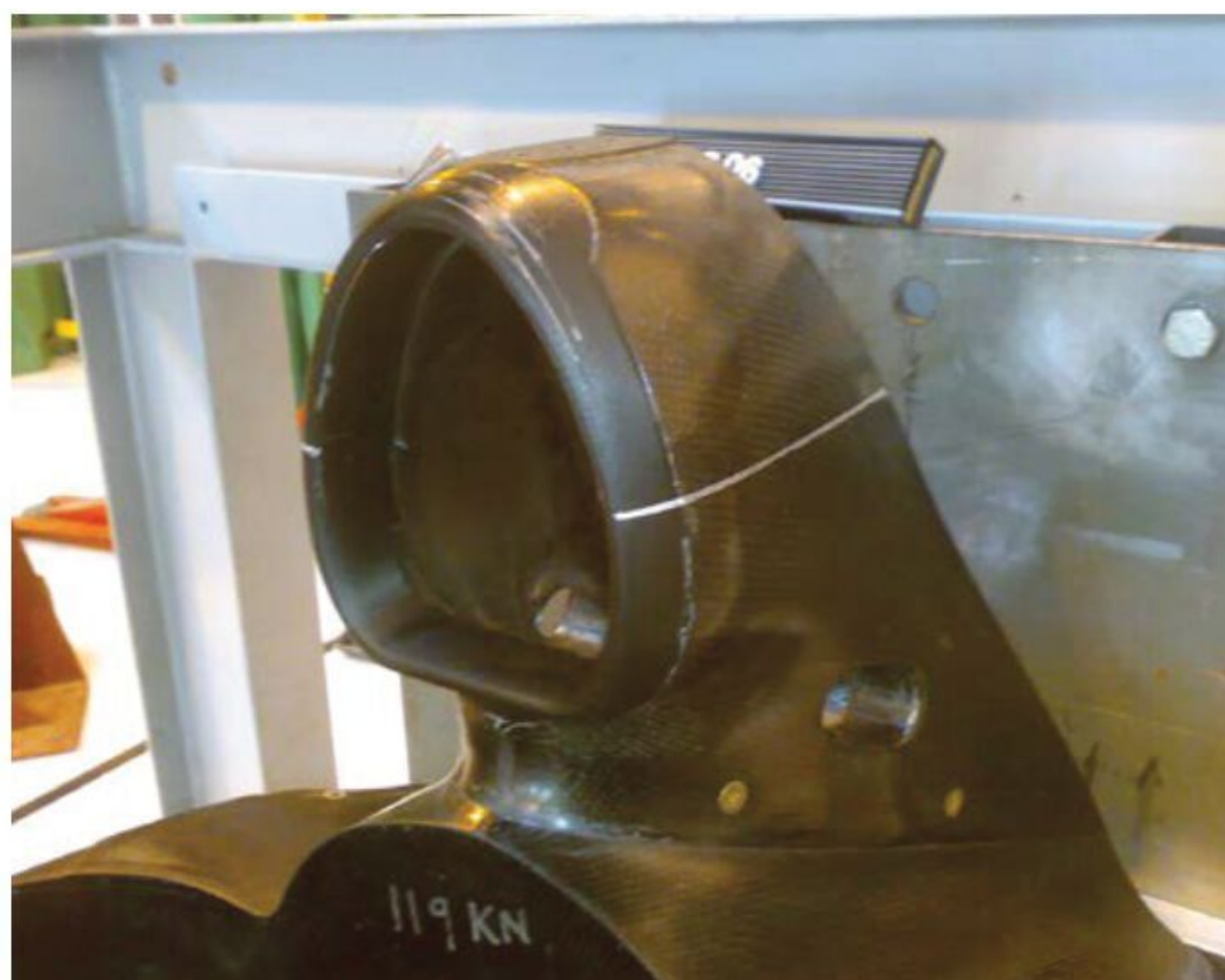
FEA was used to develop the car's FIA-standard, Formula 1-spec composite roll hoop, which was made from a billet aluminium mandrel clad with a carbon fibre exterior
