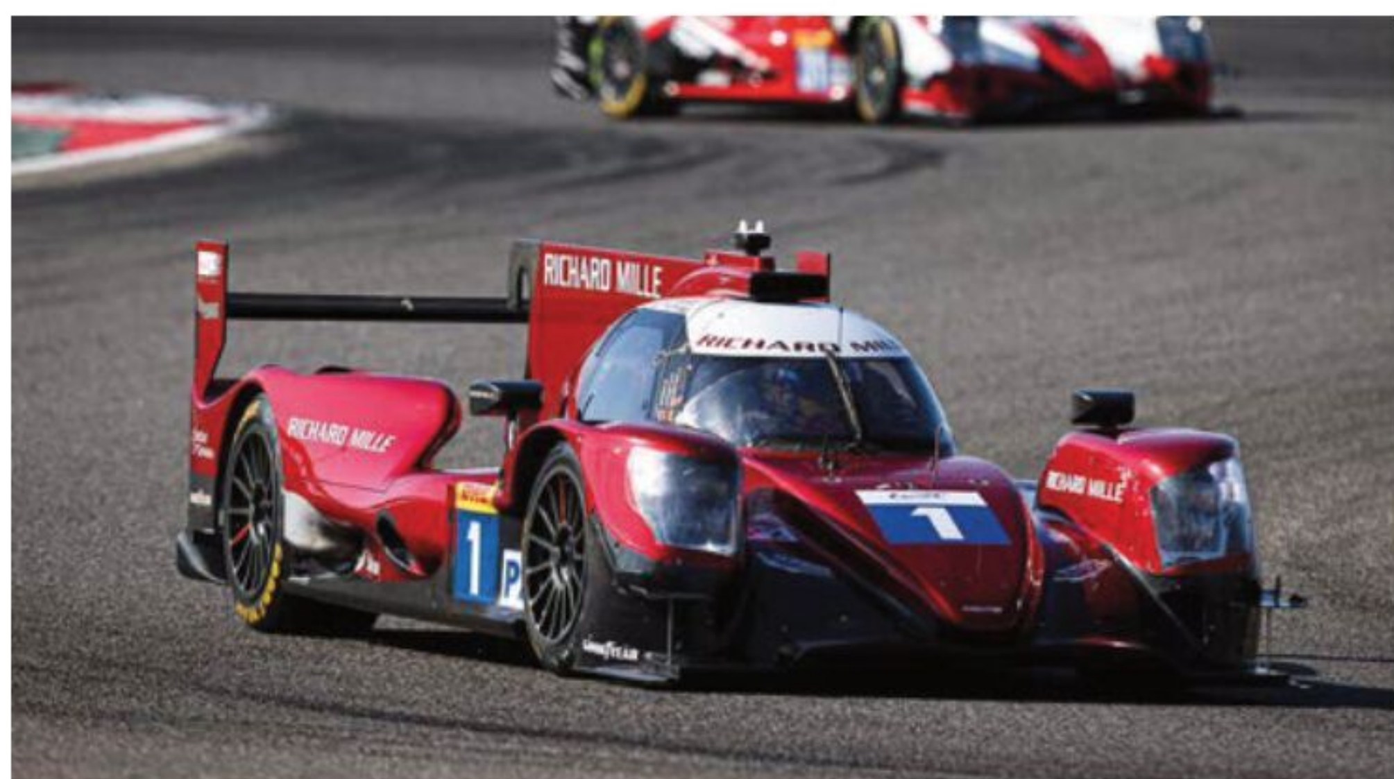
Low-speed damping – generally occurring at speeds less than 0.1m/s – is associated with a ‘crisp’ turn-in response, as this PKM-equipped Oreca 07 Le Mans Prototype shows
