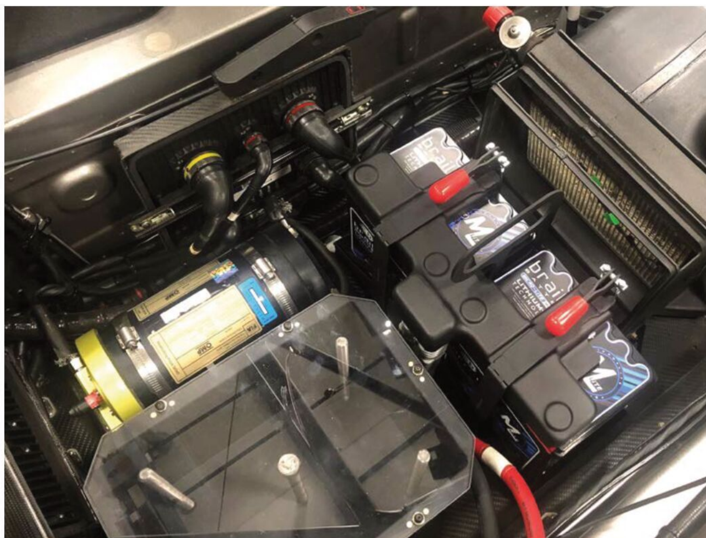
Shifting weight meant moving the air conditioning unit, fire bottle, battery box, plus all their wiring, and other electronic items
