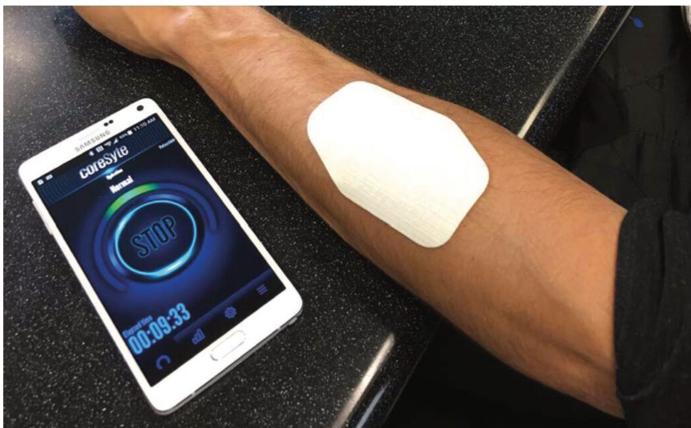
The patch takes a sweat sample every three minutes, giving a string of data points throughout a race that can then be analysed
