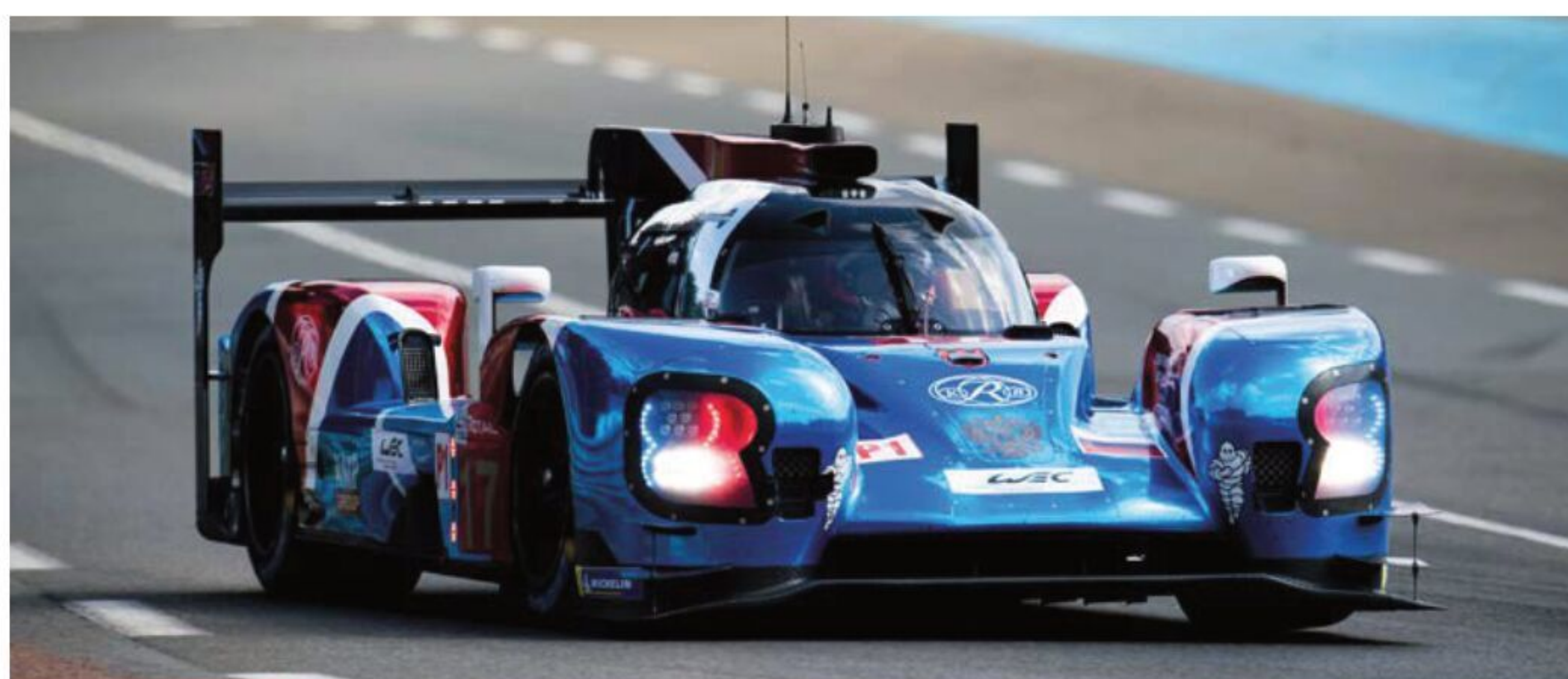
In high aero categories, such as the old LMP1 era of the WEC pictured here, bump stops provide a method of maintaining a car's minimum ride height when travelling at high speed, while at the same time allowing the use of soft springs for low-speed grip
