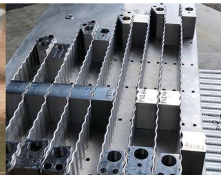
Battery packs prefer to be kept between 20 and 50degC, so the associated cooling package is critical. In some applications, liquid cooling channels, such as these produced by Goodfabs, will be wrapped around the pack
