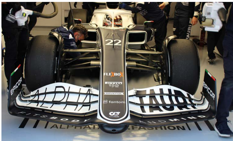
The AT03's front wing has all its elements attached to the nose, unlike some of its rivals who have opted for a separated lower section to condition the flow to the floor
