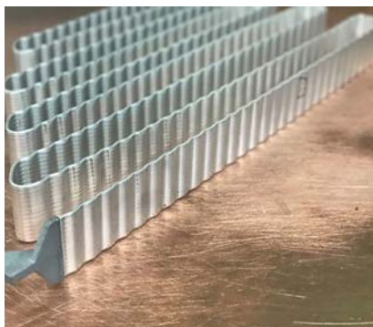
Battery packs prefer to be kept between 20 and 50degC, so the associated cooling package is critical. In some applications, liquid cooling channels, such as these produced by Goodfabs, will be wrapped around the pack
