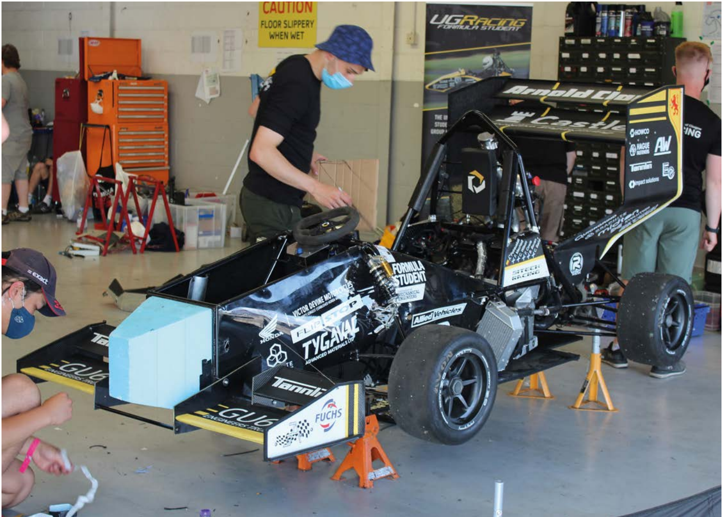
In a relatively low speed competition like Formula Student where inertia is high, response is the most critical factor, so wheelbase and track are kept deliberately small for maximum agility
