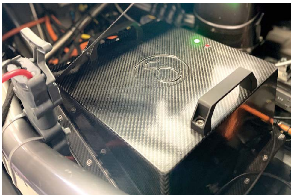
Cell construction and internal chemistry determines the balance of power and energy densities. BTCC battery pack shown
