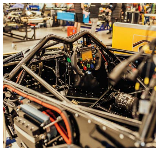
Radical has kept its faith in spaceframe chassis since its inception, arguing that they make sense from both a cost and safety perspective
