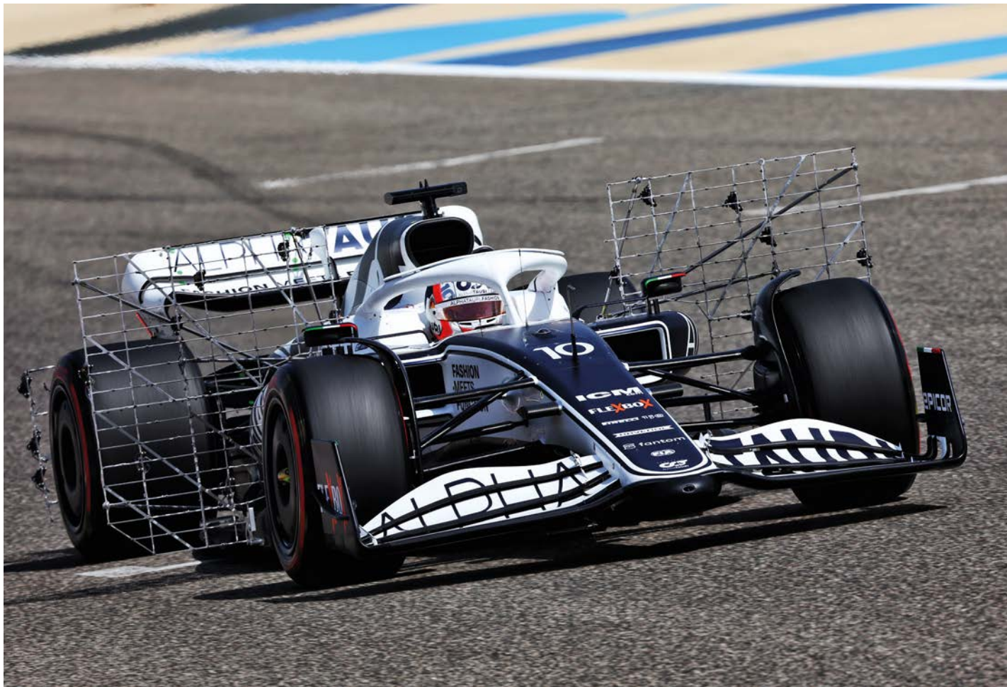
The pitot arrays fitted to the sidepods collect data on the front tyre wake in order to correlate real-world turbulence with the simulated models developed by the engineering team
