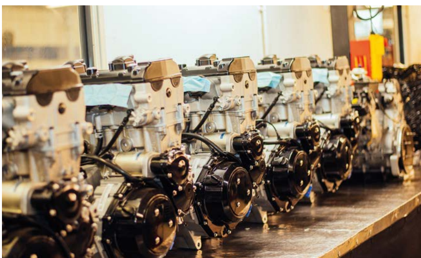
The RPE Suzuki Hayabusa, in 1340cc and 1500cc form, can be found in both the entry-level SR1 and the evergreen SR3
