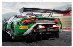
Development of the floor and diffuser is allowed, so the new car features a heavily sculoted underside and more dramatic diffuser
