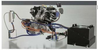
The 350+bhp internal combustion engine operates in parallel with a Cosworth Electronics-developed 40kW (54bhp) hybrid system and control unit
