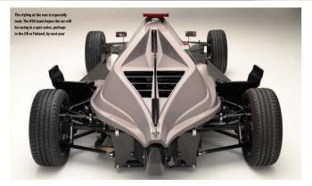
Meanwhile, the suspension is as simple as possible, harking back to Formula Fords of old, with a double-wishbone layout and a single-adjustment, oil-filled collover damper from UK supplier Protech Shocks, fitted outboard. Sensibly, the wishbones are nonhanded to reduce sparse cost.
