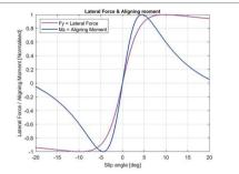
Graph showing the relationship between slip angle and aligning moment (Mz)
