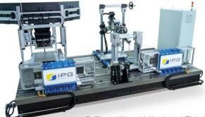
DiL and HiL are proving valuable instruments in developing steering systems using EPAS and steer-by-wire
