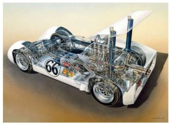
David Kimble captured the features of the Chaparral 2E beautifully in this full-car cutaway, including the aerofoil-section tubes that carried the wings with the hydraulic actuators hidden within
