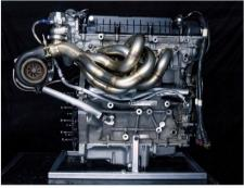
The 2.0-litre, turbocharged, road car-based engine formula remains for the BTCC going into the new era, with subtle modifications made, primarily to the camshafts and valvetrain, to improve performance and durability in a racing application
