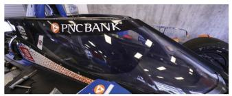
The RBAT designed Aeroscreen was the second iteration of head protection offered by IndyCar but the complete design helped to elongate the life of the original DW12 chassis
