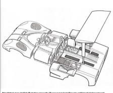
Brian Hatton's more simplistic illustration exposes the 2E's rear suspension trailing arms and forward-sloping water and oil radiators. It's slightly incorrect in that the instrument panel was actually further forward than shown
