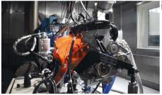
Reliability analysis of the new engine package included over 5000 miles of race running on M-Sport's transient dyno
