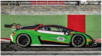
The new FIA technical regulations for GT3 stipulate the doors and roof be exactly the same as their production counterparts; the fin and roof-mounted air scoop are new concepts for the EV02
