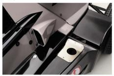
To help fit a silencer to keep noise levels within today's acceptable limits, the exhaust needed to go through some serious contortions along the chassis before emerging out of the top of the left-hand sidepod
