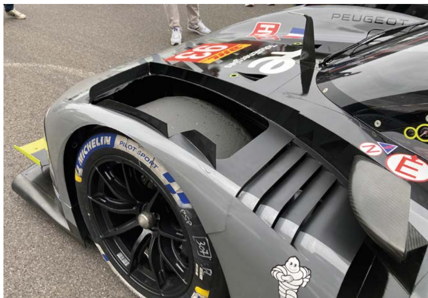
Fences around the wheelarches were added late in the process to try to meet stability criteria in the event of yaw
