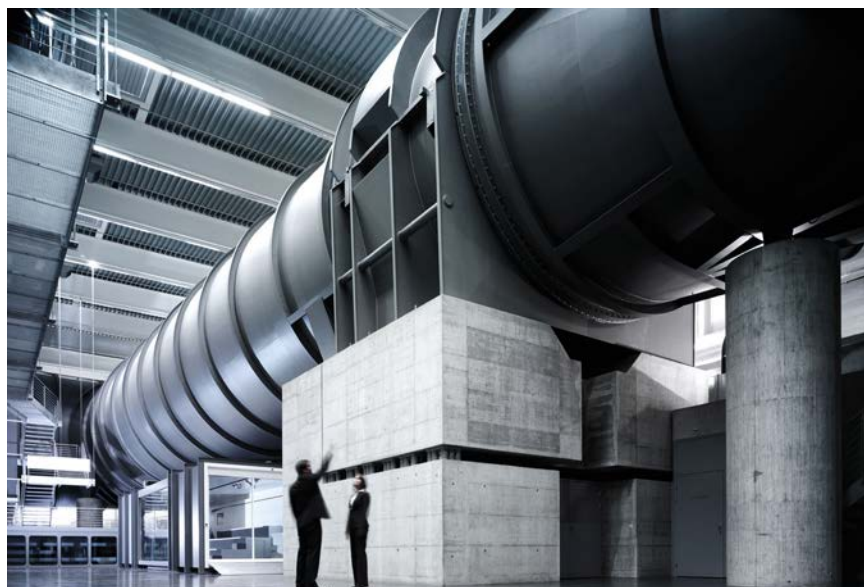
At over 141m in length and with a maximum tube diameter of 9.4m, the Sauber wind tunnel is a colossal structure, capable of accepting full-scale vehicles as well as the 60 per cent scale models required by current F1 regulations
