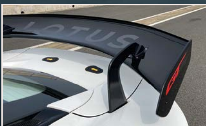
Car uses largely production body panels for cost of running purposes, but benefits from a new bonnet, floor / splitter, brake cooling ducts and a dynamic adjustable rear wing
