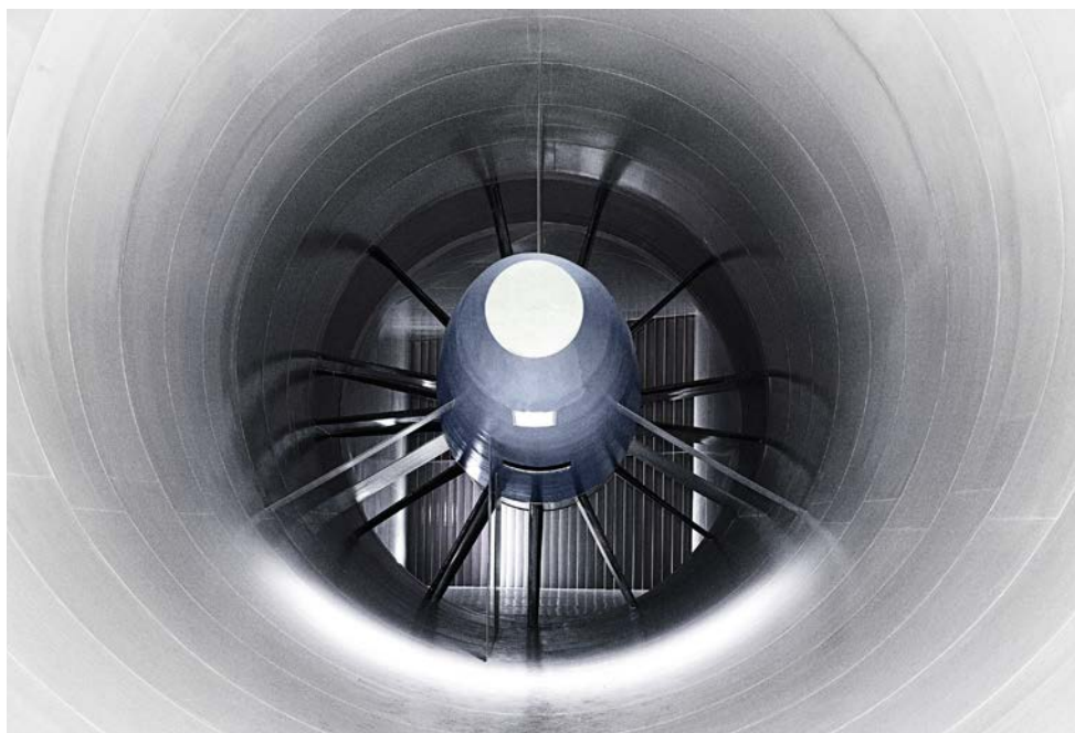
The wind tunnel's single-stage axial fan with carbon rotor blades can power the air speed up to 288km/h and uses 3000kW at full load
