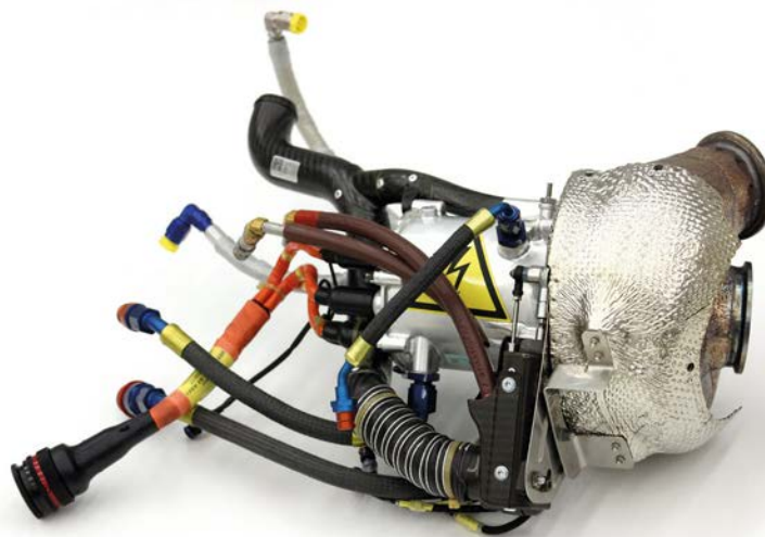
Porsche Motorsport's 35kW post wastegate-mounted H-ERS from the turbocharged, 2.1-litre, 9R9 V4 engine that powered its three time Le Mans-winning 919 LMP1 hybrid Prototype
