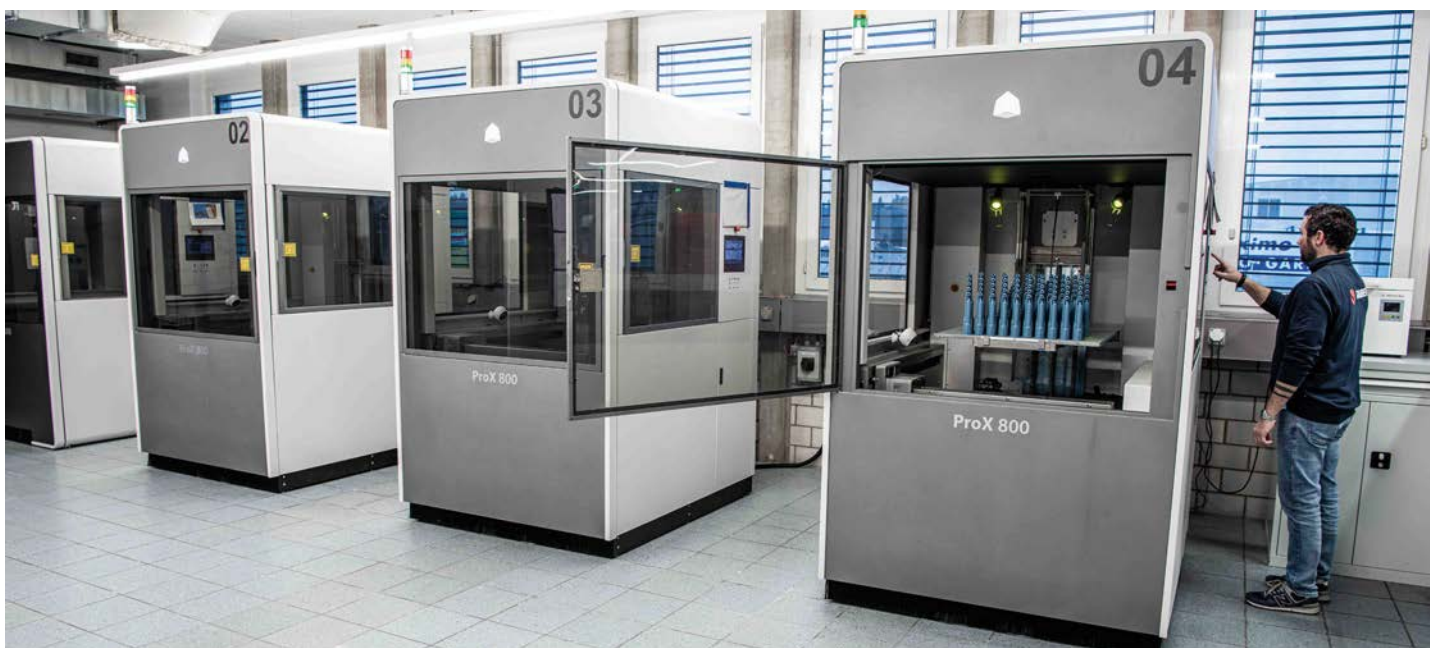
Sauber Technologies has invested heavily in AM technology in recent times. Shown here is its four stereolithography (SLA) polymer additive manufacturing machines
