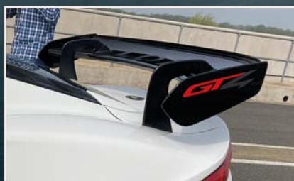
Car uses largely production body panels for cost of running purposes, but benefits from a new bonnet, floor / splitter, brake cooling ducts and a dynamic adjustable rear wing
