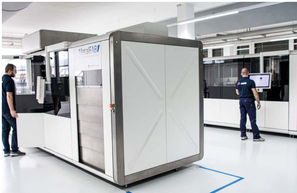
Additive Industries' modular and scalable MetalFAB1 system, designed for integrated and automated production with metal powder bed fusion technology using four lasers
