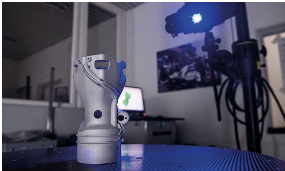
After an AM part is manufactured and processed, it is laser scanned and compared to the original CAD file to ensure no discrepancies
