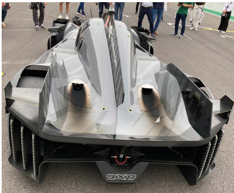
A rear Gurney flap was added to help increase drag, necessary to put the 9X8 in the required performance window before racing starts
