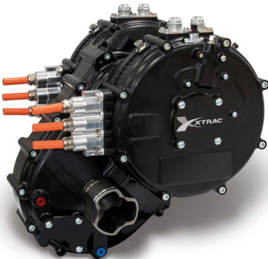
EV transmissions are a large and ever-growing part of the business. This is Xtrac's Integrated Lightweight Electric Vehicle gearbox
