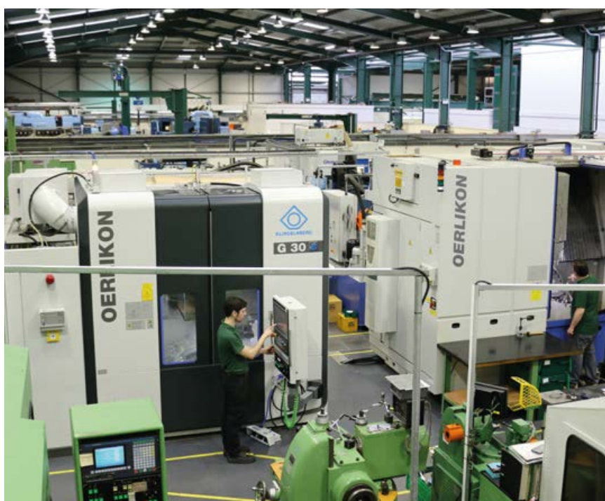
The factory floor is close to heavy industry, with millions invested into machinery, such as these bevel gear grinders
