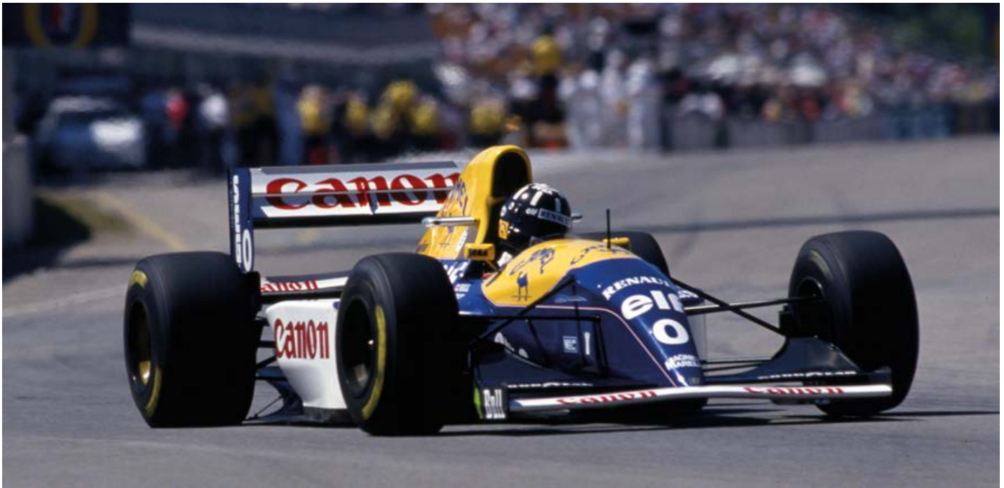
The Adrian Newey-designed Williams FW15C had semi-active suspension and dominated in 1993. It is perhaps no coincidence then that Red Bull appear to better understand the porpoising issue
