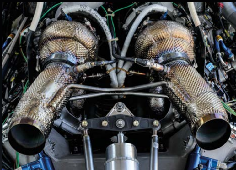
Engine is based on the company's 3.4-litre V8 from 2005 (shown), which was later bored out to 4.6-litres for the 918 road car. For LMDh, it uses twin turbos to achieve the prescribed power curves
