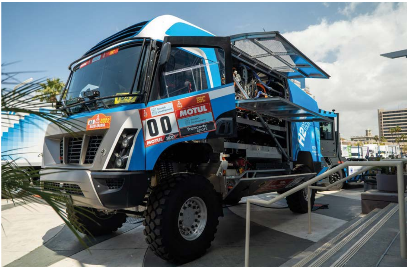
The first hydrogen-powered entry on the Dakar Rally was the H2 built by Gaussin of France. It featured a 380kW fuel cell, 82kWh battery and twin 300kW motors. It completed the 2022 event
