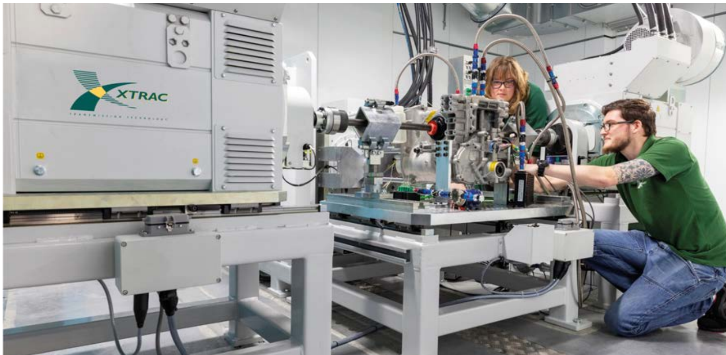
Xtrac employs a wide range of gearbox testing equipment, including recently acquired loaded EV rigs, which allow the company to run entire test and development processes in house
