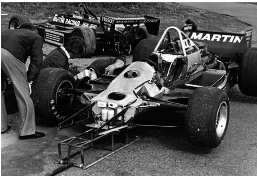
The monocoque used in the T80, T81 and T87, was the last time Team Lotus used aluminium construction
