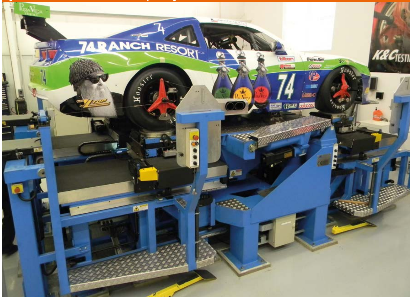
Fig 1: The Morse Measurements kinematics and compliance rig
