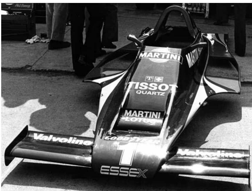
Front wings were added to the T80 to try to solve the porpoising issue but more work was needed to fix it properly
