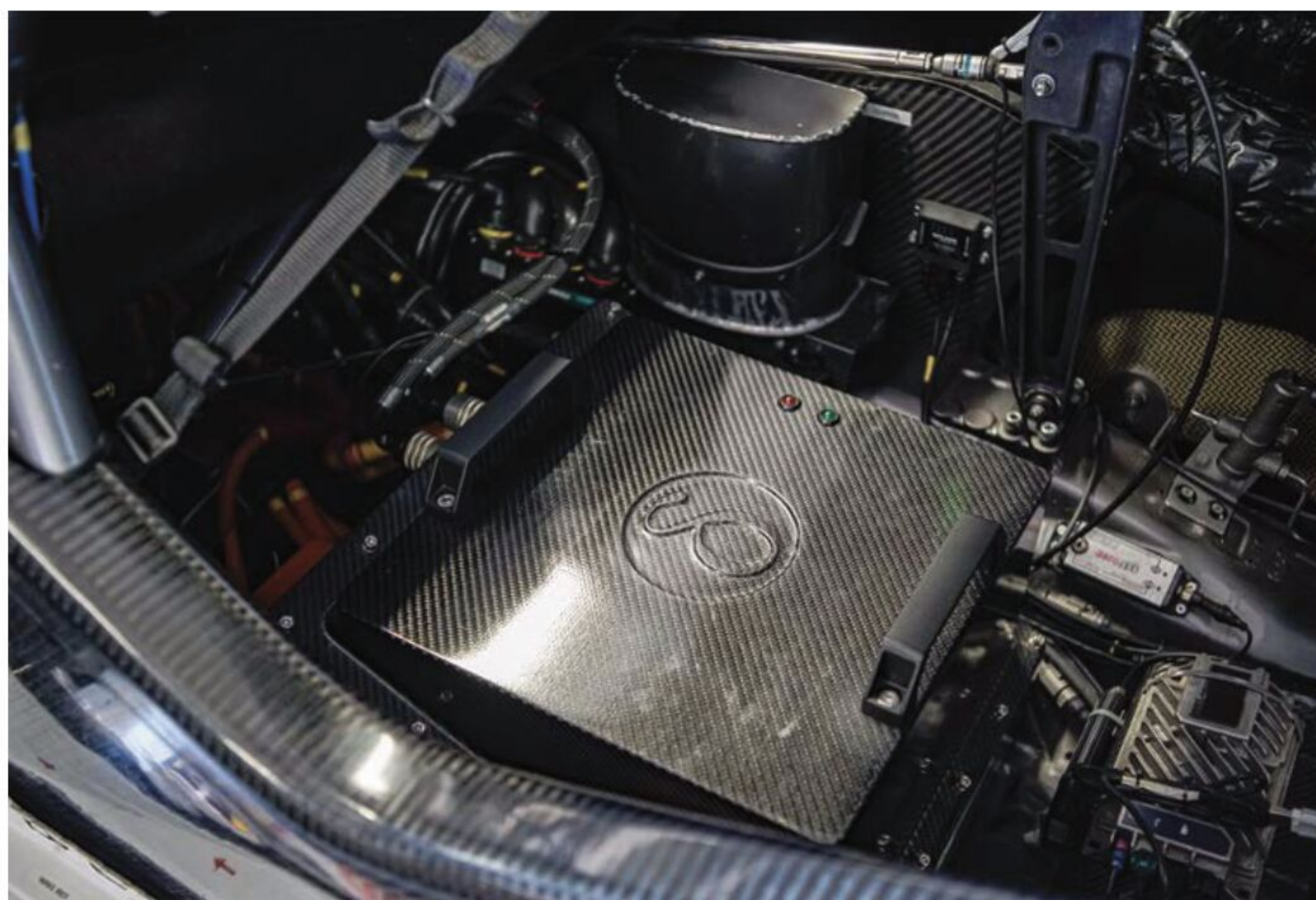
The 23kg Delta Cosworth battery pack is positioned alongside the driver, with all the regular safety protocols adhered to
