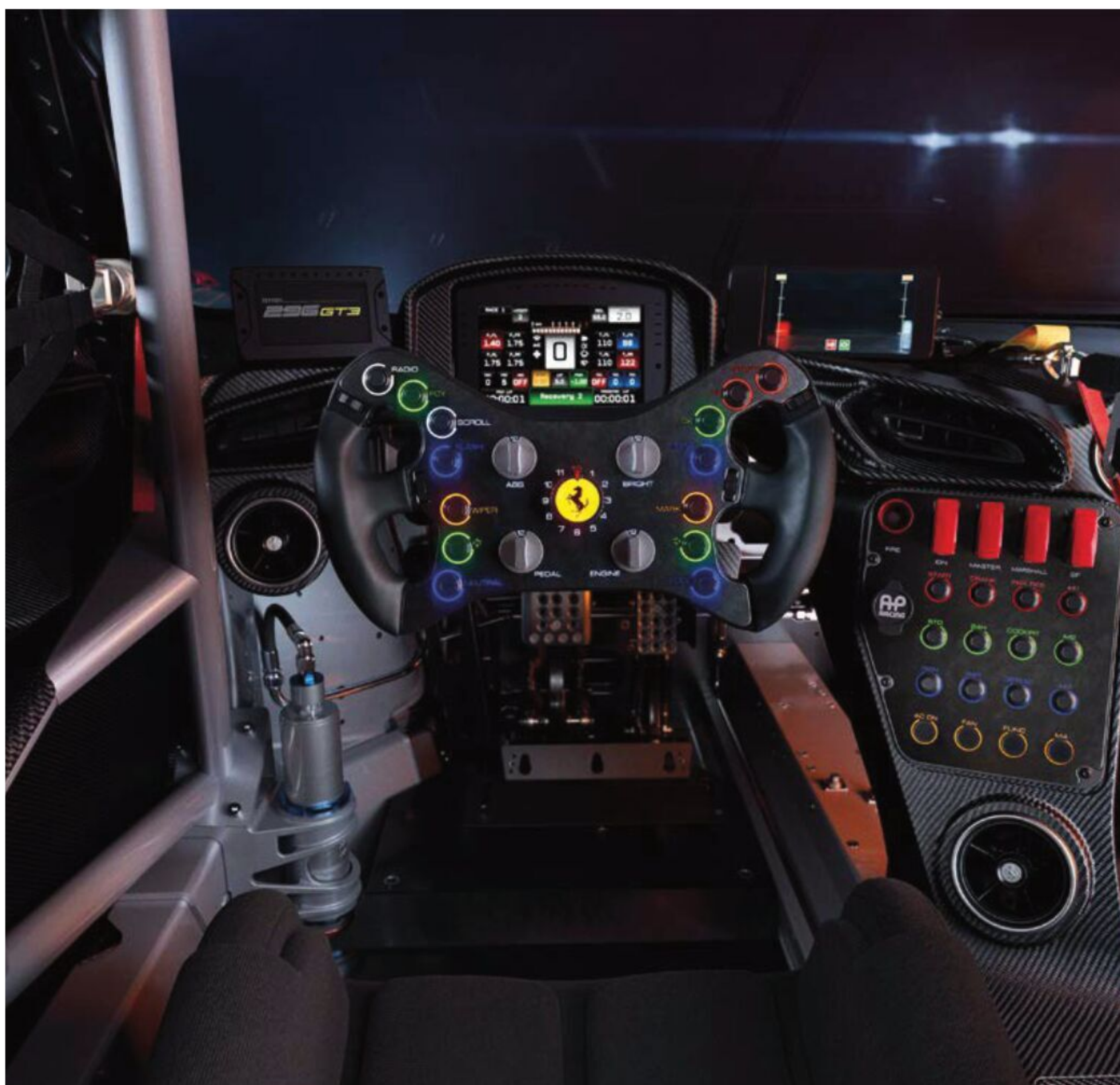
Multi-function programmable steering wheel also has a 12-layer shift control in the centre giving maximum functionality
