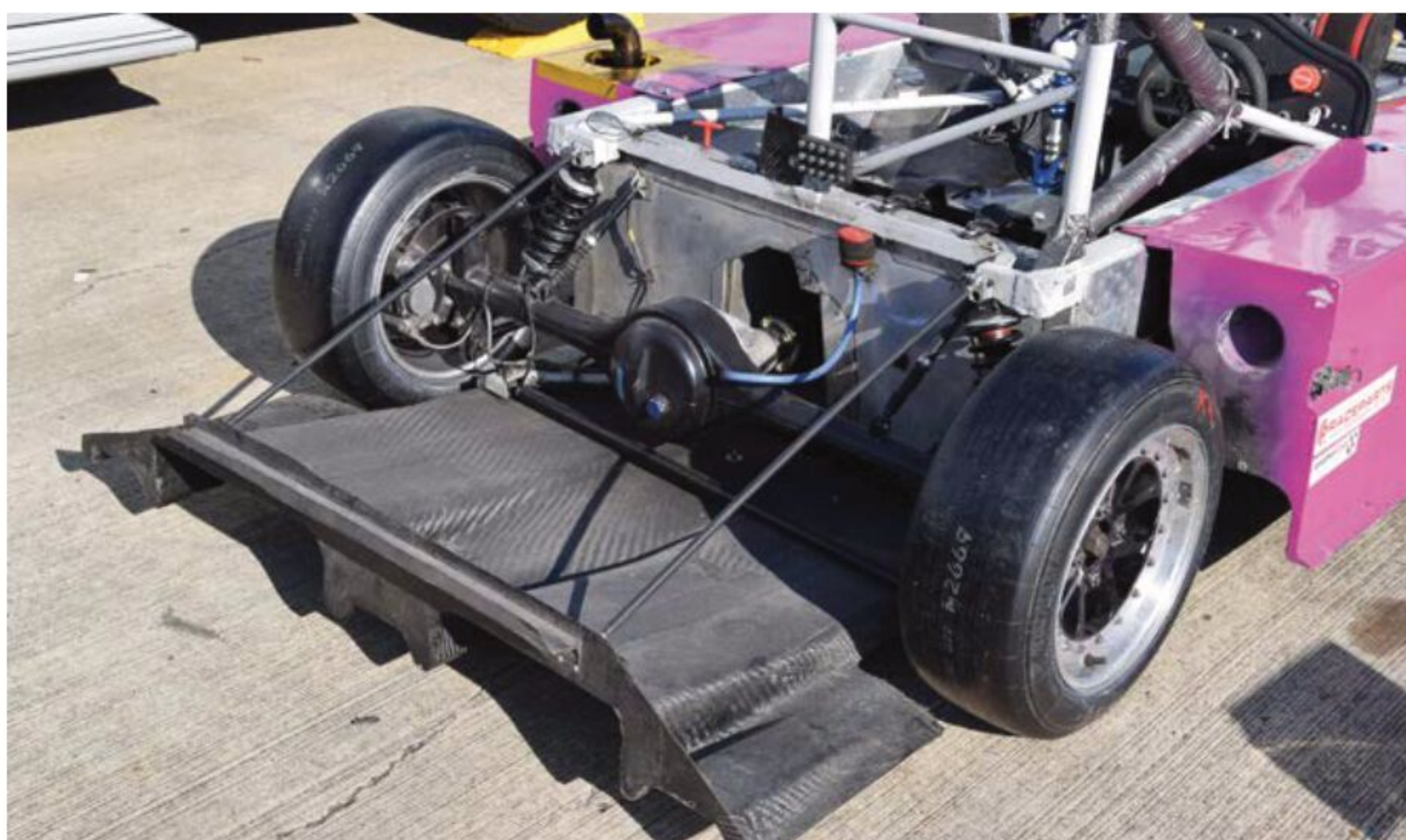
Where space age meets iron age: front-engined cars must run live axles and this example, in the highly developed CGR2 Evo, is from a British Morris Minor so is at least 50 years old, maybe considerably more
