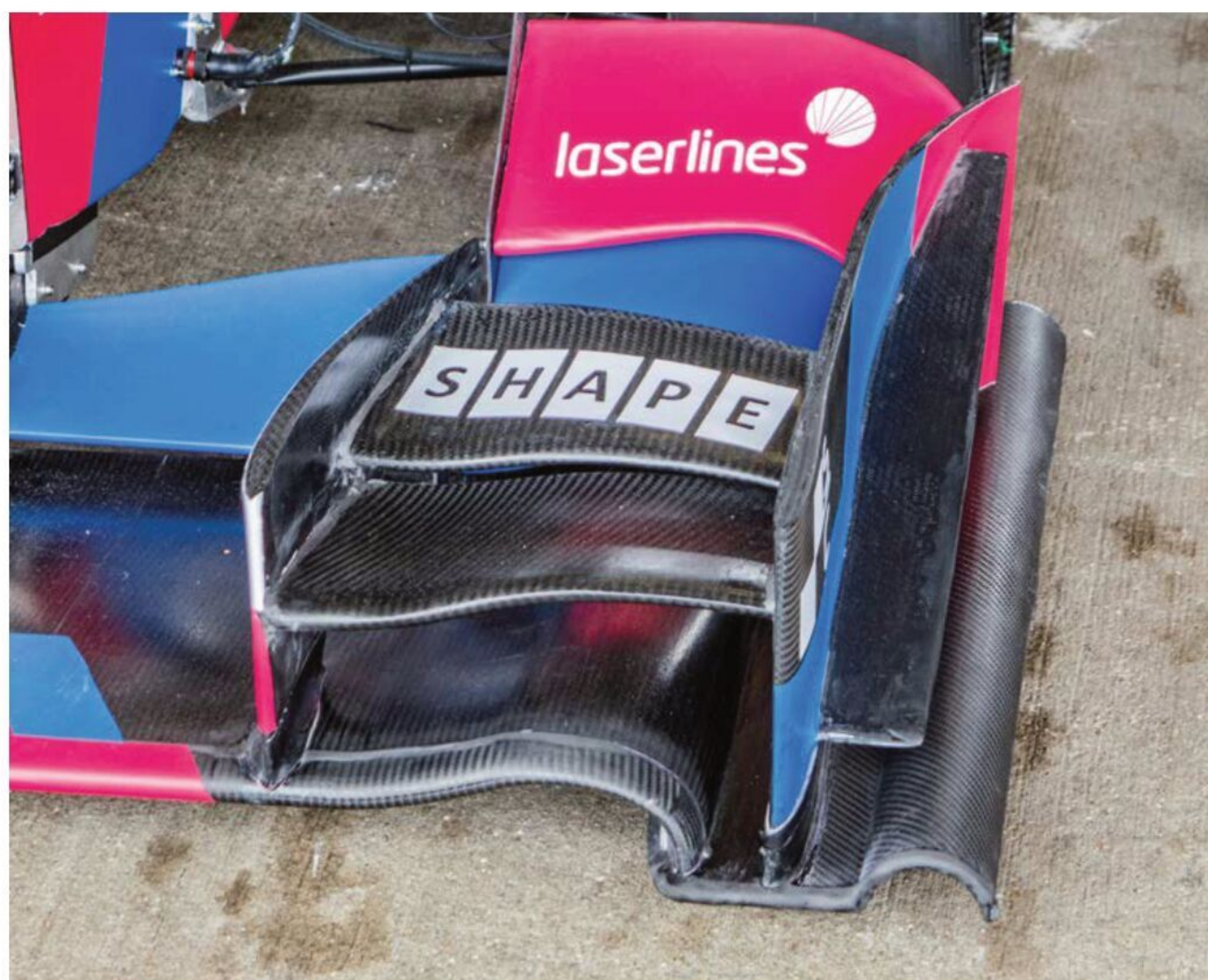
The advanced front wing design provides high front end loads as well as flow field conditioning for structures behind the front axle
