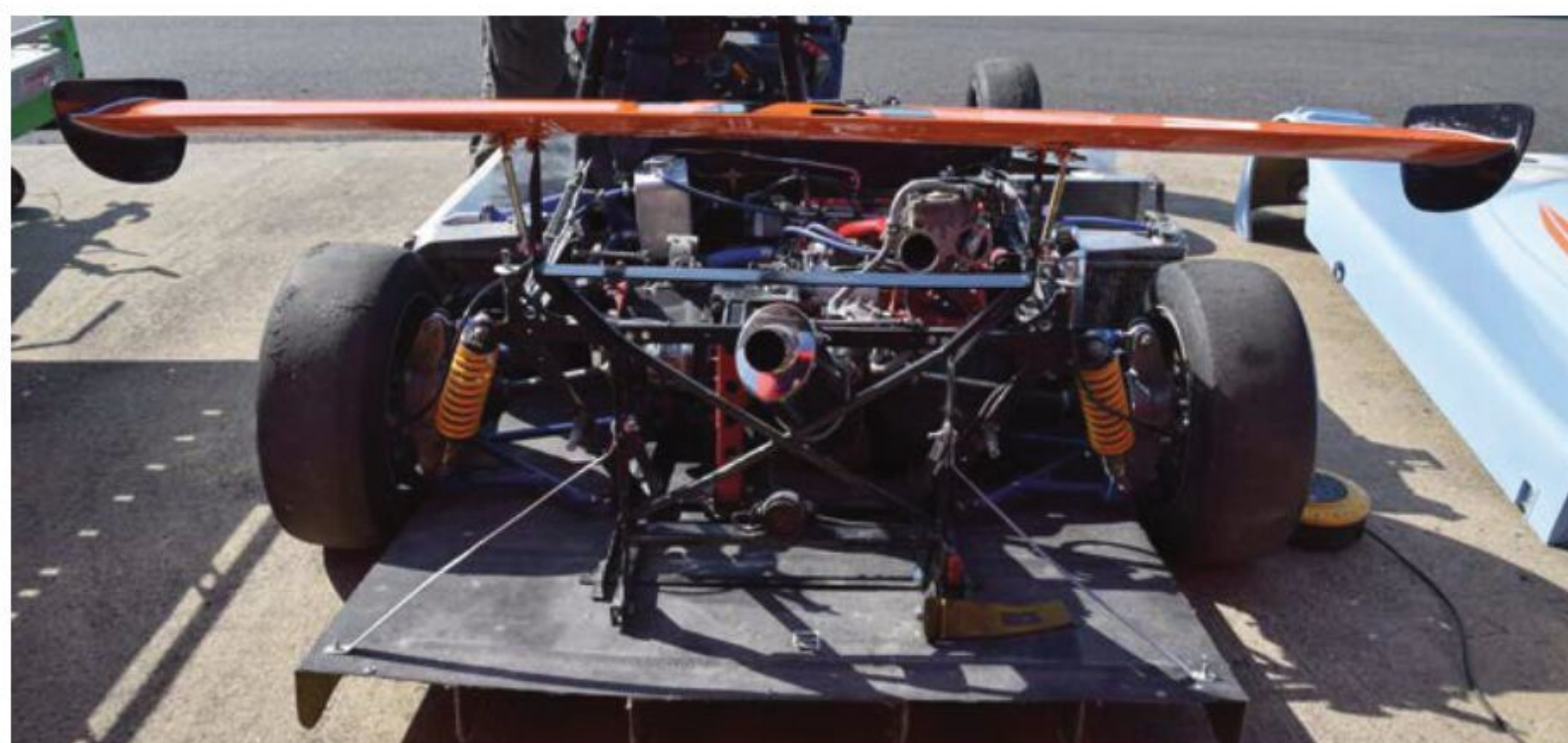
Despite the low-powered engine, aero development is rampant in the series, and most cars sport fairly large wings and diffusers – the latter is a recent addition to the SZT Mk1 pictured here
