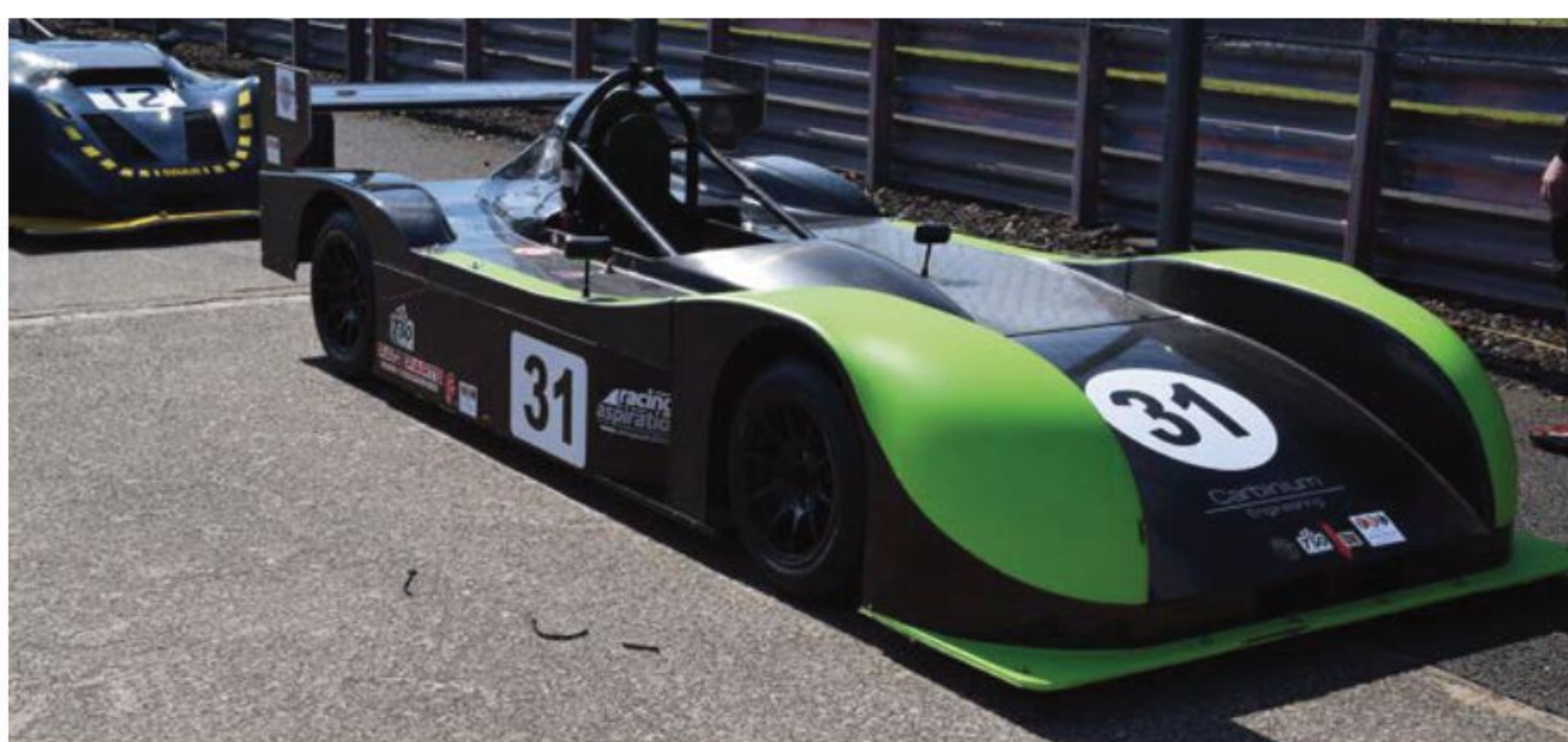
Olly Collett runs a lightweight carbon body on his Racekits Falcon, which has allowed him to improve the aerodynamics while not adding too much weight to the overall package
