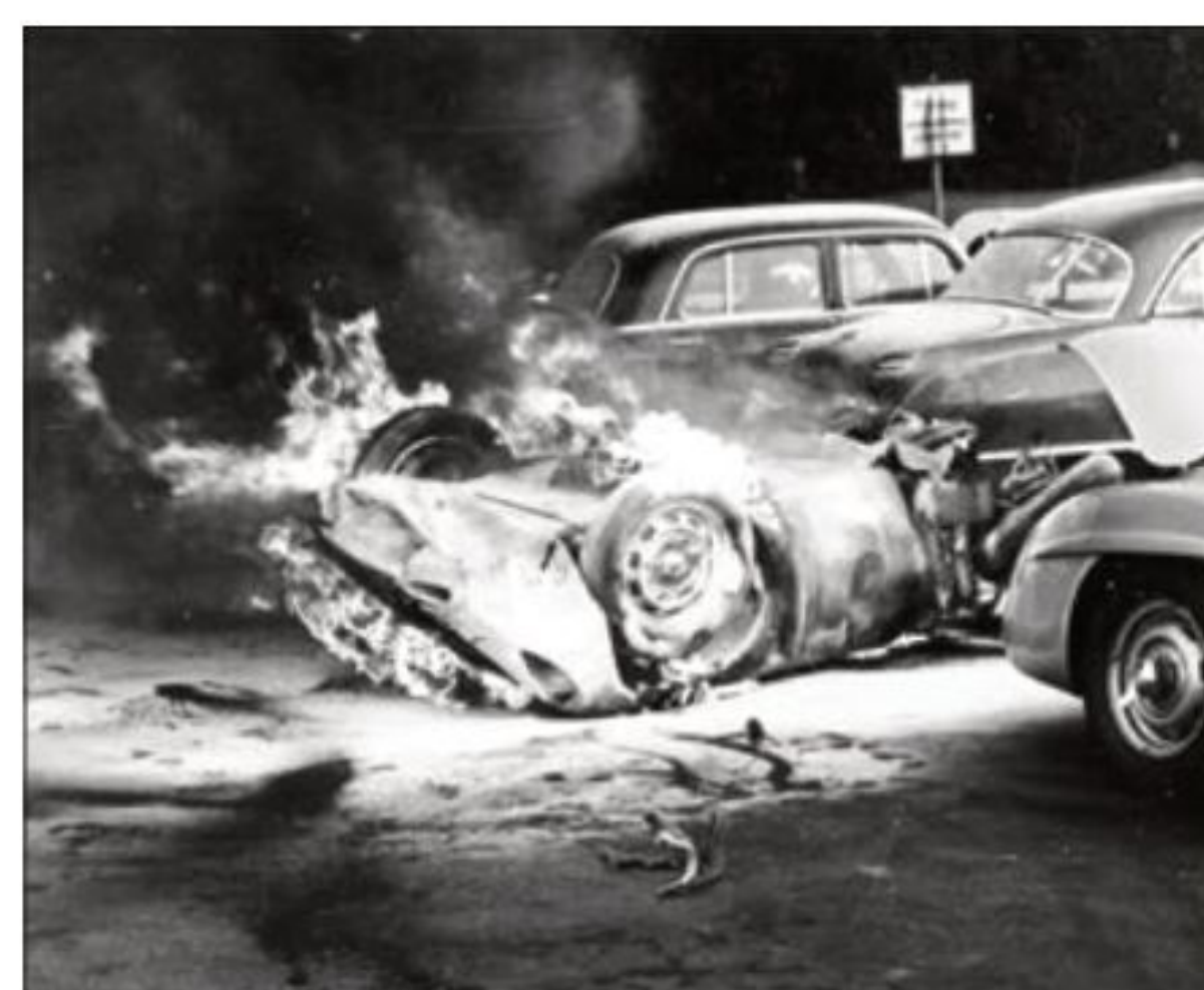
When the Type 645 landed, outside of the circuit, its nearly full fuel tank and magnesium body combined in this terminal inferno
