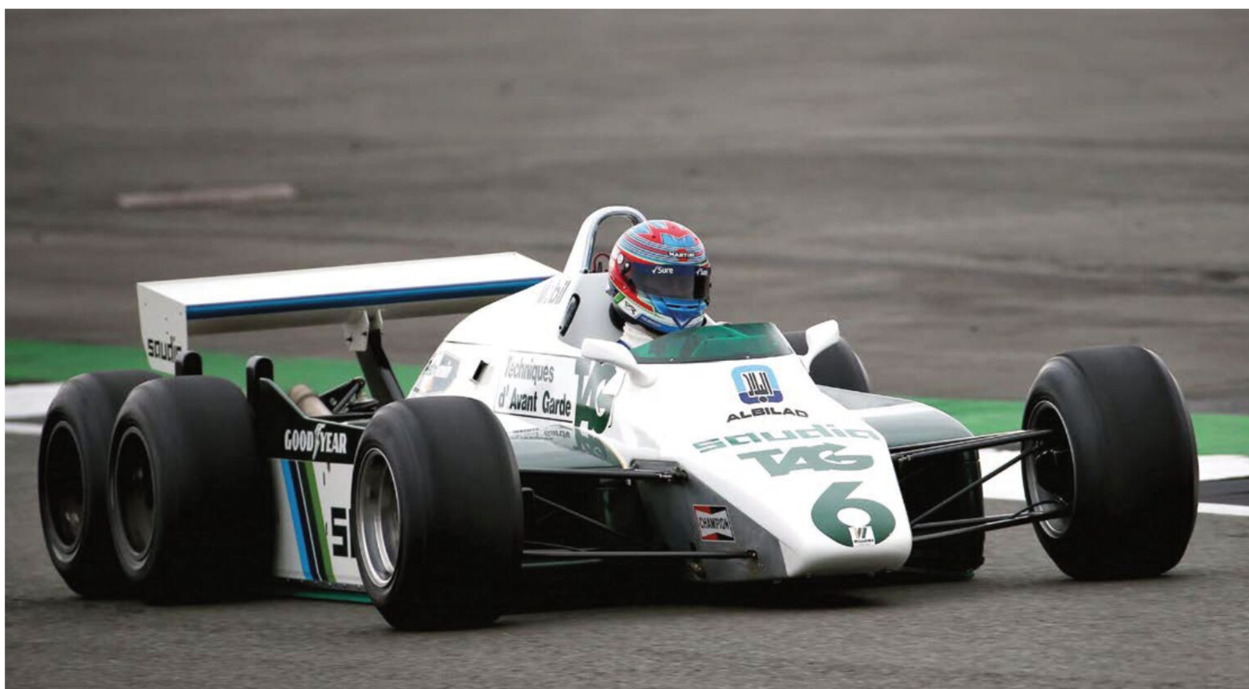
In 1981, Williams' Frank Dernie came up with the low-drag FW08B, in an attempt to keep its DFV engine competitive against the new turbo motors. The FIA banned it before it had a chance to race
