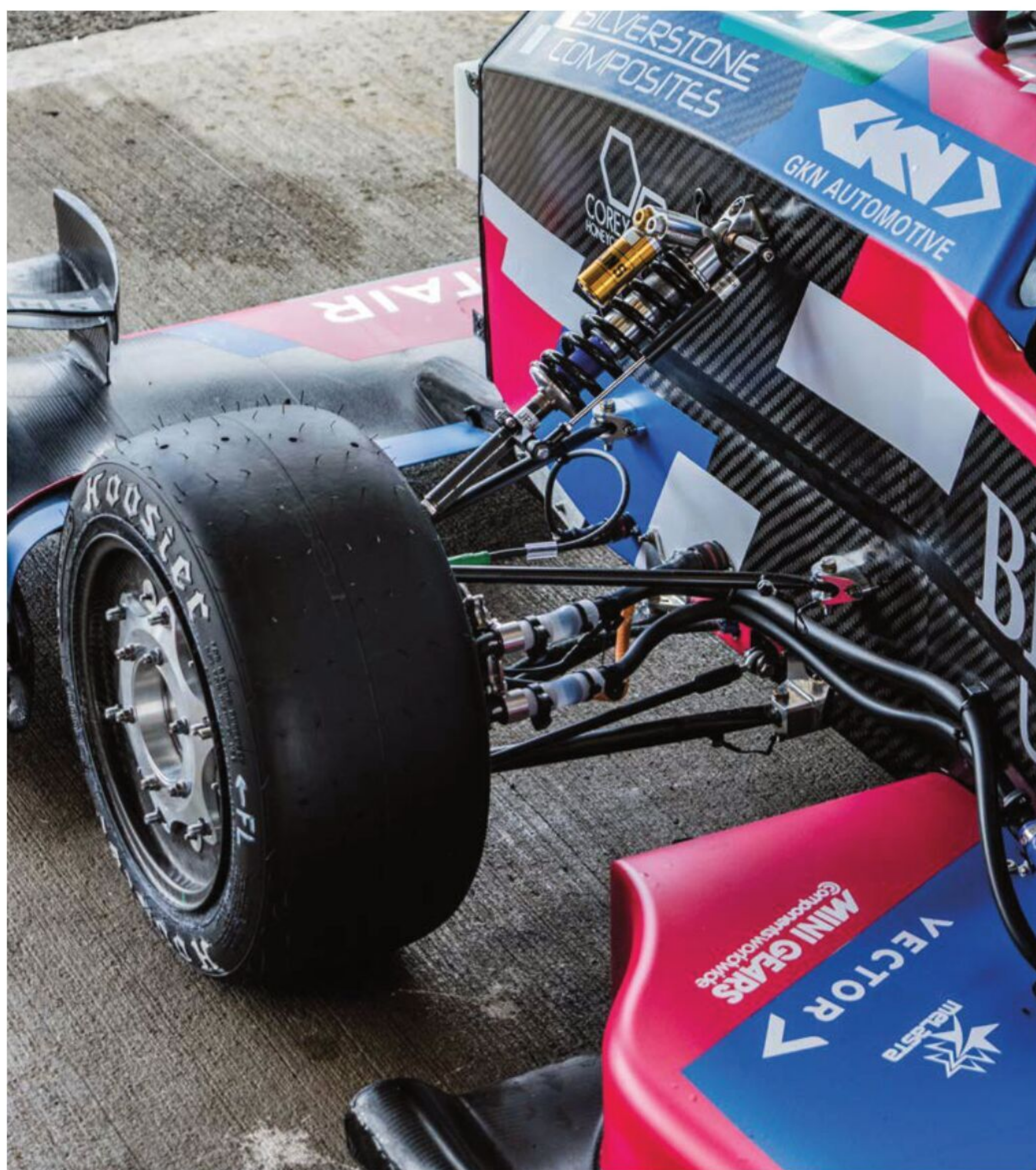
The four-wheel drive car features liquid cooled in-wheel motors. Note the coolant lines from the onboard heat exchanging system
