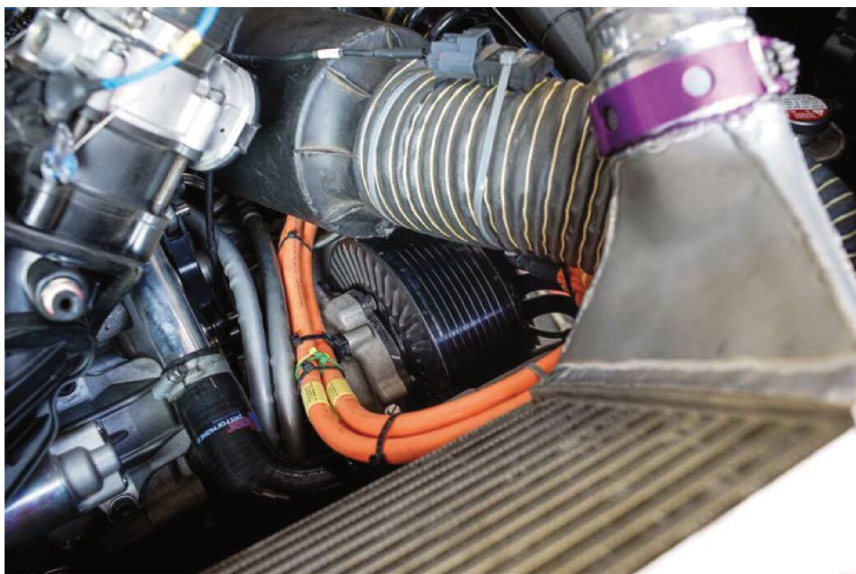
The three-phase electric motor is mounted in the P2 off-axis configuration inside all entries in the British Touring Car Championship
