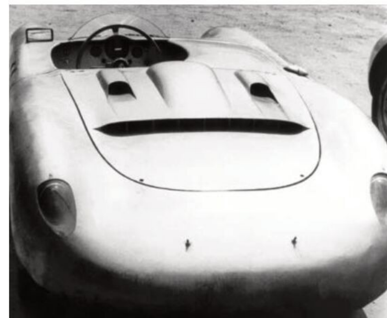
A rear view of the Type 645 Spyder, as readied for racing, showed its rear deck slot for engine cooling, rear-facing inlets for its twin carburetors and low-drag, faired-in tail lamps
