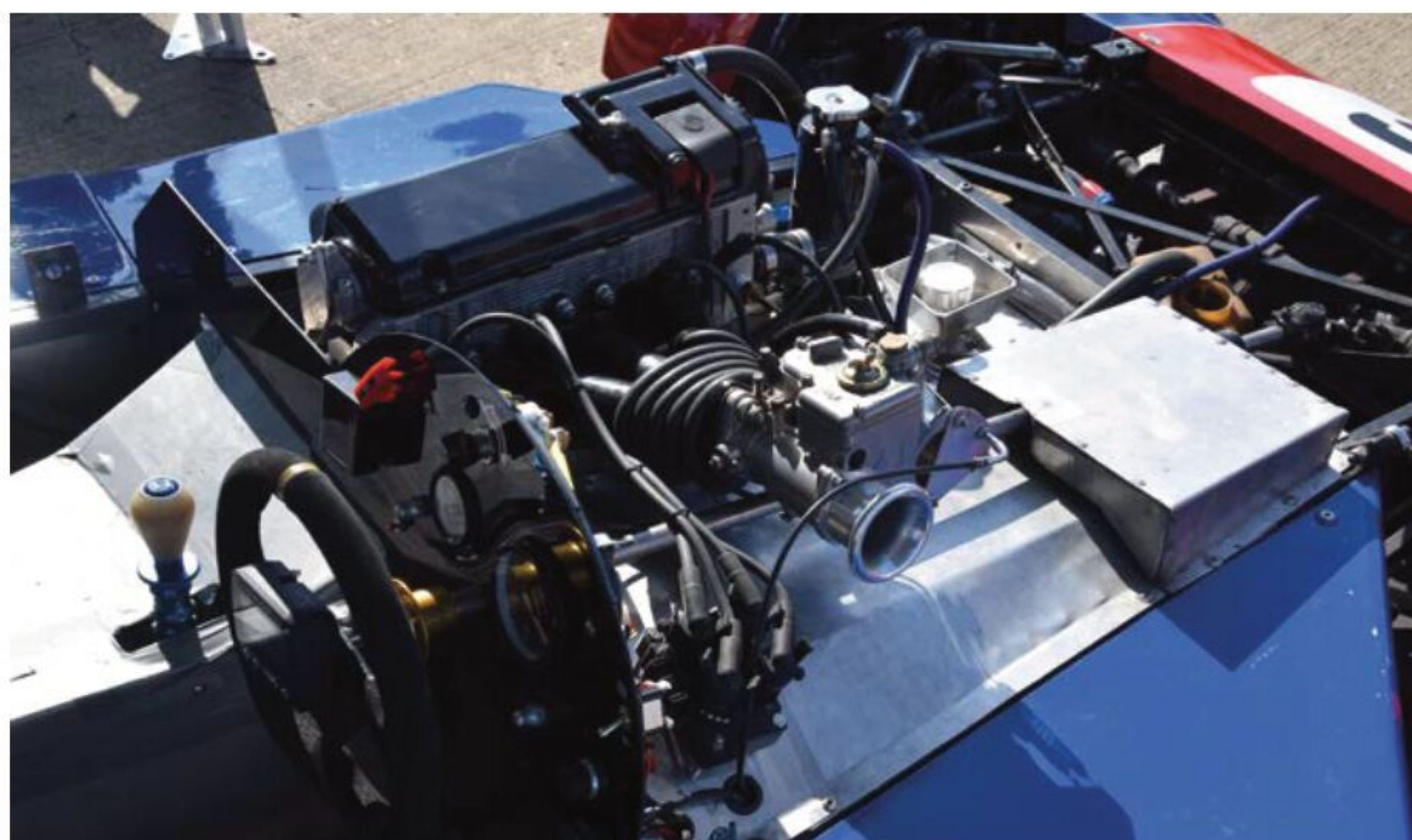
All cars competing in 750F run the Fiat 1108cc FIRE engine with single carburettor induction and a control camshaft. Engine positioning is free. In this Darvi, for example, it sits up front, very close to the driver
