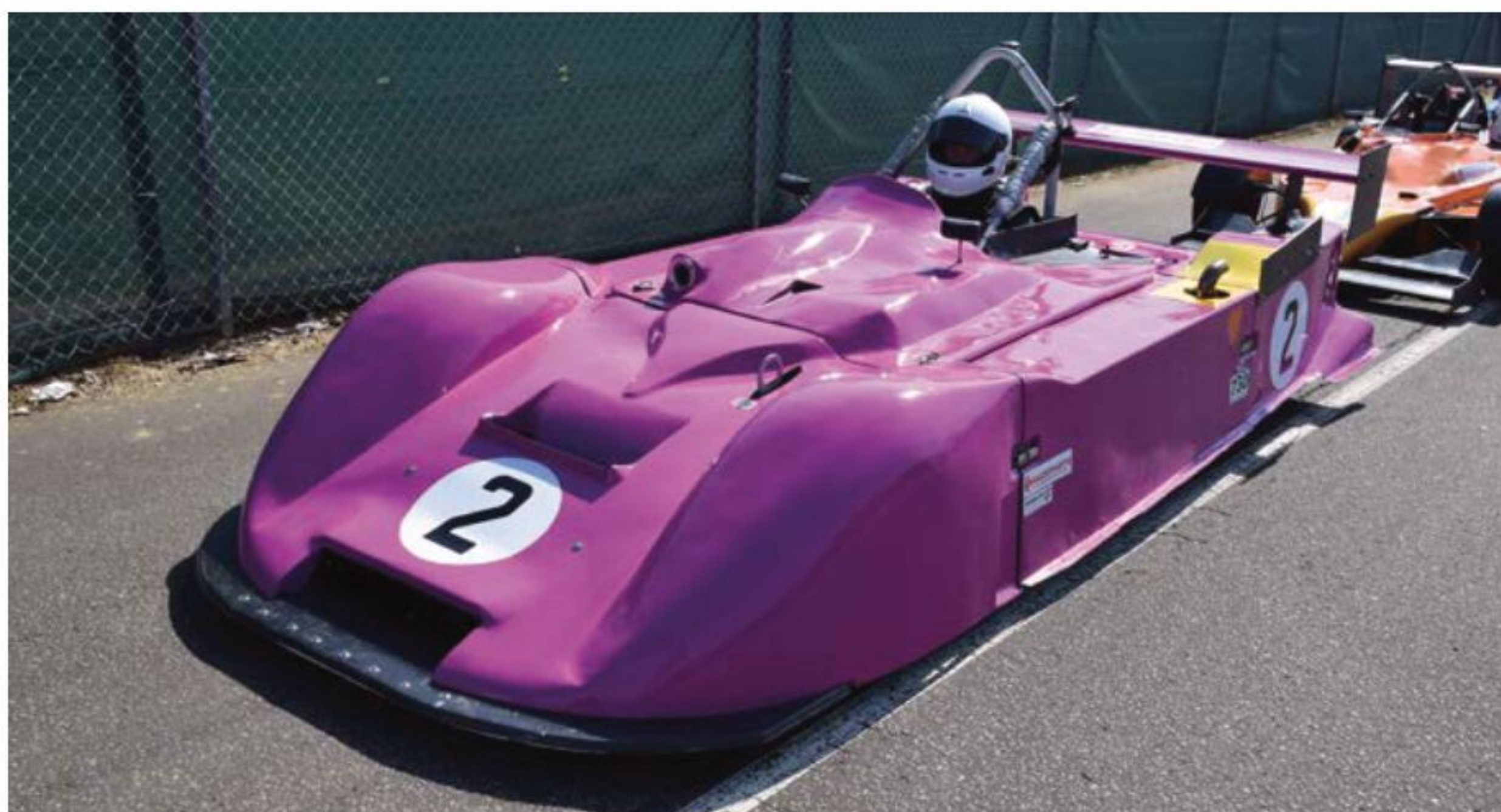
Looking more like a land speed racer, the design of Chris Gough's CGR2 Evo has taken the quest for straight-line speed to the extreme, but downforce generation has not been forgotten along the way
