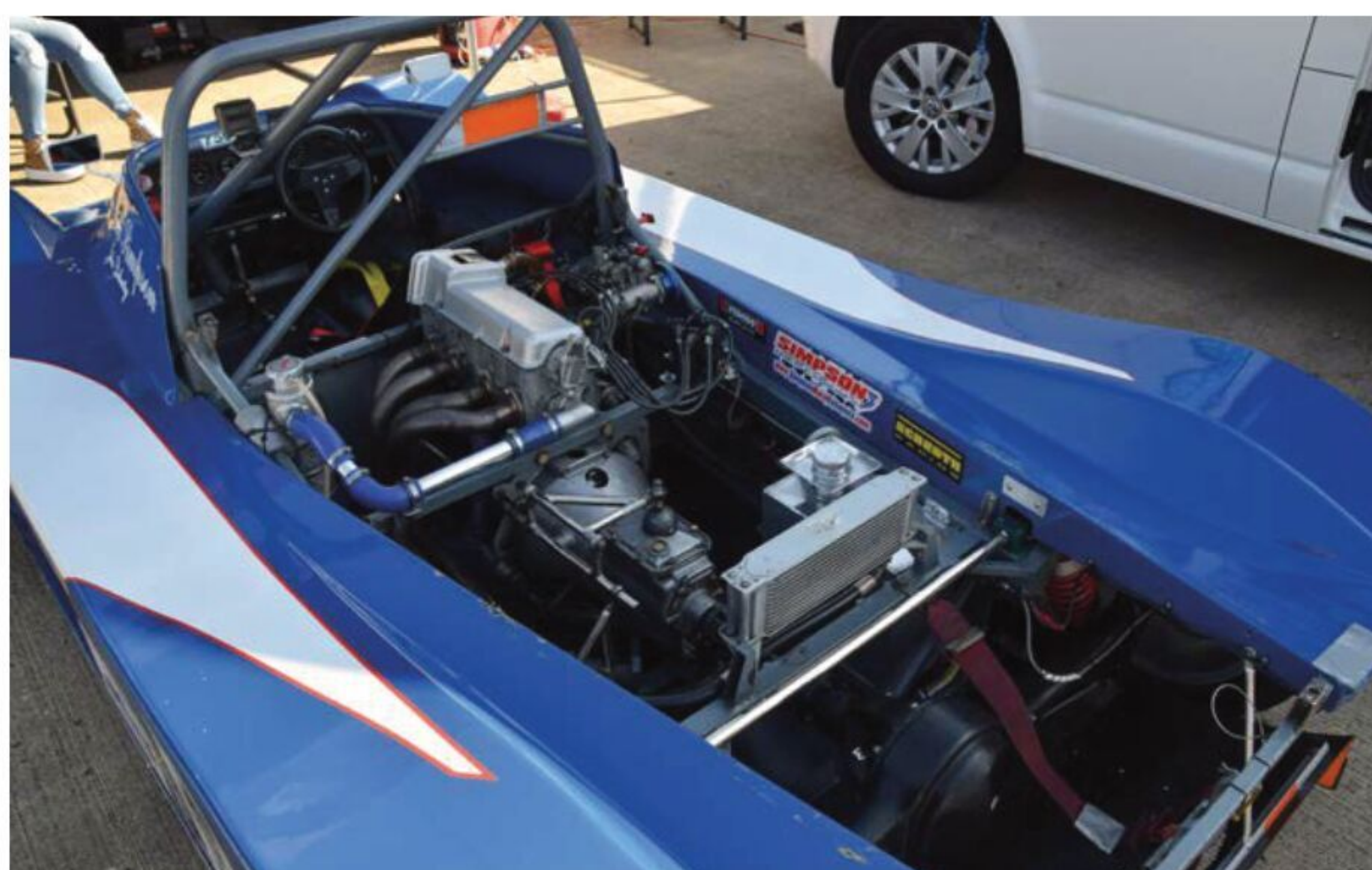
Bob Simpson has been racing in 750 Formula since 1968, and has driven this SS/F 750 for the last 30 years. The car was one of the first in the series to run with a rear-mounted engine
