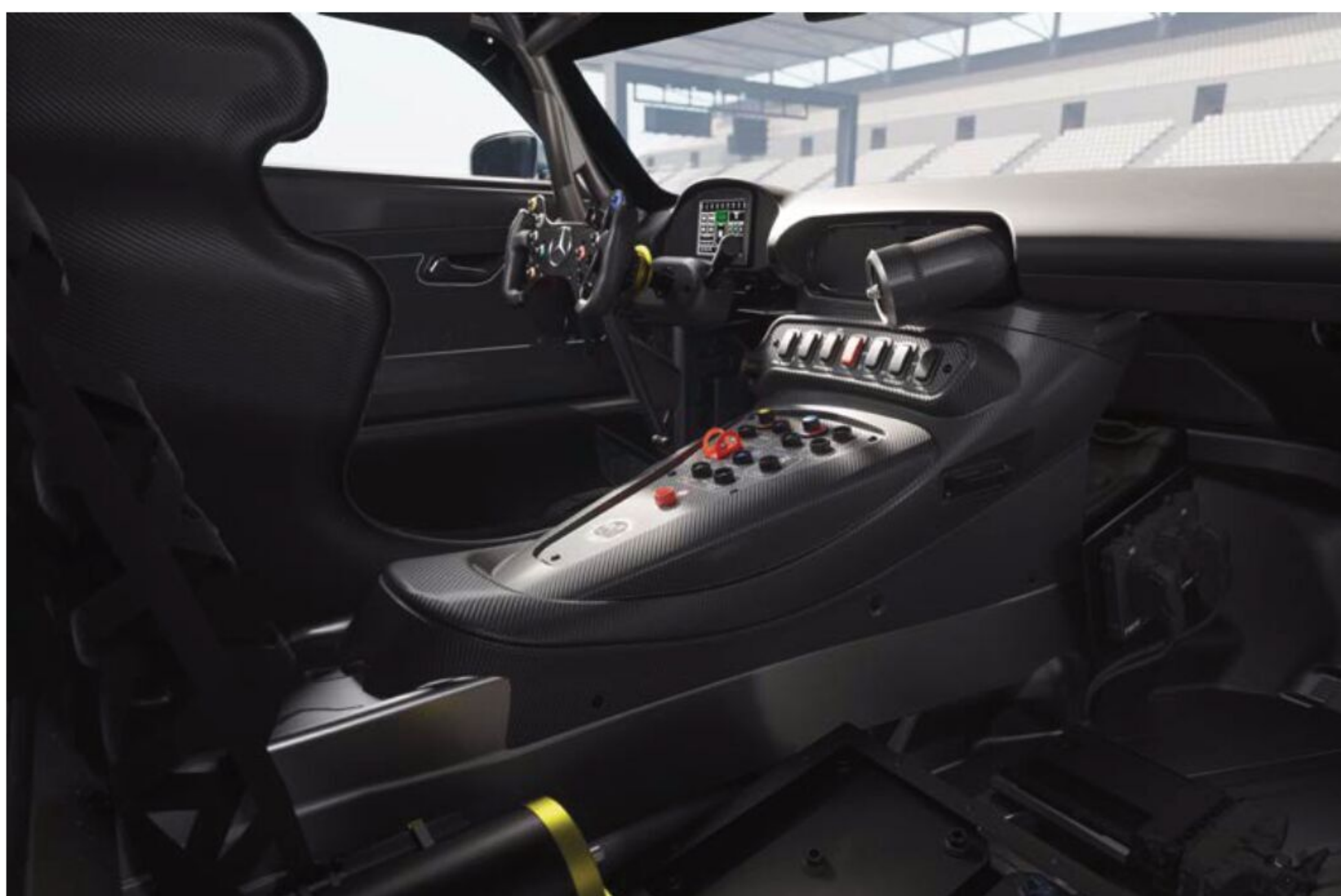
Keeping switches at eye level is particularly important in customer-focused racing where non-professional drivers will compete
