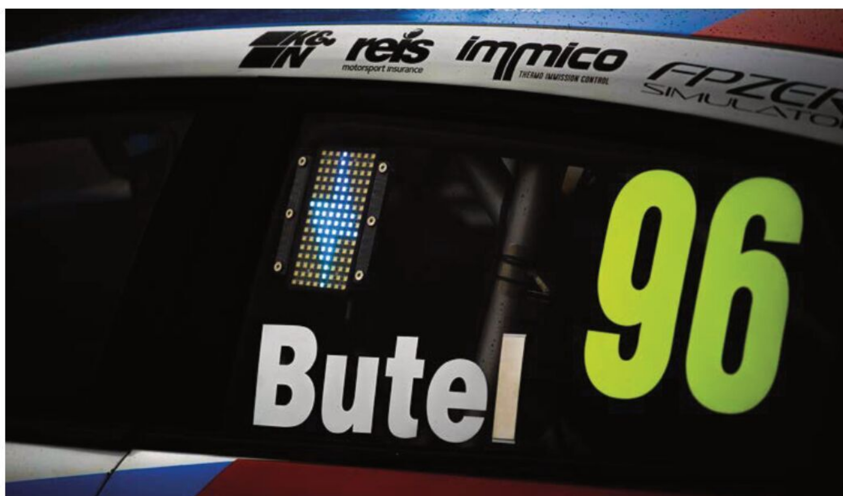
A blue lightning bolt illuminated in the window indicator shows fans and spectators when the hybrid system is being used
