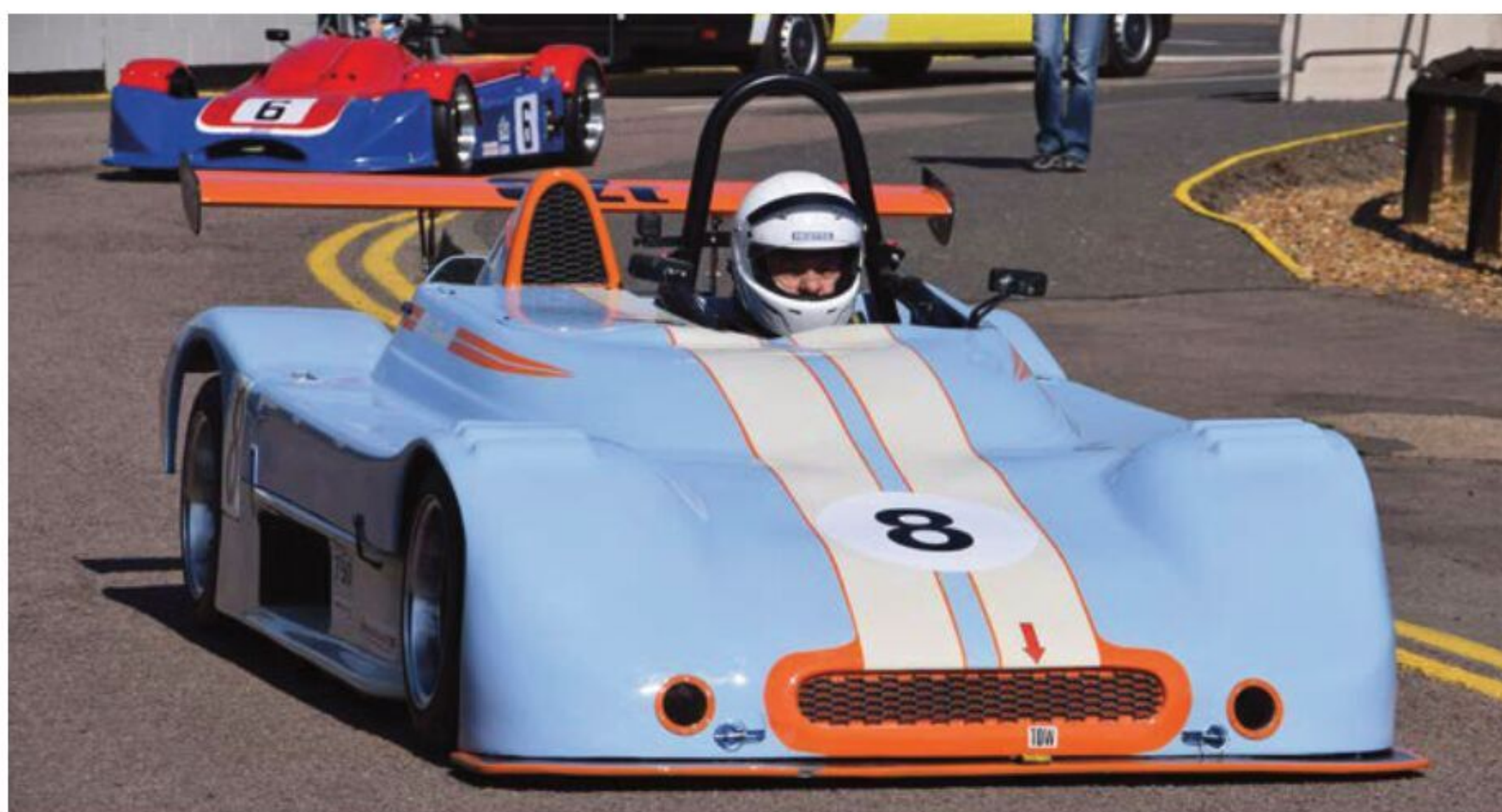
Bill Smith's SZT has a body derived from a kit car. The driver position is on the left, to help balance the weight bias resulting from the transverse-mounted engine
