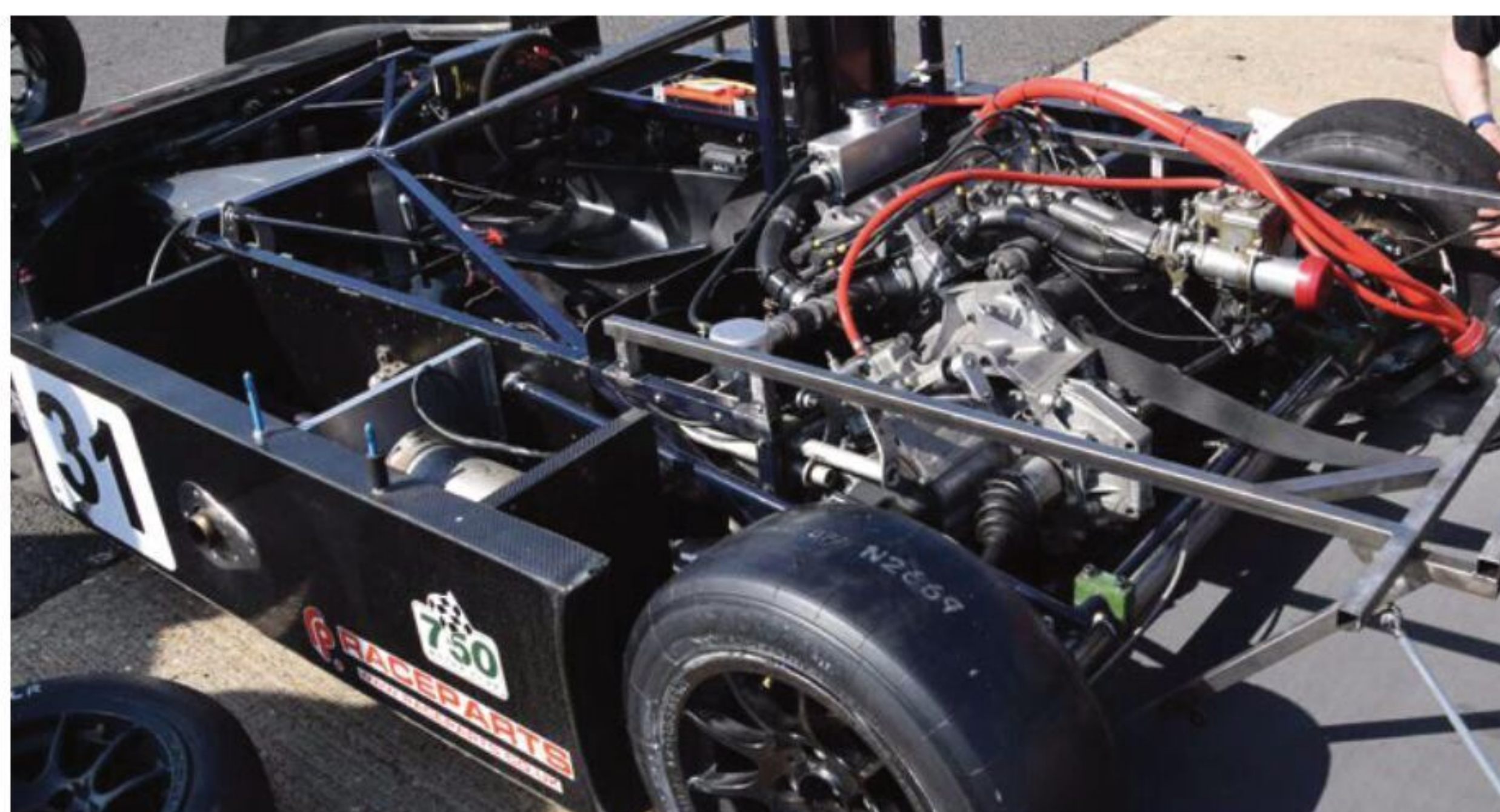
Chassis construction must be of metal, but otherwise is open to interpretation. This car has the engine mounted transversely in the rear, which means it has to use a production Fiat gearbox
