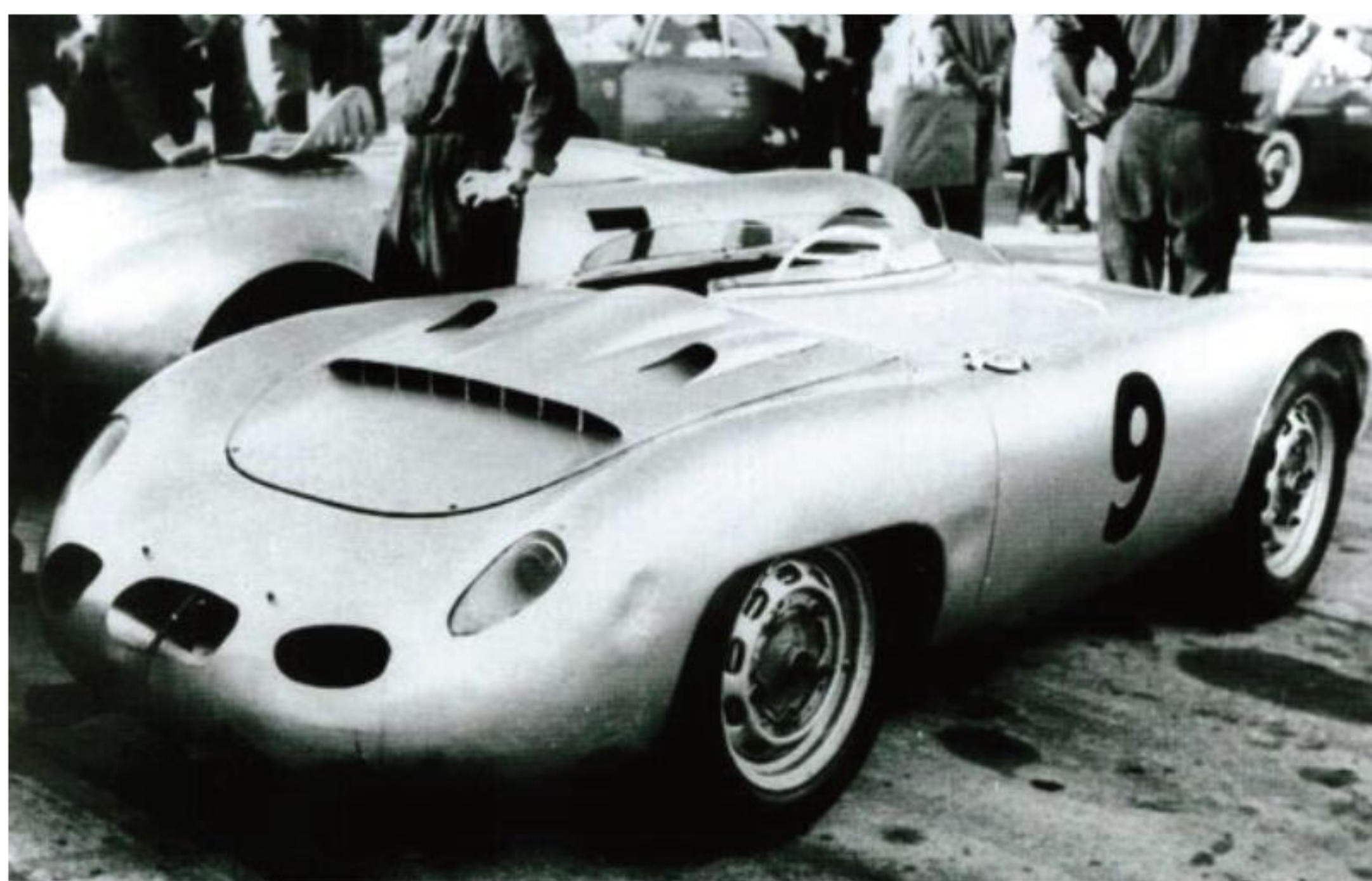
When the Type 645 next raced at the Avus on 16 September 1956, additional vents were cut in its tail to further assist engine cooling. Numerous dents are testament to the fragility of its magnesium bodywork
