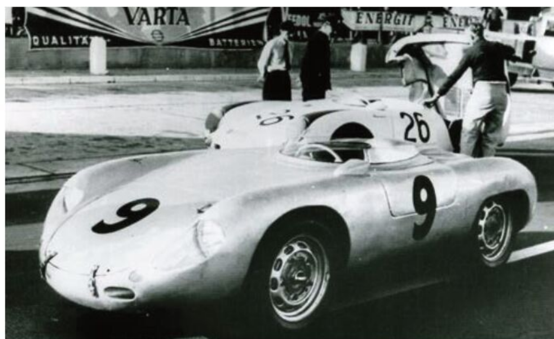
When the Type 645 next raced at the Avus on 16 September 1956, additional vents were cut in its tail to further assist engine cooling. Numerous dents are testament to the fragility of its magnesium bodywork
