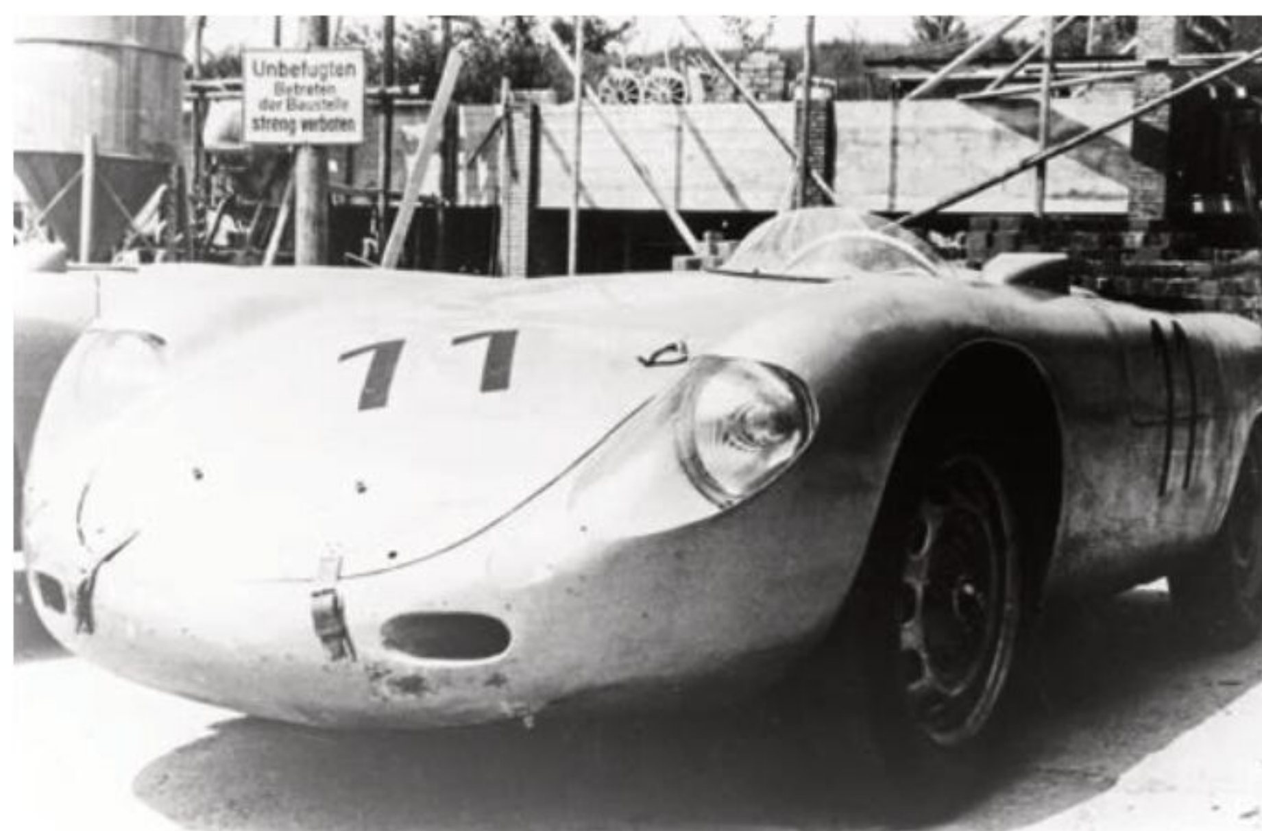
The Type 645's front view at Solitude displays its faired-in headlamps and the front lid that served as a surface cooler for the engine oil, the filler for the tank sited behind it
