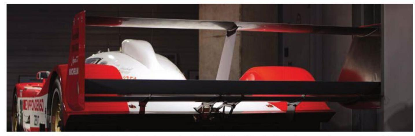
Biplane rear wing fitted to the TS010. The lower beam wing has the job of working the floor, the upper wing controls aero balance
