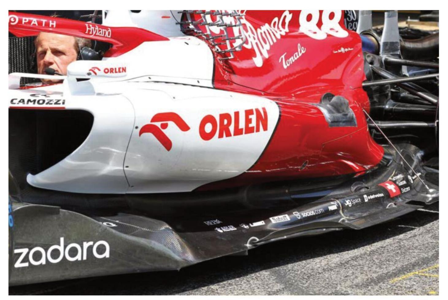
Deeply sculpted section under sidepod leaves space for upper floor surface to interact with under-floor flows and other aero devices
