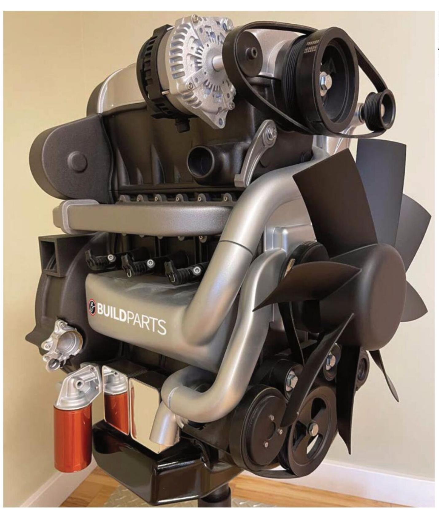
CIDEAS used FDM, SLA and CLIP processes to create this highly detailed 100 per cent 3D printed trade show display engine model
