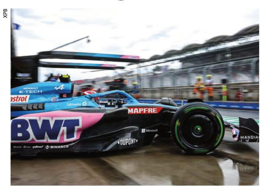
It's hoped F1's porpoising issue will be solved with changes to the plank and skids this season, and to the floor from next year; including lifting the outer edges by 15mm and raising the diffuser throat
