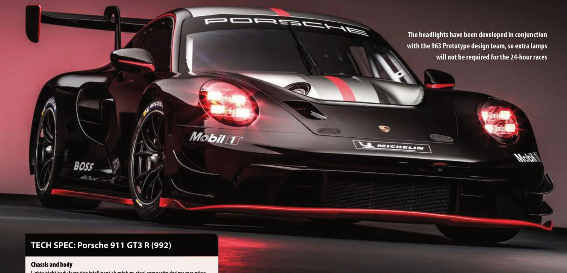
Lightweight body featuring intelligent aluminium-steel composite design; mounting points for lifting device; removable rescue hatch in the roof; welded-in roll cage; approved for co-driver use on circuits.
