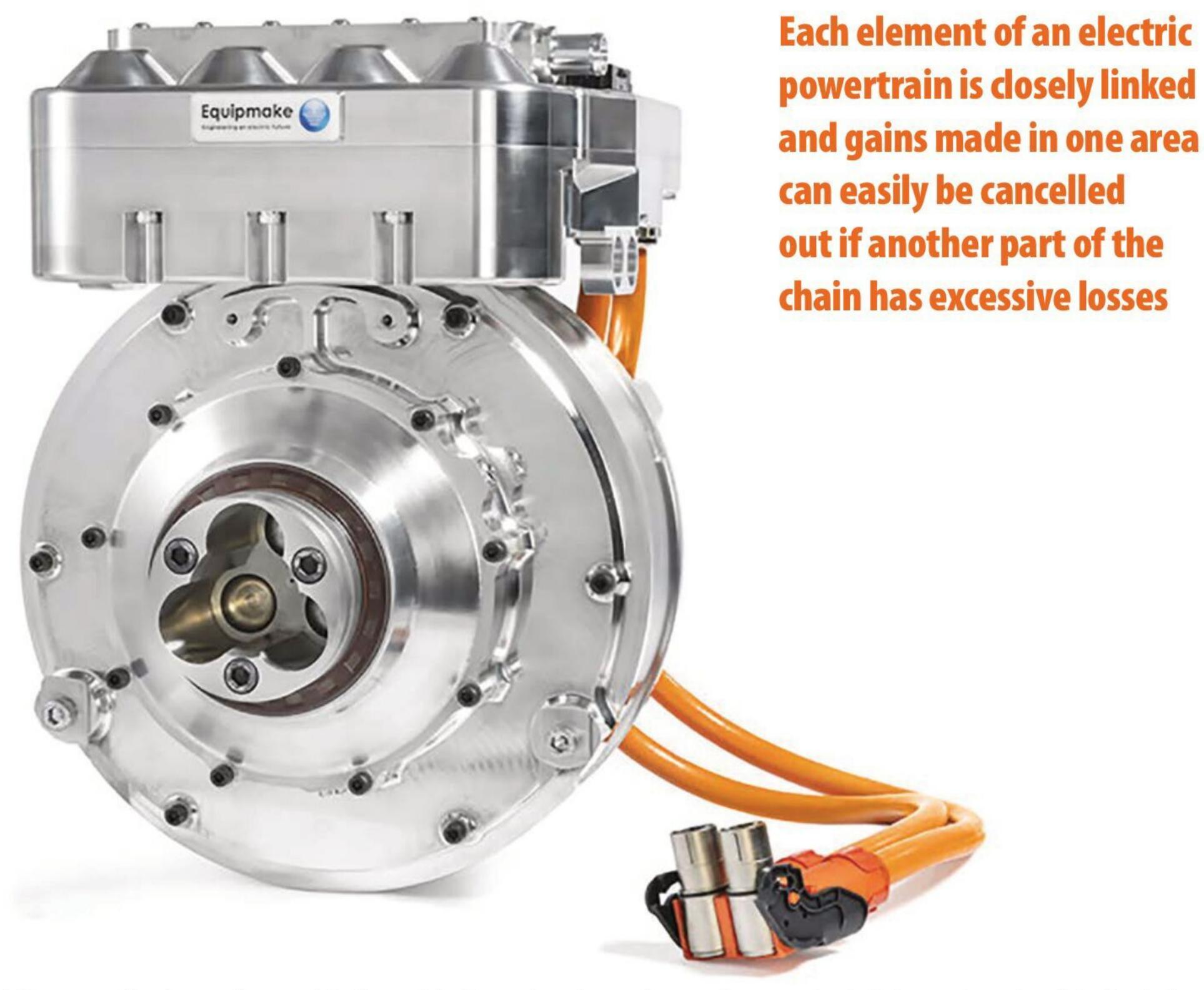
An axial flux e-motor with an integrated inverter unit. In this type of electric motor the gap between the rotor and stator, or rather the flux between the two, is parallel to the axis of rotation
