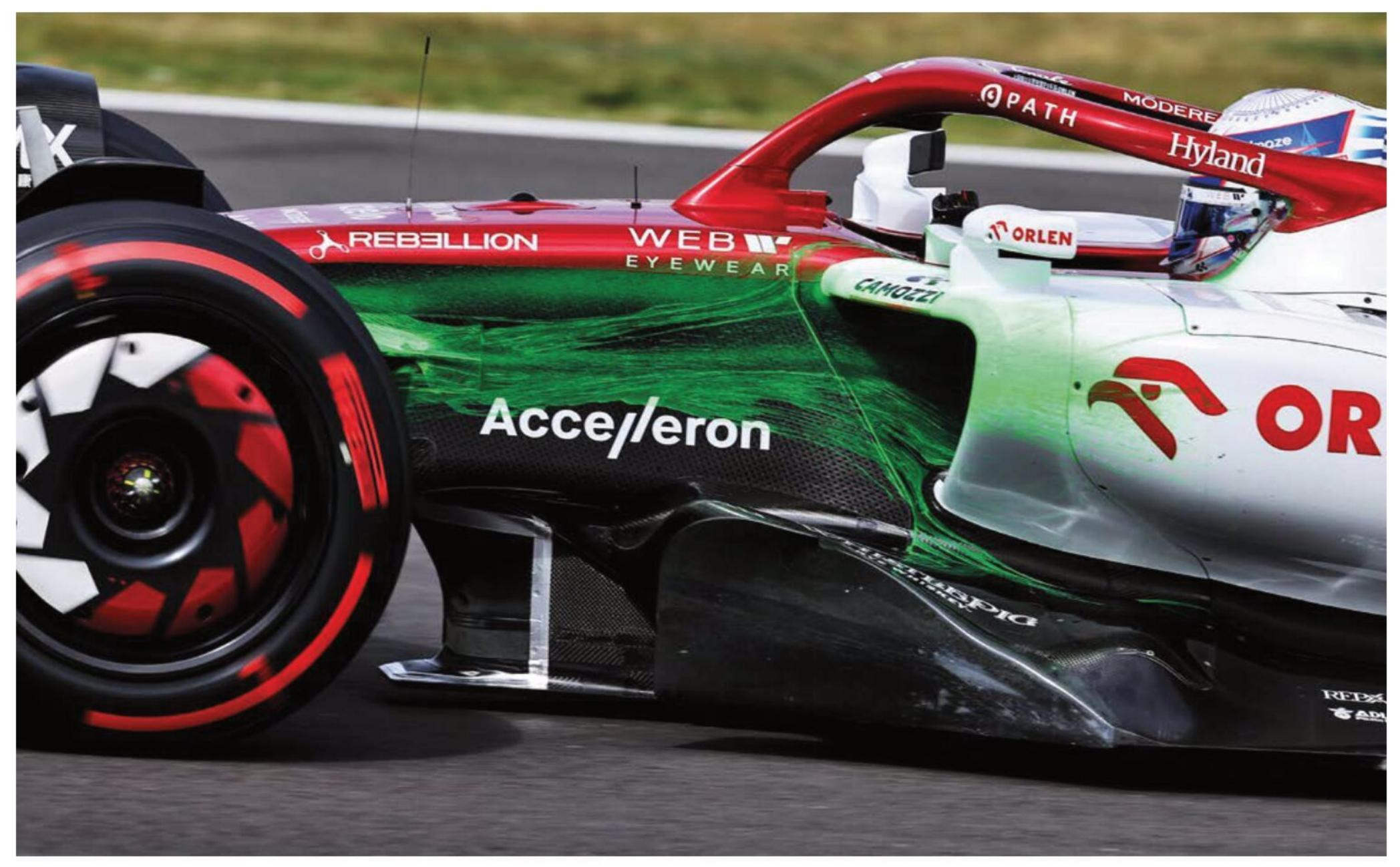
Green flow viz paint sprayed on to the front of the Alfa Romeo C42 clearly shows the airflow converging behind the front wishbones before going on to expand as it enters the sidepod opening
