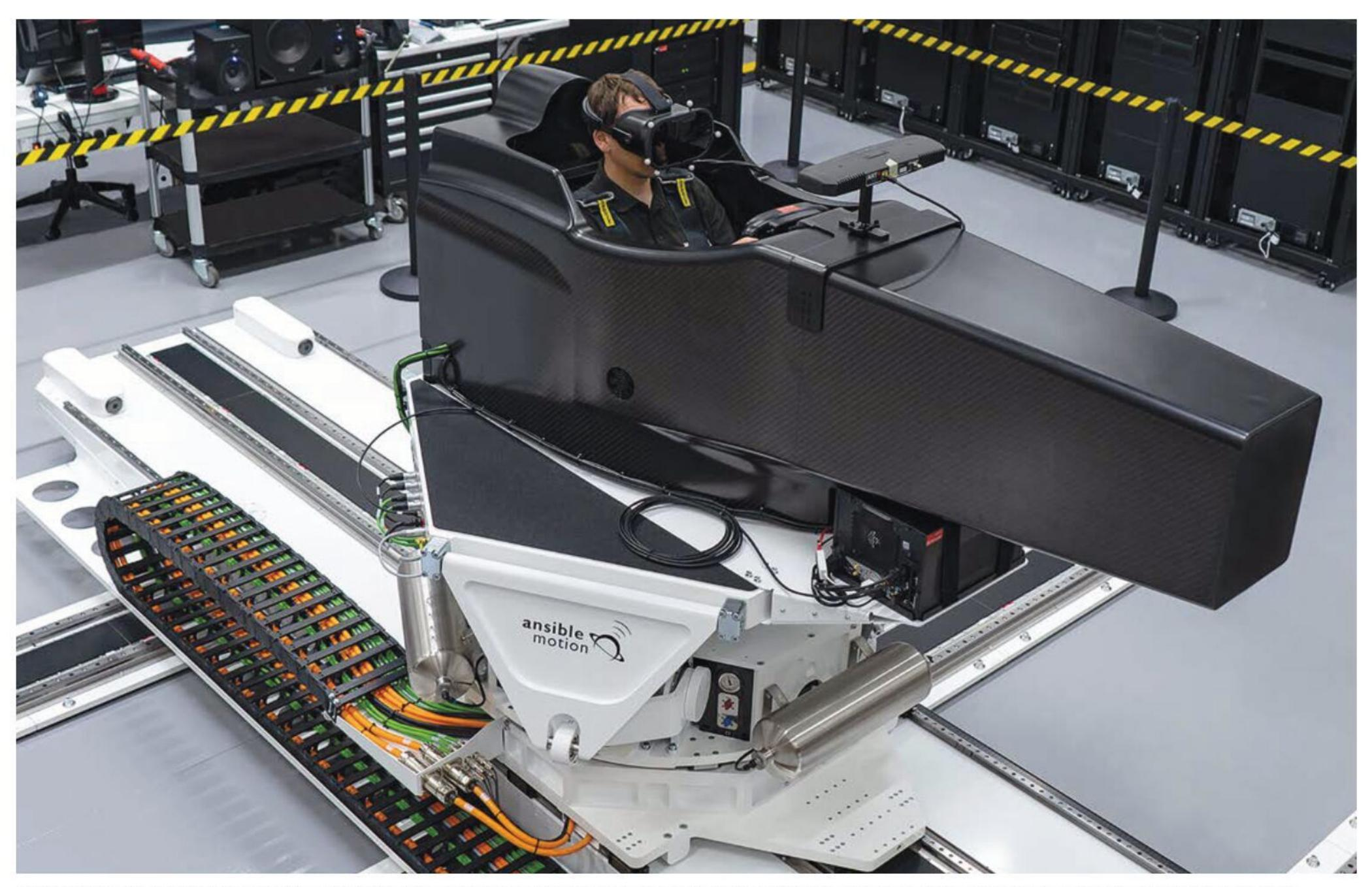
Ansible Motion's Delta S3 DIL simulator in action. While hi-tech kit such as this has long been used for driver training it can now also play a part in the overall development of the racecar
