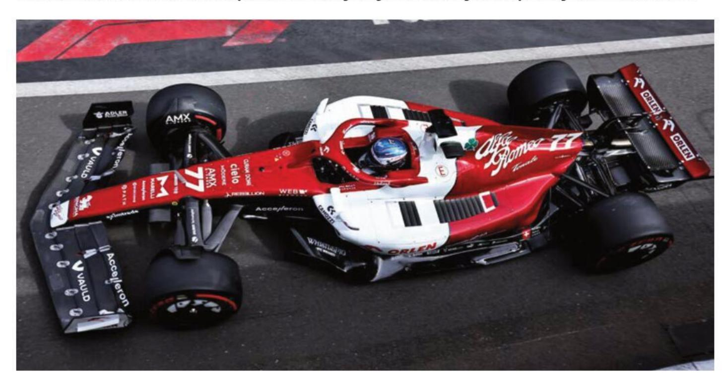
In cool conditions blanks are placed over the sidepod louvres to keep the desired pressure and temperature delta across the coolers
