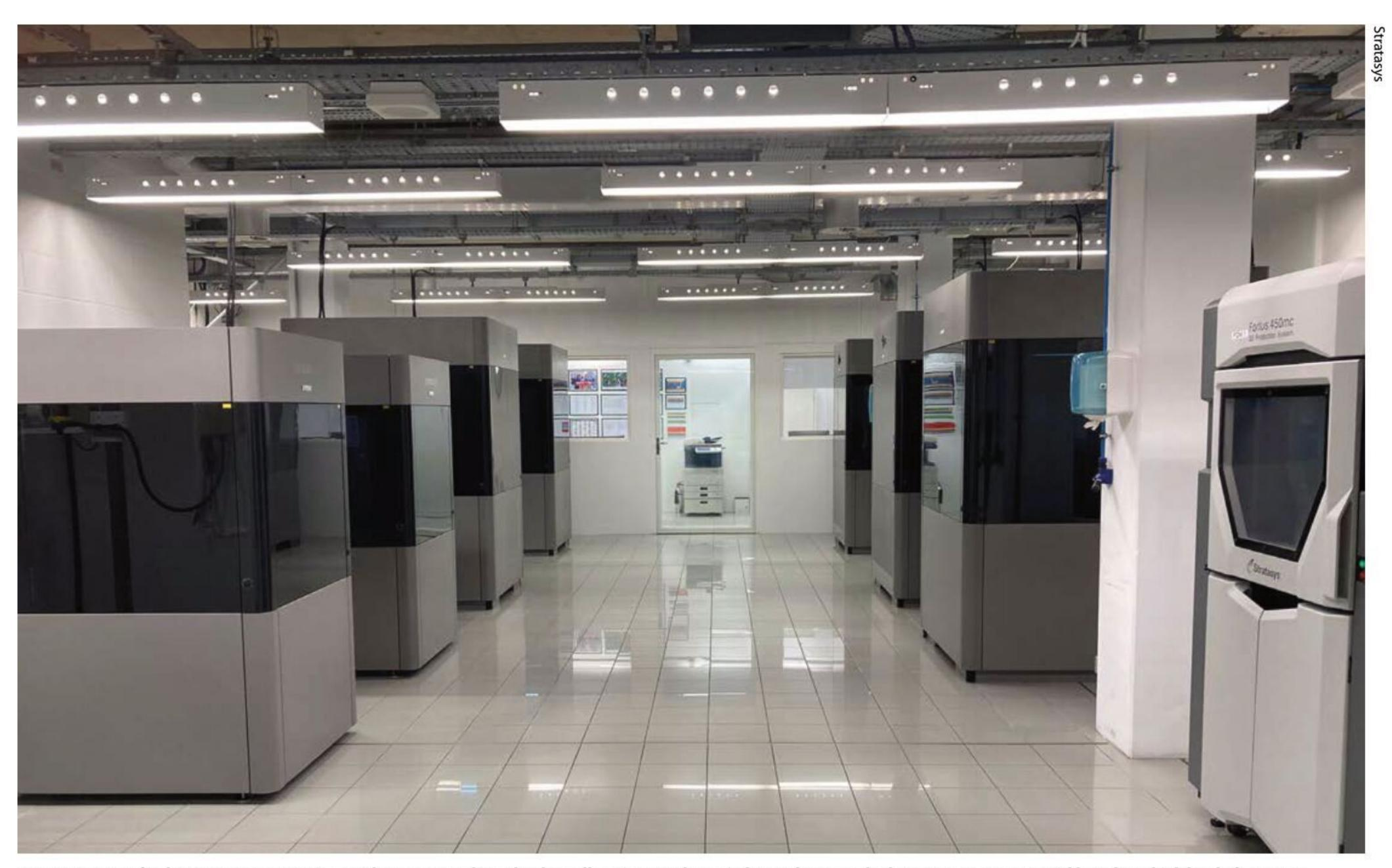
McLaren's array of in-house Stratasys 3D printers. The team says the technology allows it to produce wind tunnel parts and other components very quickly and to a high level of accuracy
