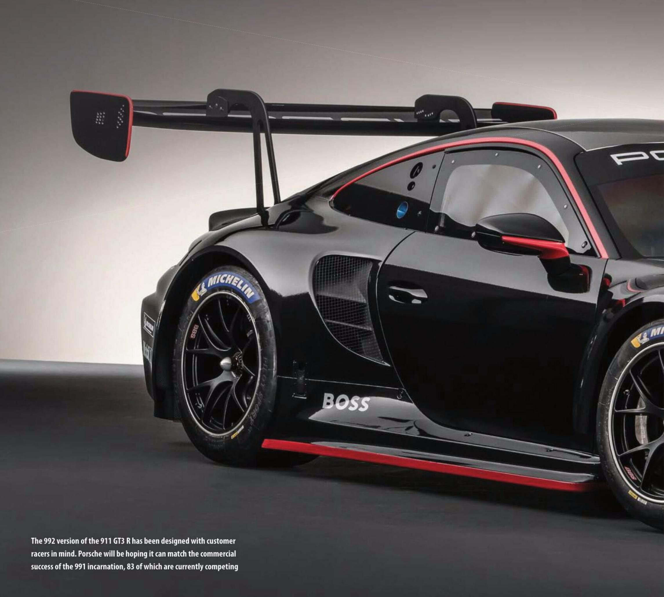
car has now completed its test programme and will be made available for competition starting at the Daytona 24 hours in January 2023. The company has made a number of changes to its previous model, including revised aerodynamics, an engine upgraded to 4.2 litres, wider track, longer wheelbase and a wealth of safety features, all targeted at making the car easier to drive, more durable and also faster.
