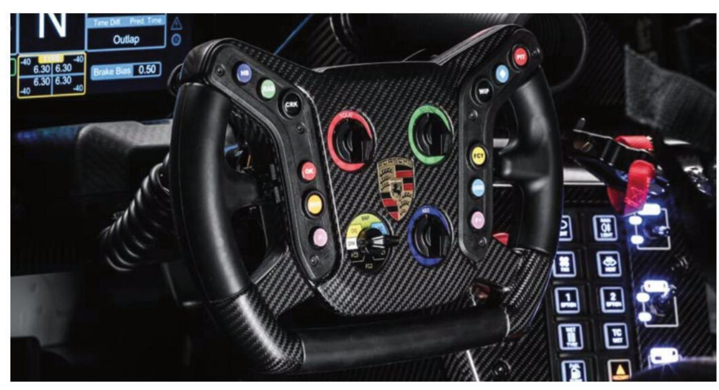
Shift paddles on the Porsche wheel actuate a 6-speed constant-mesh gearbox which is derived from the current 911 GT3 Cup racecar
