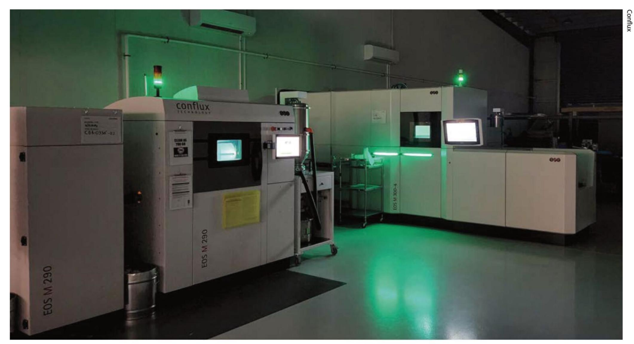
Producing parts on-site at Conflux's vertically integrated additive manufacturing facility. AM technology is ideal for making the complicated heat exchangers the company specialises in
