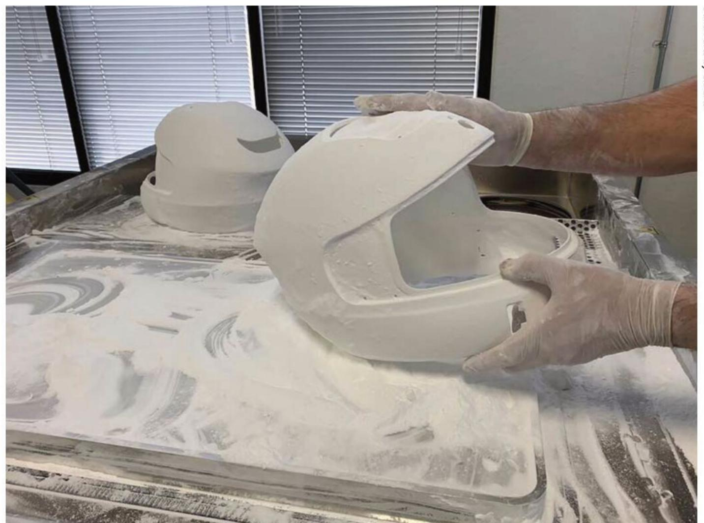
SLA (stereolithography) was used to produce this HUD Navigation smart motorcycle helmet demonstrator. Accura 25 resin was chosen for its accuracy, durability and heat deflection. The process, which cures a resin with UV light, gives a good surface finish
