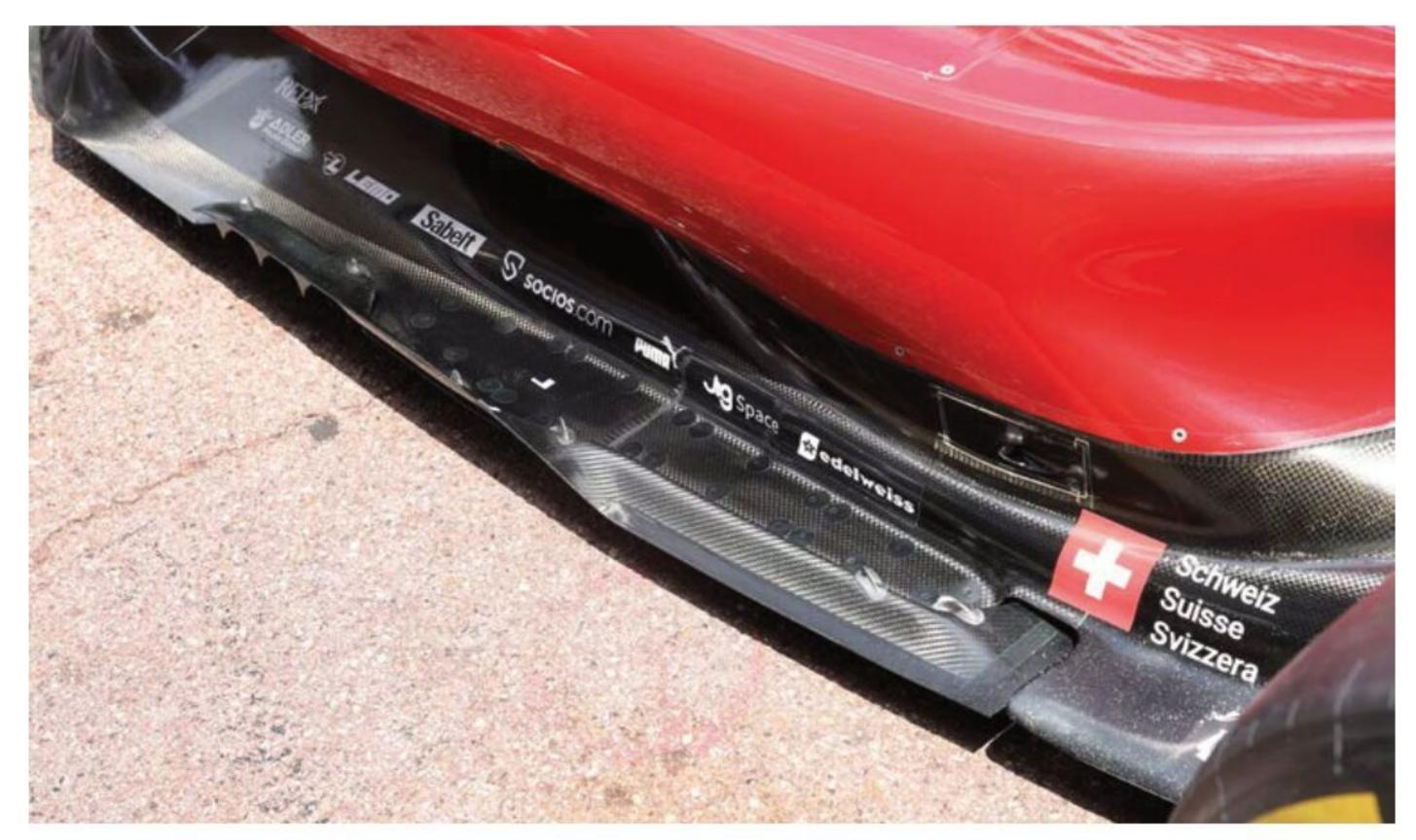
An exit flow device positioned midway down the C42's floor rejects airstream that isn't attached to the tunnel flow under the car
