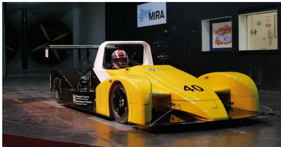
Final figures were verified by independent CFD, on track through pushrod load sensors and in controlled conditions at the MIRA tunnel
