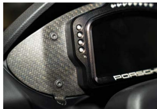
Close up of one of the interior components of the Porsche 718 Cayman GT4 Clubsport MR made from Bcomp natural fibre materials
