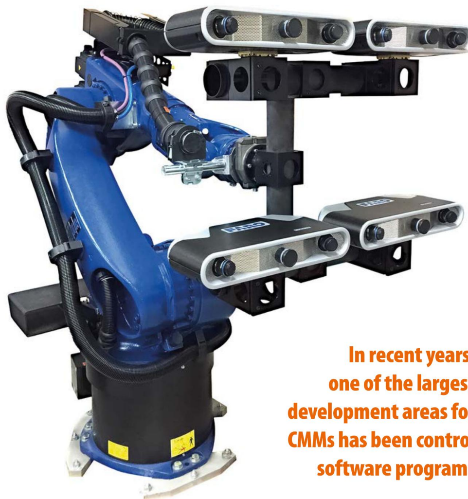
An example of a metrology array, used to measure the surfaces of a vehicle to correlate CAD files to final product dimensions
