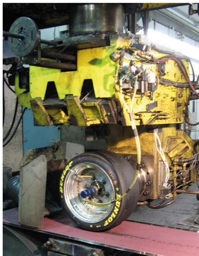
On a flat track tyre testing machine what is positive or negative camber? Which direction is the belt moving? Is it a right or left wheel? Hence the notion of inclination angle
