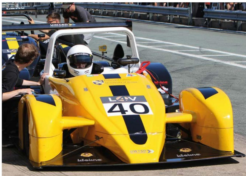
The newly bodied car, now called the MCR S2N, features pontoons over the front wheels and deep channels either side of the nose structure. The splitter is also both longer and wider
