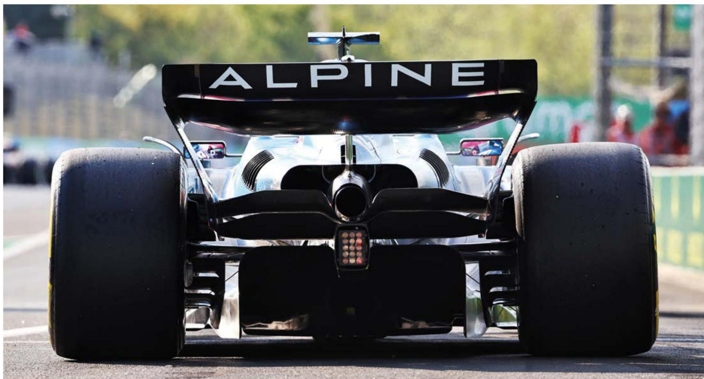
The beam wing has a strong influence on the diffuser. The rear wing, beam wing and diffuser are only powerful in the current aerodynamic regime when they work in harmony
