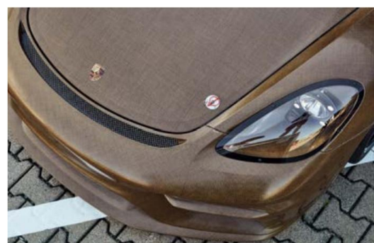
Porsche 718 Cayman GT4 Clubsport MR with natural-fibre composite exterior formed using ampliTex and powerRibs
