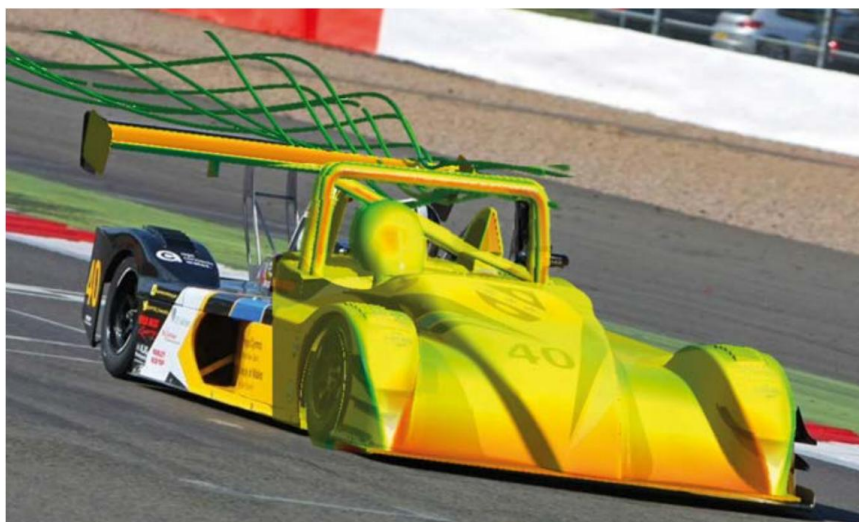
CFD merge of the original car showing the flow over the control rear wing. While this aerodynamic device is not particularly effective, the real issue with Sports 2000 racers is understeer
