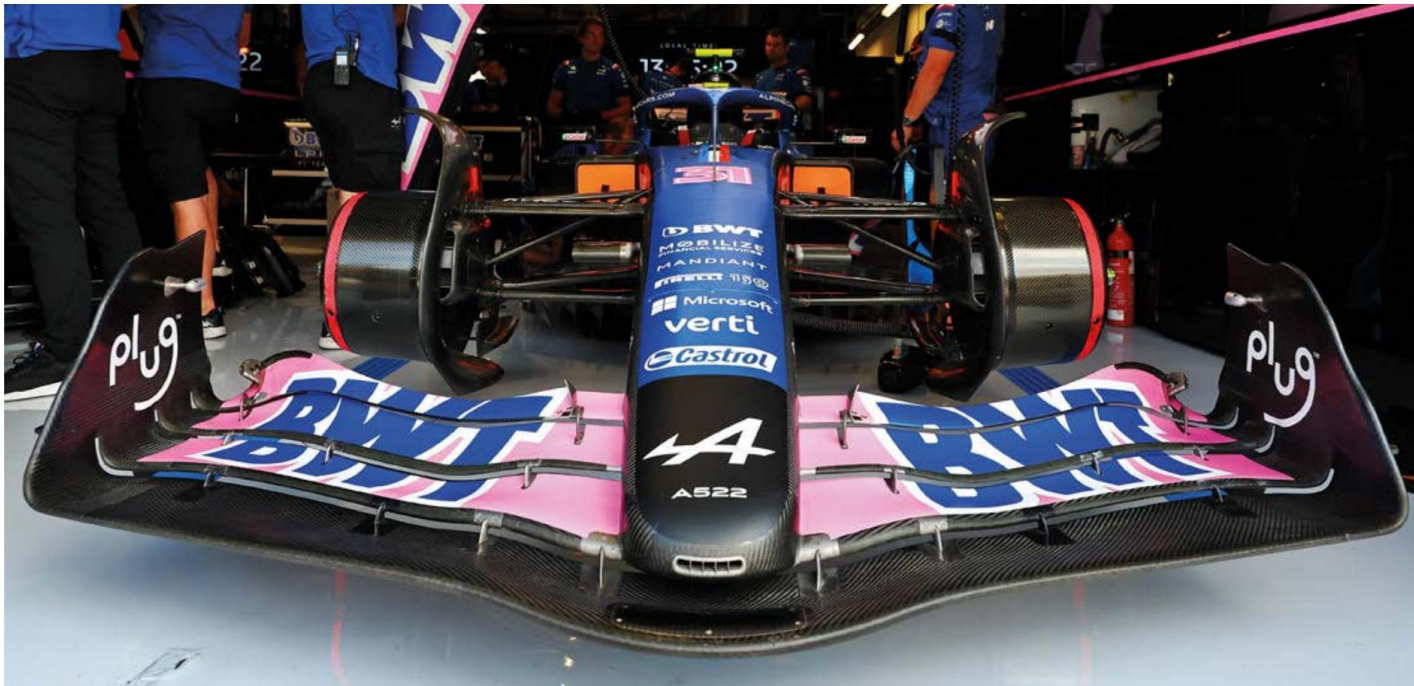
Due to changes in regulation with regard to ground effect floors, Alpine's front wing now plays more of a flow conditioning role in ordering the flow field towards the front of the floor
