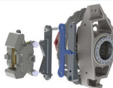
Fig. 1: AVL's new dynamic Brake Torque Sensor is mounted directly between caliper and knuckle
