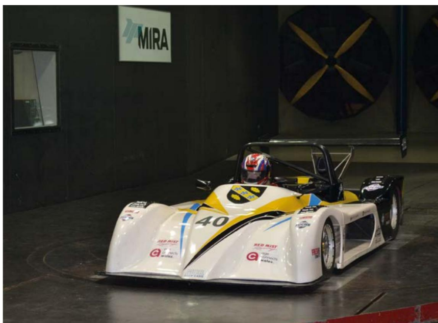
The car with the old bodywork, here without dive planes, was taken to the MIRA wind tunnel to validate the CFD model
