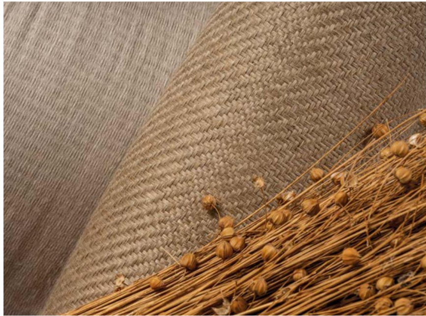
AmpliTex reinforcement fabric (dry), showing the natural fibre its made from and two different weave patterns
