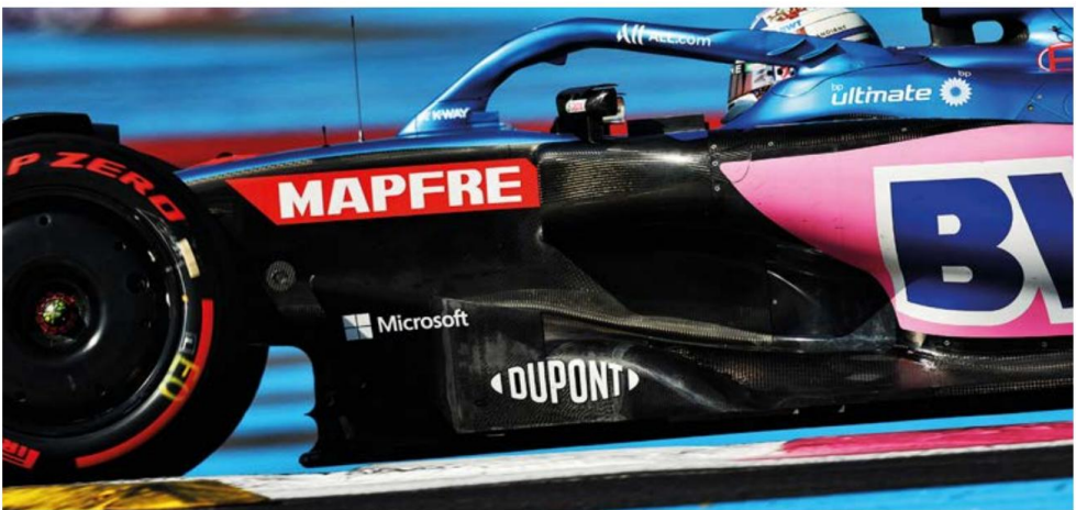
The A522's post-Silverstone sidepod design features a deep sculped section under the sidepod to leave space for the upper floor surface to interact with the underfloor flows and other aerodynamic furniture at the rear of the car
