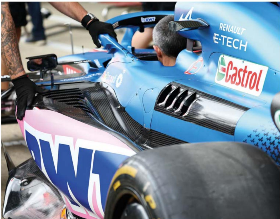
The A522 is designed to allow significant changes to be made to the body without needing to alter the position of underlying systems
