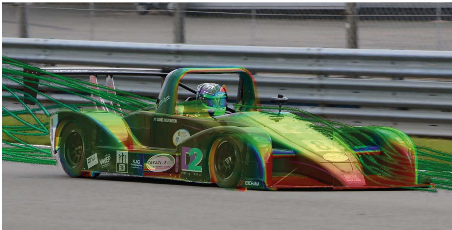
CFD study from Trinity St David blended with an on-track image of the MCR S2N. Work by students on the university's motorsport engineering course has transformed the aero on this Sports 2000 racer
