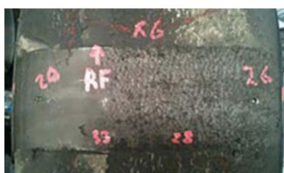
Pic 2a: Example of a racecar development OptimumG was involved in. Initially, we had very uneven front tyre wear and major loss of performance in just a few laps because of a very long VSAL. Only a small part of the tyre is working, and a major part has serious graining
