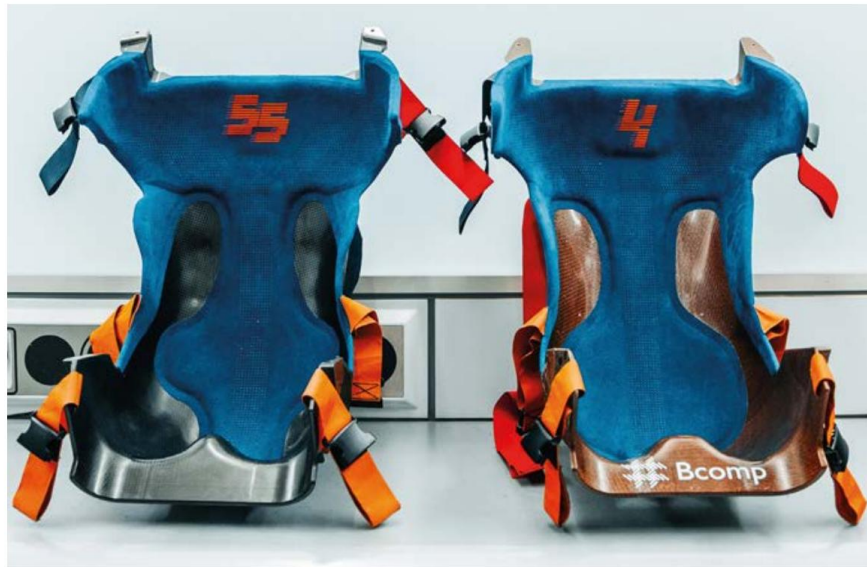
McLaren racing seat with Bcomp ampliTex and powerRibs integrated into the structure
