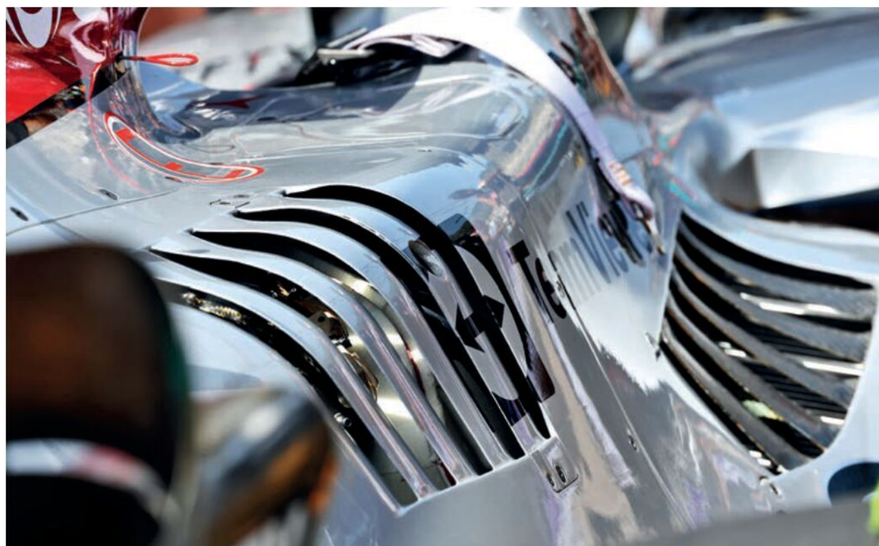
Mercedes' charge air cooling is based on water-to-air heat exchange and coincides with the design philosophy of the car. This allows the car to run fewer cooling louvres in the body than many of its competitors
