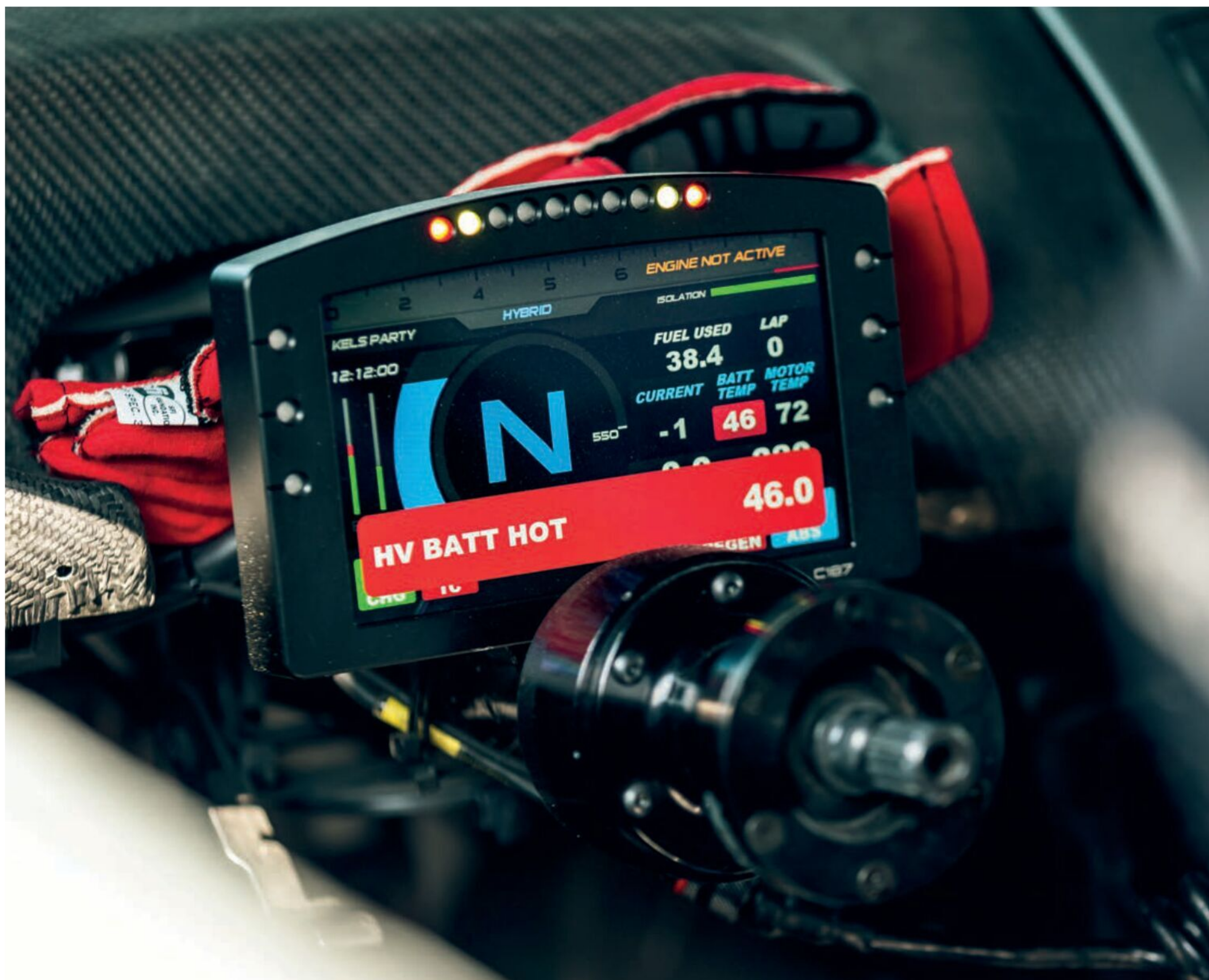
Keeping the driver abreast of battery conditions is an essential part of running a hybrid racecar, and the ECUs onboard have to monitor this and respond to different torque requests on the go
