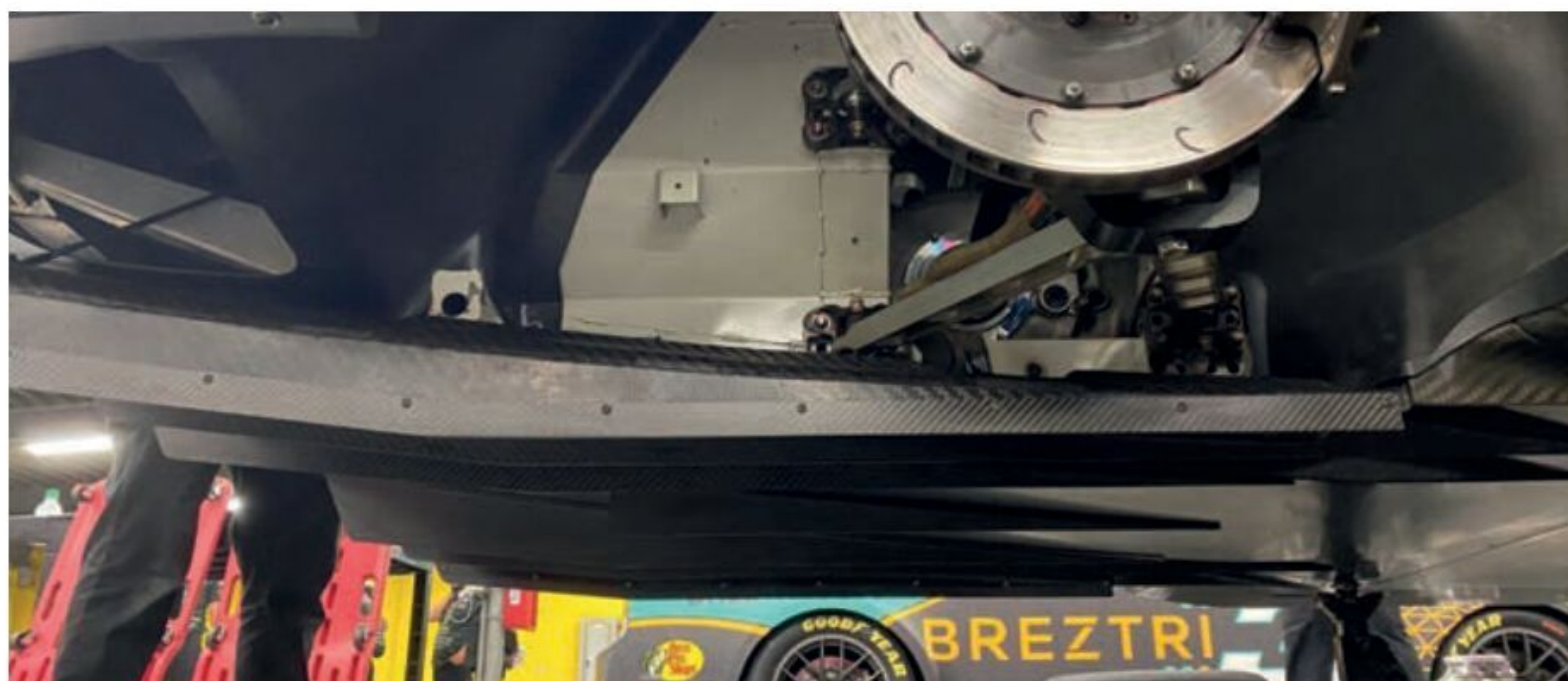
Fig 10: Extended carbon skirts on the outer walls of the diffuser tunnel also re-captured some of the lost downforce
