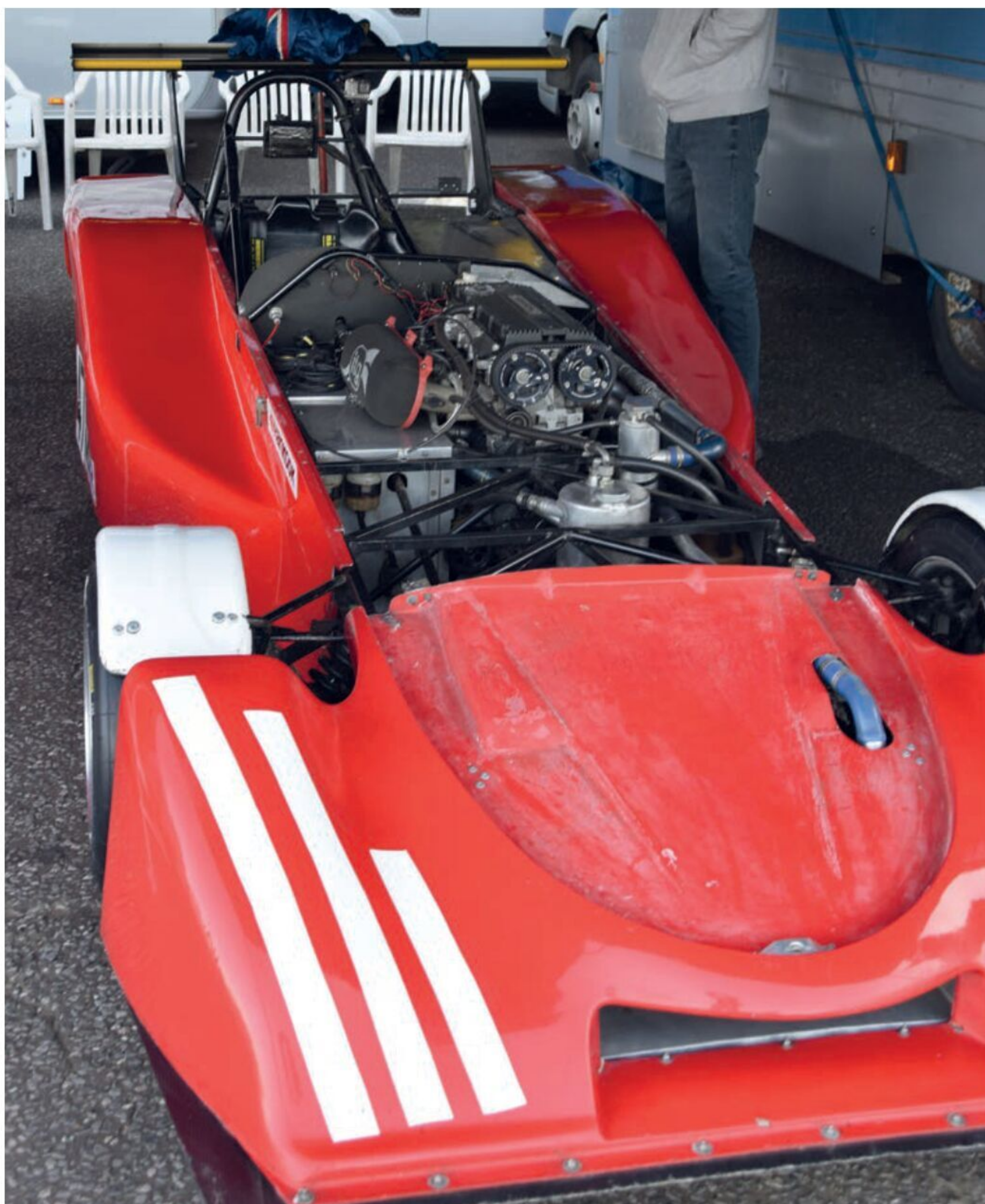
The 1.8-litre Rover K Series in Peter Richings's Mallock Mk30PR. Note that although the engine is ahead of the driver, it's also positioned close to the centre of the chassis, with the driver sitting over the rear axle
