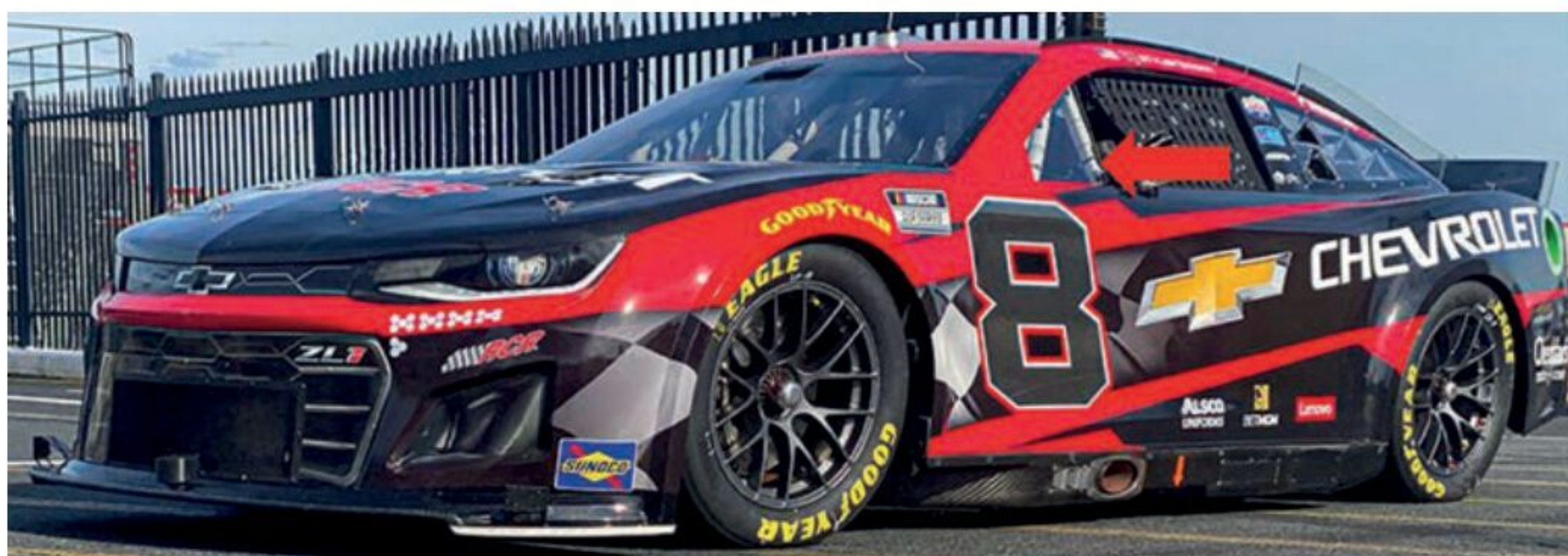
Fig 5: A-post window deflector (arrowed) replaced the previous NACA duct and reduced cabin temperatures by 18-27degC
