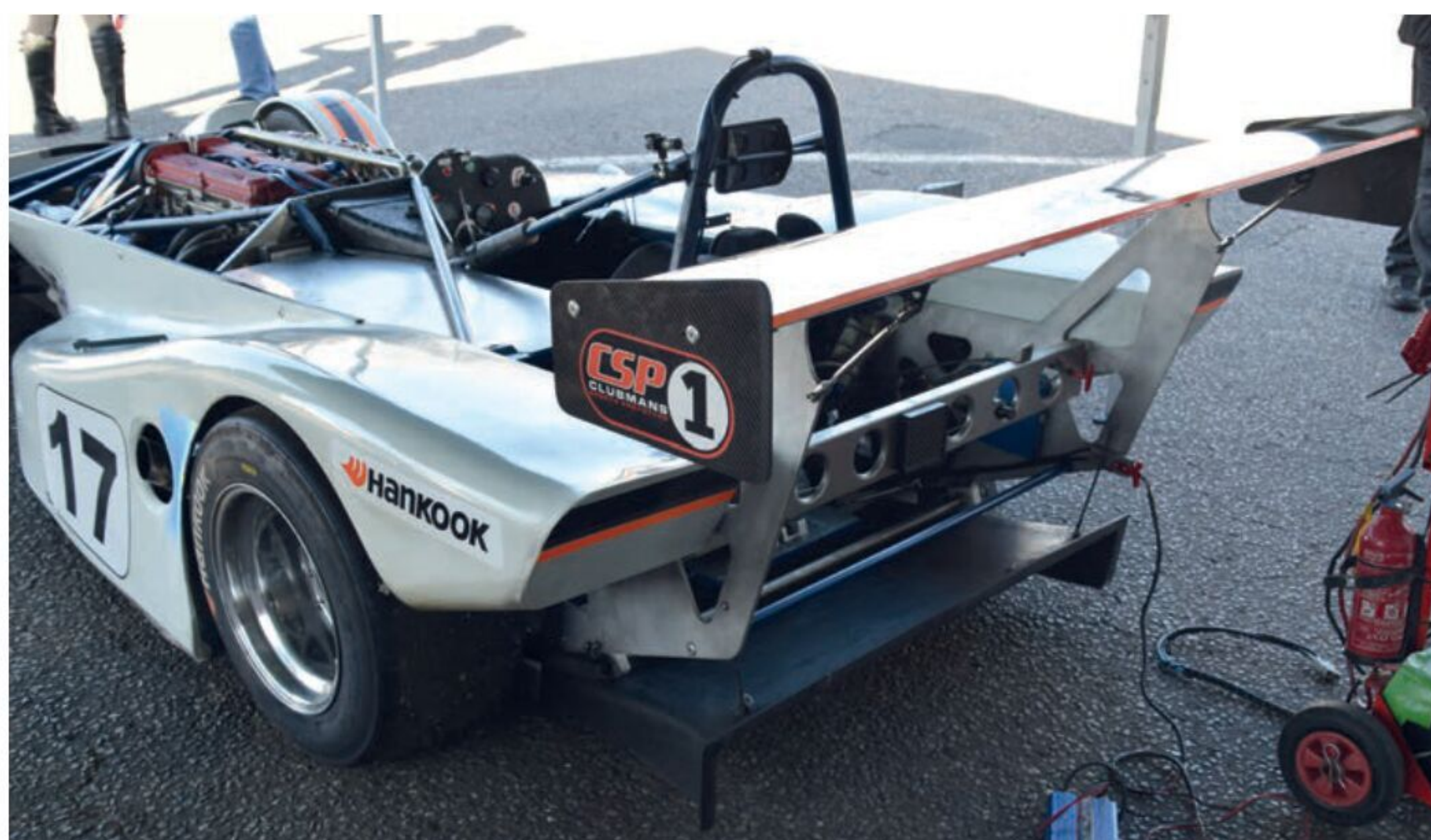
Most of the CSP1 cars feature flat floors, large rear diffusers, big rear wings and quite high downforce levels. Note the typical rear-biased driving position, more akin to a dragster than a circuit car, one of the signature elements of the Clubmans series
