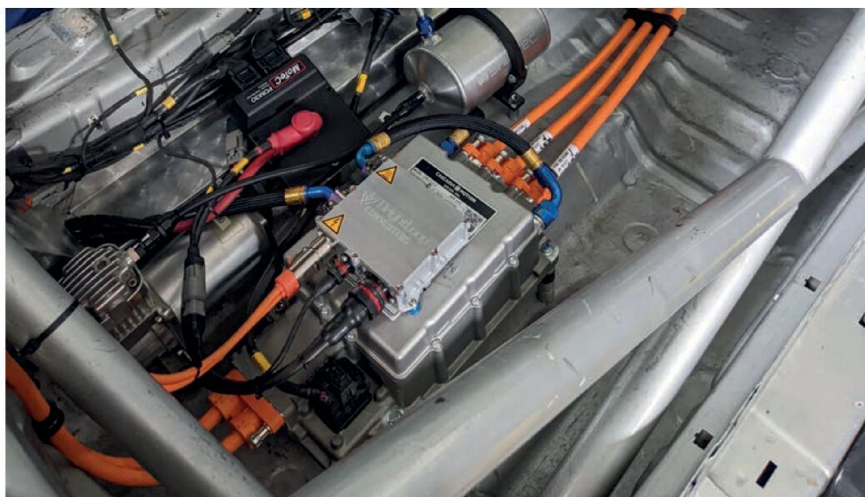
An inverter, DC DC converter and power distribution module mounted inside a hybrid Time Attack car
