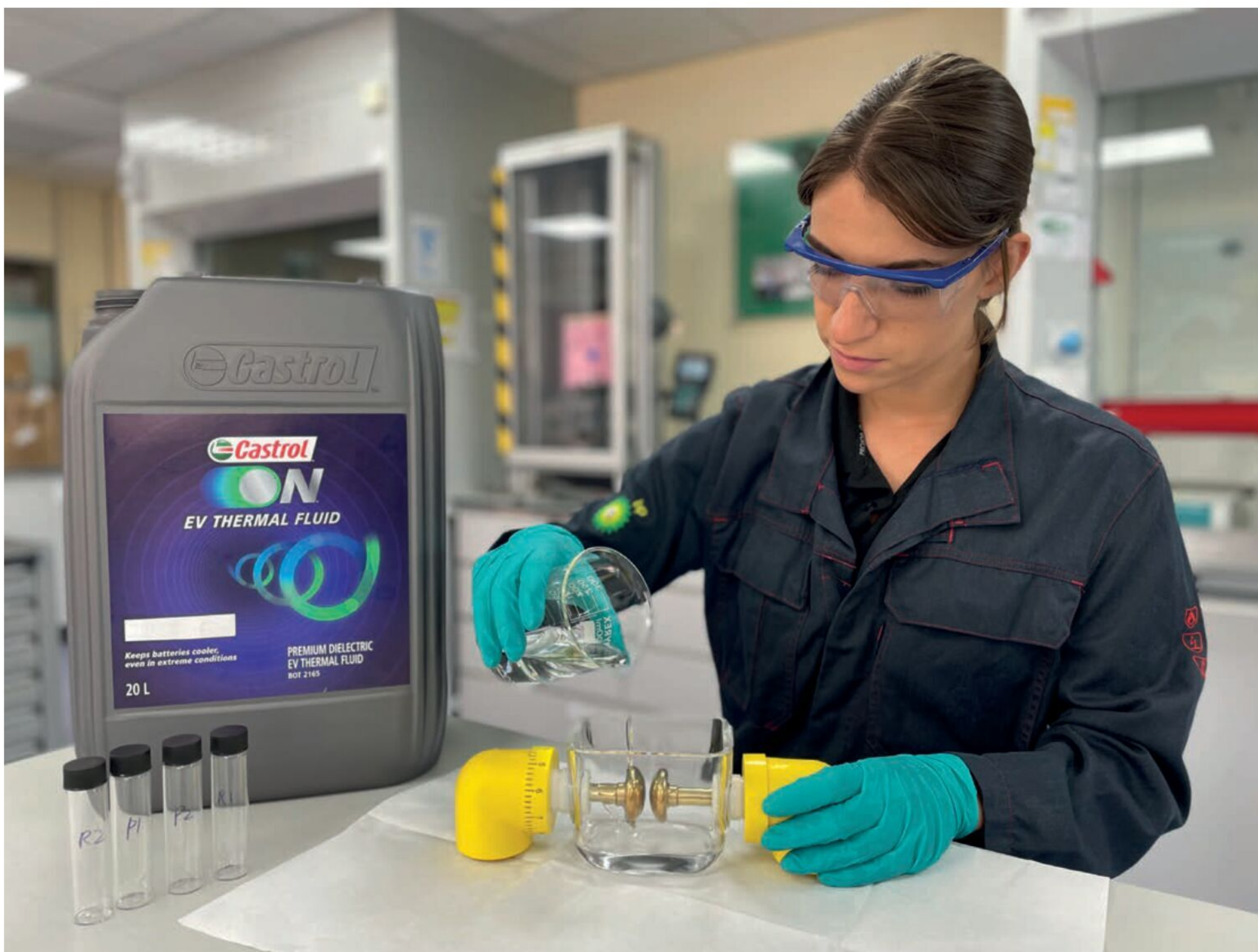
Meanwhile, engineers at Castrol, the lubricant and coolant arm of British Petroleum (BP), are working on the development of suitable immersion cooling fluids for use in EV applications
