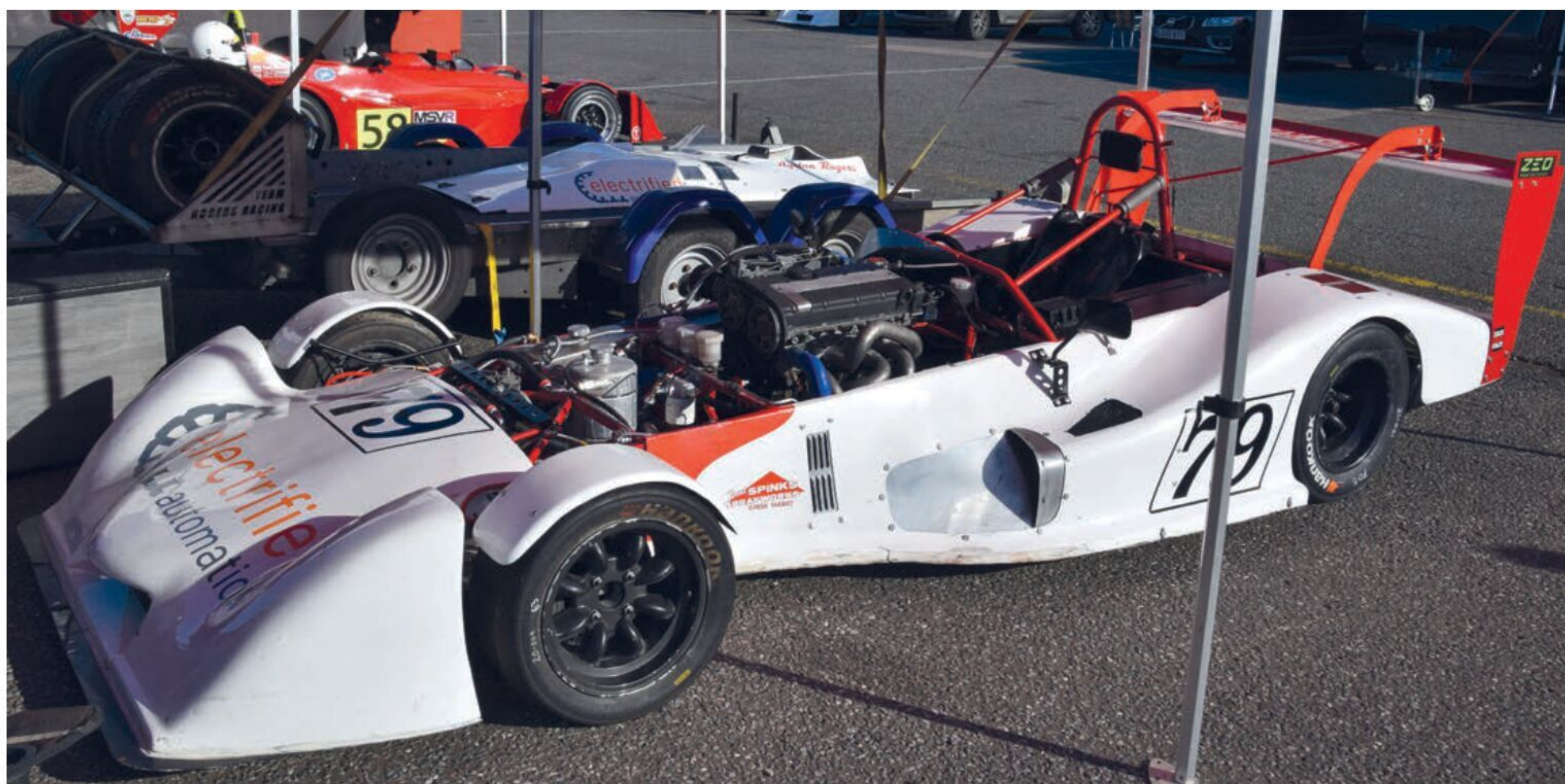
Ayrton Rogers developed his Mallock Mk27 with straight-line speed in mind, while it also features a swan-neck rear wing. With the engine cover off, the car's Vauxhall 16v powerplant is visible
