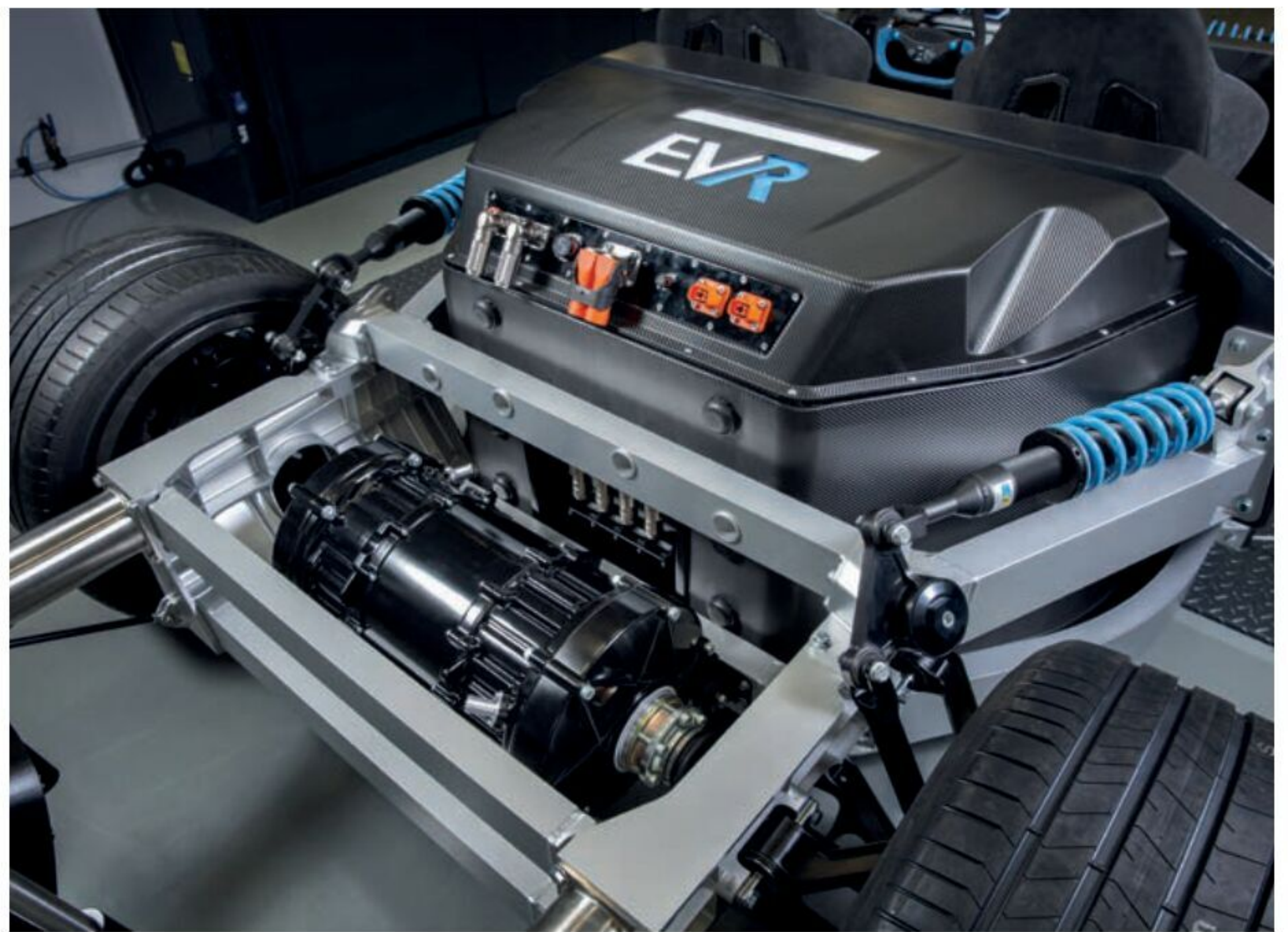
Williams Advanced Engineering recently launched its EVR, which focuses on the growing electric hypercar sector, with a lightweight composite structure and a high performance battery system
