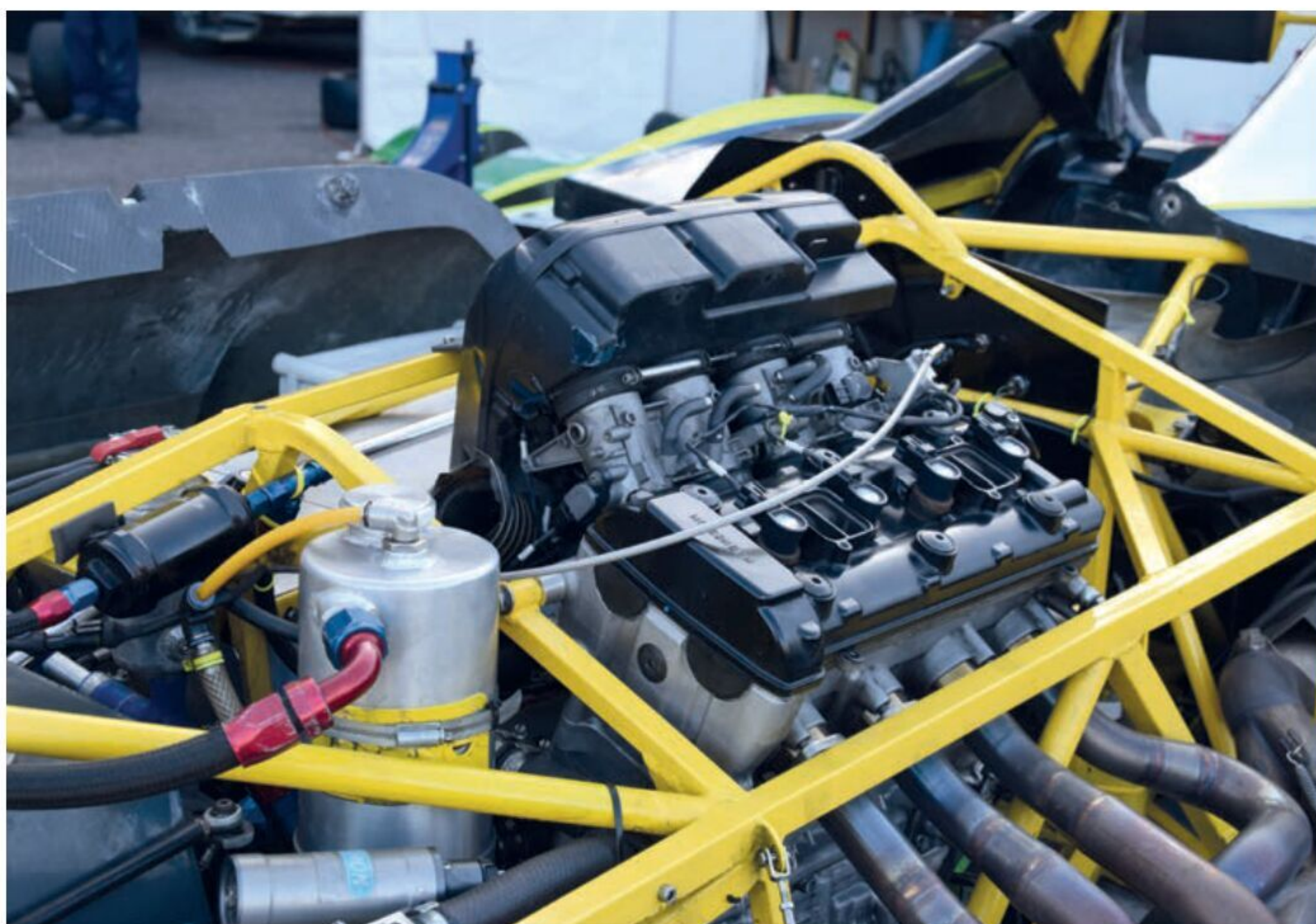
Motorcycle engines are allowed, but they are restricted to 1600cc. This is the 1510cc Hayabusa unit in Adrian Lester's Clubman 35
