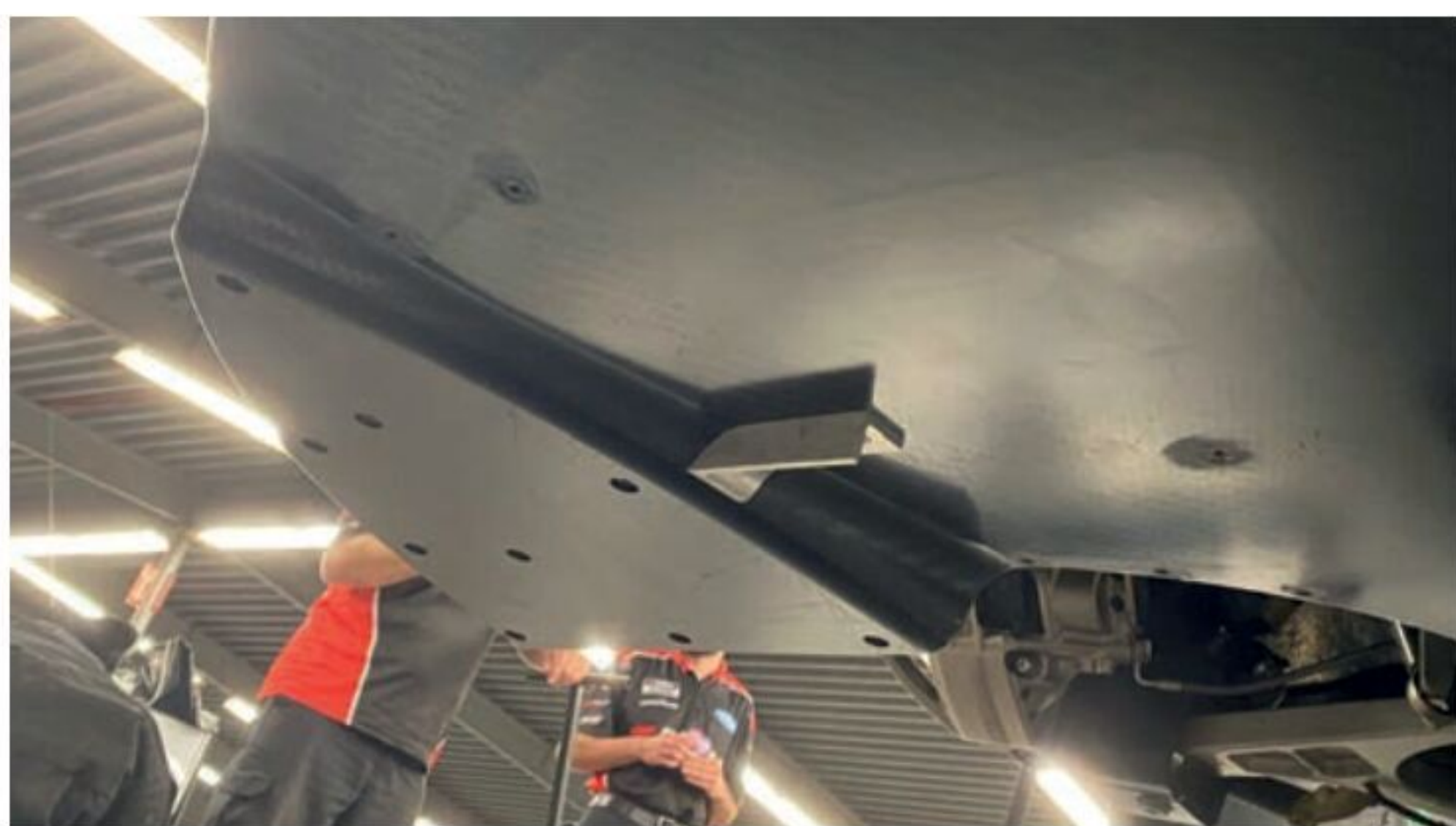
Fig 8: So-called splitter stuffers helped flatten the lift coefficient vs ride height for the car
