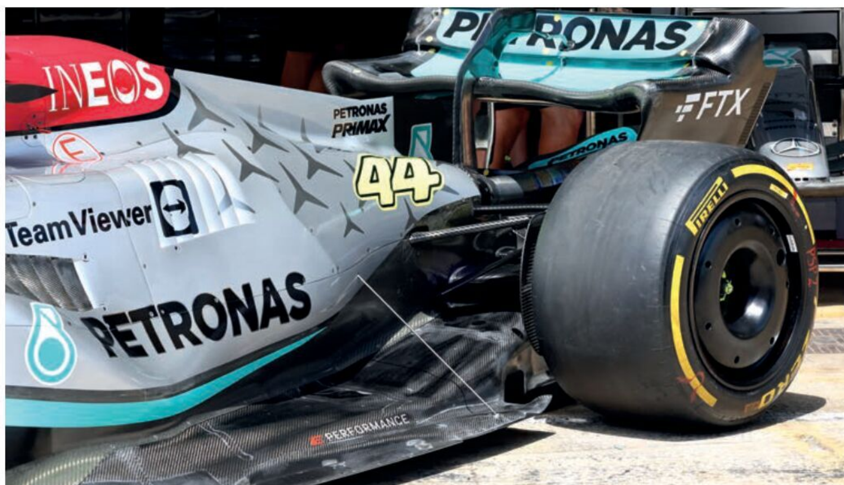
The W13 floor has an exit flow condition positioned midway down. This rejects airflow under the car that isn't in the tunnel flow. Slots further back on the floor edge re-ingest some of the exit flow to work the diffuser and control rear tyre jets
