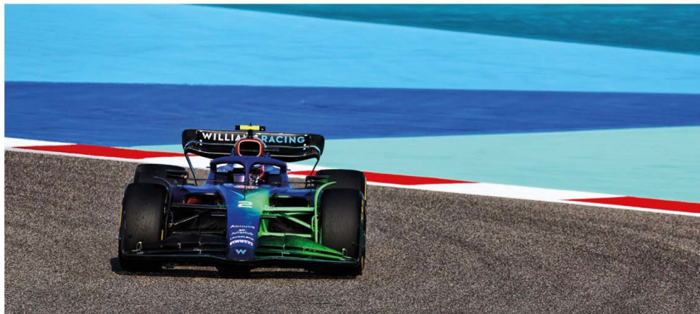
To establish a valid aeromap, you need to consider other dependencies such as speed, side slip, steering angle and roll, as well as the interaction of the front and rear ride heights of your car
