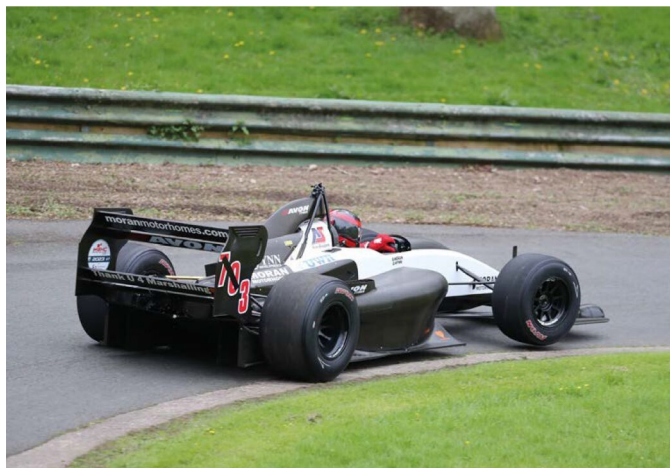
More torque in the V8s means less gear changing, an advantage on the hills. Pictured is Scott Moran's Gould GR59 with 4.0-litre Judd
