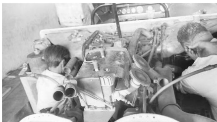
After it suffered from vapour lock, Chaparral engine man, Gary Knutson, equipped the JLO auxiliary engine with fuel injection and capacitive discharge ignition to enhance its reliability. Even then, the driver had to constantly monitor its cylinder head temperature and adjust the mixture accordingly, whilst driving flat out!
