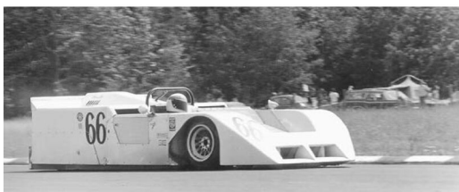
As much for its potential as for its performance, the 2J had rivals reaching for the rule books. After only a few races, it was concluded that both the rotating fans and the skirt contravened the no moveable aerodynamic parts regulation and, by the end of its first season, the 2J was banned
