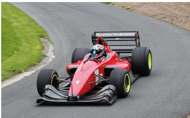
Reigning BHC champion, Wallace Menzies, runs a normally aspirated, 3.3-litre Cosworth XD in his Gould GR59, which gives out close to 700bhp. Note the pitot tube at the front, just one of dozens of sensors on this heavily datalogged car
