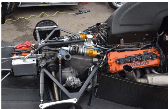
Dave Uren's Gould GR55 runs with a normally aspirated Cosworth XB, a unit originally designed for use in IndyCar. This engine is becoming rare now, so others use the later XD version
