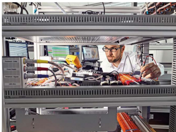
Hardware-in-the-loop simulation (HILS) integrates physical components of the racecar into the process
