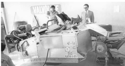
Stripped of its front and rear body sections, the 2J reveals its deep central aluminium monocoque structure. The hinged 'doors' met the letter of the Can-Am regulations. Standing behind the car in sunglasses is Cameron Argetsinger, who had joined Chaparral Cars as a vice president in 1970
