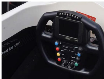
Driver aids such as launch and traction control are crucial, and usually both can be controlled from the steering wheel. Note subtle sports psychology on the left of Alex Summers' cockpit
