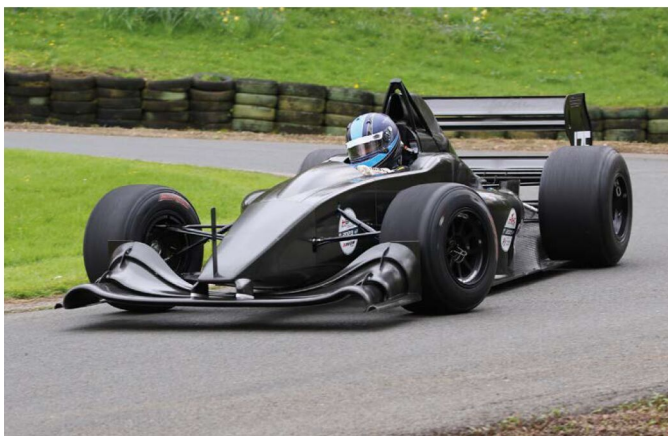
BHC front runner, William Hall's Gould GR59, packs a 4.0-litre Judd V8. These engines were originally designed for high-end sports car racing and are ultra reliable, as well as making tremendous amounts of torque
