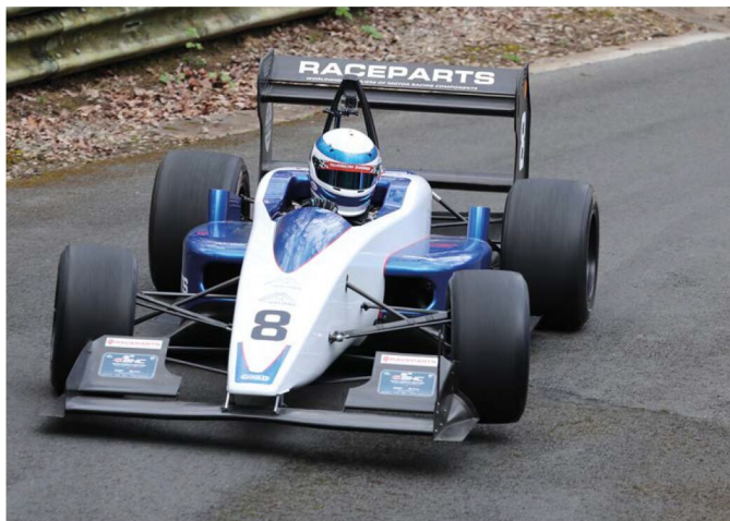
Paul Haines has a 1300cc turbo Hayabusa engine in his 320kg Gould GR59. It makes 460bhp and he's often in the mix with the V8s
