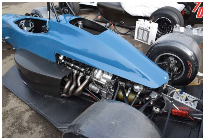
The RPE V8 in Trevor Willis' OMS 28 was developed for the Radical SR8 and is essentially two Suzuki Hayabusa motorcycle engines working off a shared crank. This engine is said to give out around 480bhp
