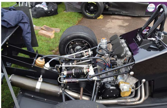
Suzuki Hayabusa motorbike engines are a common choice in the British Hillclimb Championship. This example has been stretched from the standard 1300cc to 1.6-litres and is fitted into a Force PT chassis
