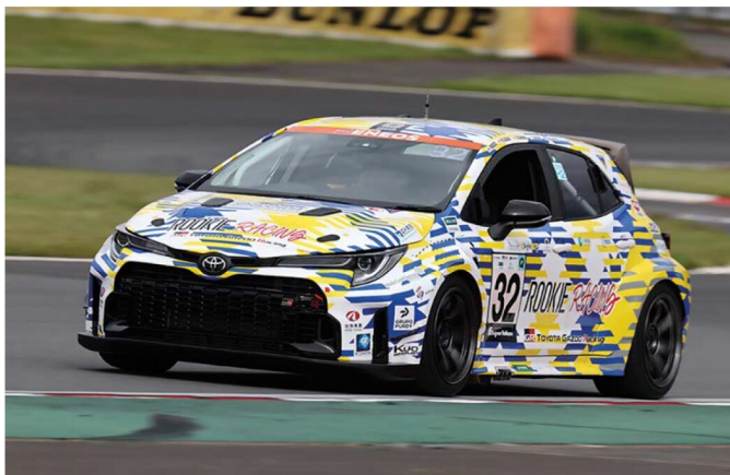
Toyota competed in the Super Taikyu series in Japan with a Corolla using liquid hydrogen storage. The ACO considers this technology not mature enough at this stage for racing at Le Mans, given that liquid hydrogen needs to be stored below -250degC
