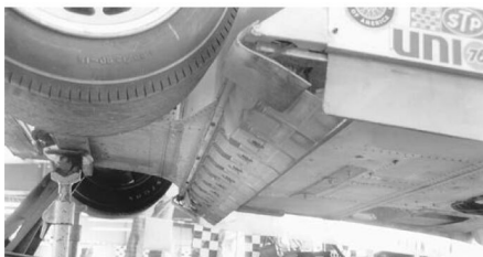
Providing the vital seal at the front of the suction area was a transverse row of a dozen Lexan pieces. Designed by Chevrolet's Don Gates, each comprised an individual system, with a hinge to the body, and each was backed up by two more Lexan parts, hinged to harness both spring and vacuum force to keep its trailing edge on the track
