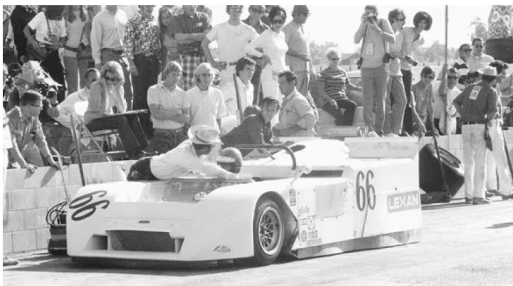
Jim Hall leans across Vic Elford into the cockpit of the 2J at Riverside in the car's last race appearance. Although unsuccessful as a racecar, the 2J made history as the first automobile capable of generating so much suction downforce that it could be driven on a ceiling
