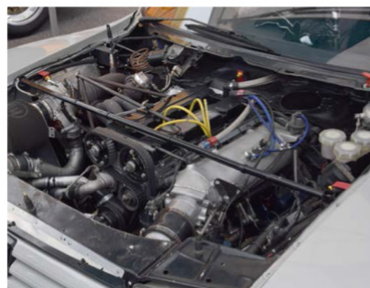
The 309 features a Cosworth YB engine that gives 600bhp, while drive is now via the rear wheels and its suspension is based around Tiga Group C2 uprights
