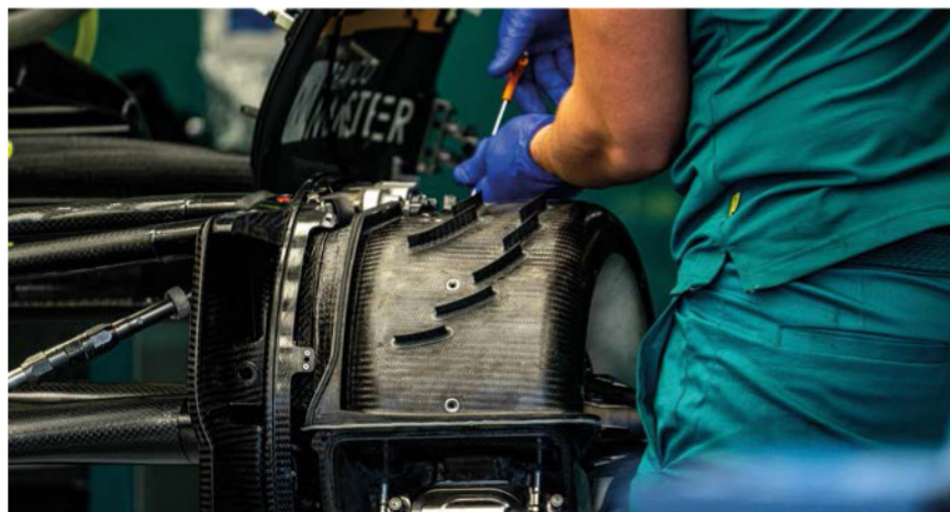
Aston Martin has been using these small vanes on its rear brake drums to try and gain an aerodynamic advantage
