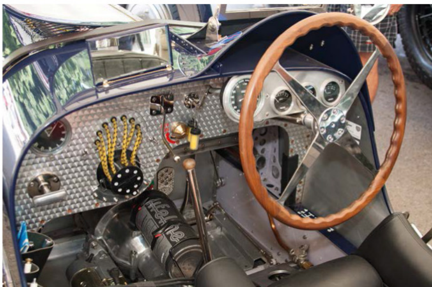
Scintilla magneto was mounted in the dash and shaft driven from one of the camshafts. It triggered a single plug ignition system with the plugs mounted vertically in the engine valley. The second camshaft drove the rev counter
