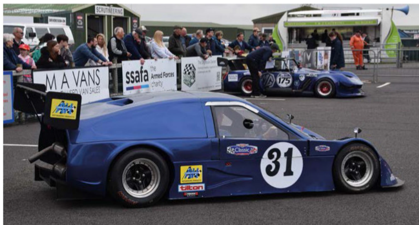
It might look like a little bit like a Honda CRX, but there's not much Honda in Thomas Carey's racecar. The car's unusual semi-spaceframe monocoque chassis started life as a Royale Sports 2000
