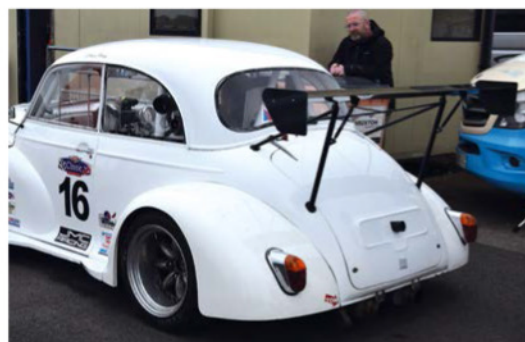
Craig Percy's 1967 Morris Minor started life as a police car, but now packs a 6.3-litre small block Chevy engine producing 430bhp
