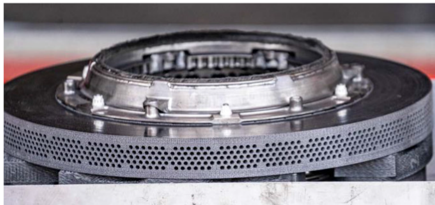
From 2022, the complex internal drillings made into Formula 1 carbon discs must be a minimum of 3mm in diameter
