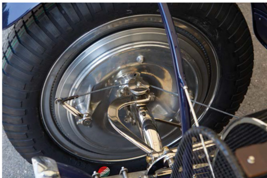
Front end continued the Bugatti trend of a hollow, two-piece front axle with semi-elliptic leaf springs, though new for the Type 59 were complex and exotic Hydraulic de Ram shock absorbers, mounted inboard of the chassis rails
