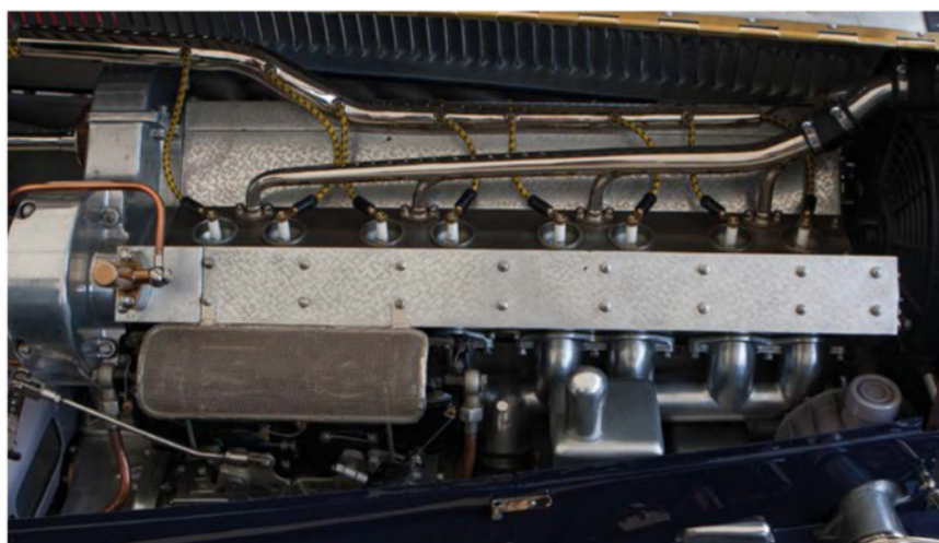
The displacement of the Type 59's straight-eight, DOHC engine was initially 2821cc, and it used plain bearings for the crank and dry sump oiling system, where its predecessors had utilised roller bearings, and a Roots-style supercharger
