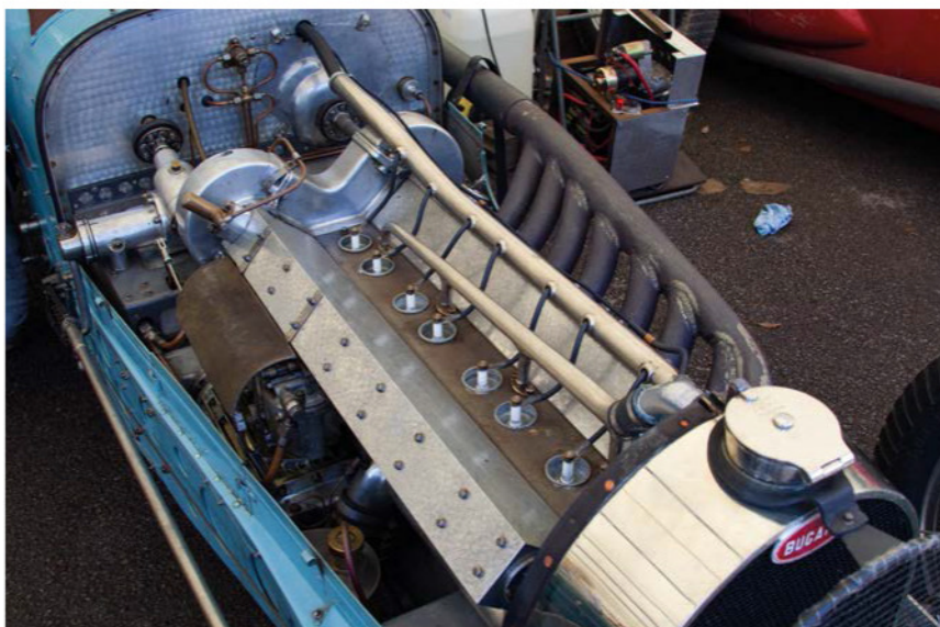
Ettore Bugatti persevered for several years with his SOHC straight-eight engine but, after buying and closely inspecting two American-made Miller racecars in 1929, he relented and changed to a double overhead cam design
