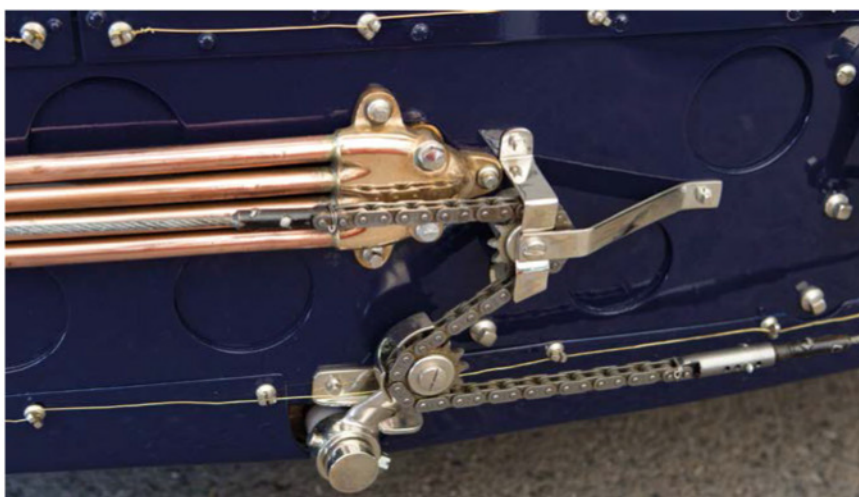
Front and rear mechanical brakes were connected by this external chain drive, while the four copper pipes are a rudimentary oil cooler that relied on the passage of air over them to effect a change in temperature of the fluid within
