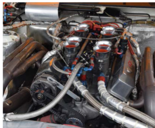
At the time these pictures were taken, the Carlton TS6000 had this cast iron block, 600bhp, 5.7-litre Chevy V8 fitted, but an aluminium alloy version of 6.0-litres is set to take its place
