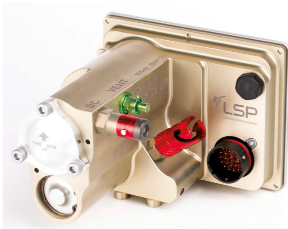
The latest BBW systems, such as this IBSe from LSP, offer additional functionality, such as launch control and adjustable brake bias
