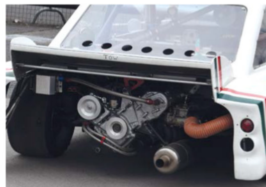
With the engine position at the rear, Imps were a perfect base for silhouette racers based on Sports Prototypes. Burgoyne's car uses a highly tuned, 1040cc Hillman four-cylinder engine
