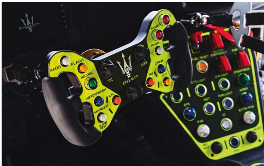
Switchgear in the cosy cockpit is targeted at the customer driver, with colour coding and a high-mounted set up
