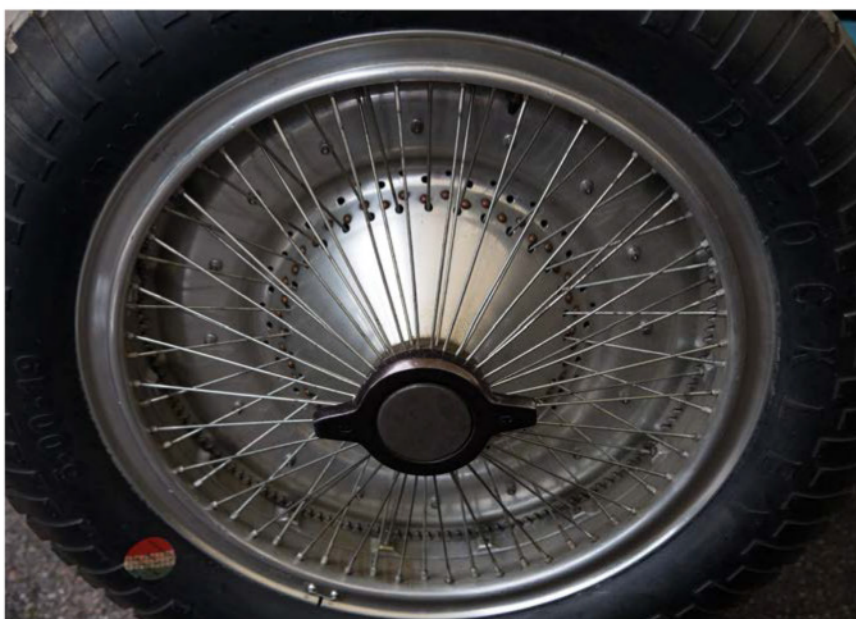
One of the distinguishing features of a Type 59 is its wire wheels, with the brake drums an integral part of the design
