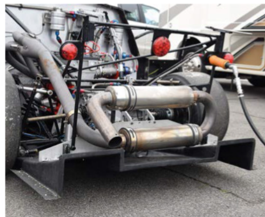
The CRX usually races with a 2.0-litre Cosworth BDG powerplant, but at this event was running with a 1760cc BDA. The diffuser is among a number of aerodynamic improvements made to the car
