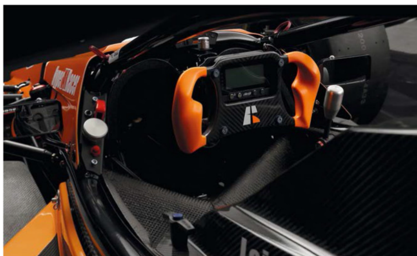
Bespoke steering wheel incorporates specially designed grips for improved ergonomics. Gear selection for the six-speed sequential ‘box is via a deliberately ‘old school’ lever. This car is all about the driving experience
