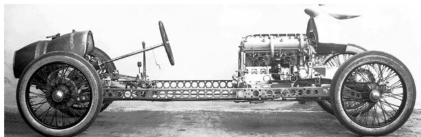
Extreme drilling of frame side members, and just about every other conceivable part, suggests flexibility, but apparently that was not considered deleterious to the Benz RH's handling qualities
