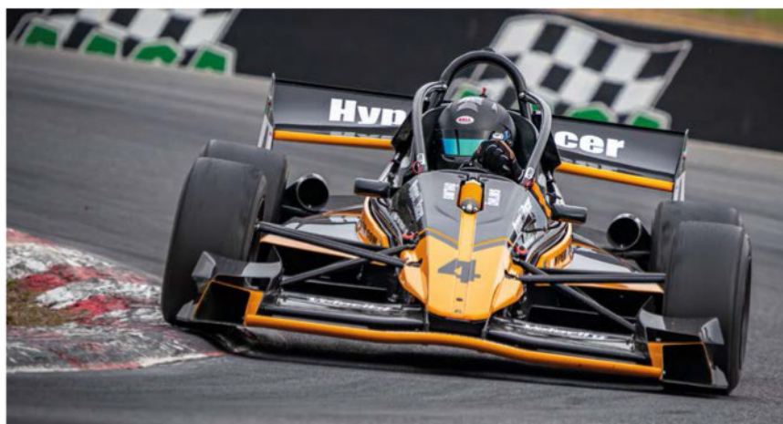
The X1 is extremely quick through the corners, with the spec aero package generating around 600kg of downforce. The car's large, single-plane rear wing helps balance out the powerful ground-effect floor
