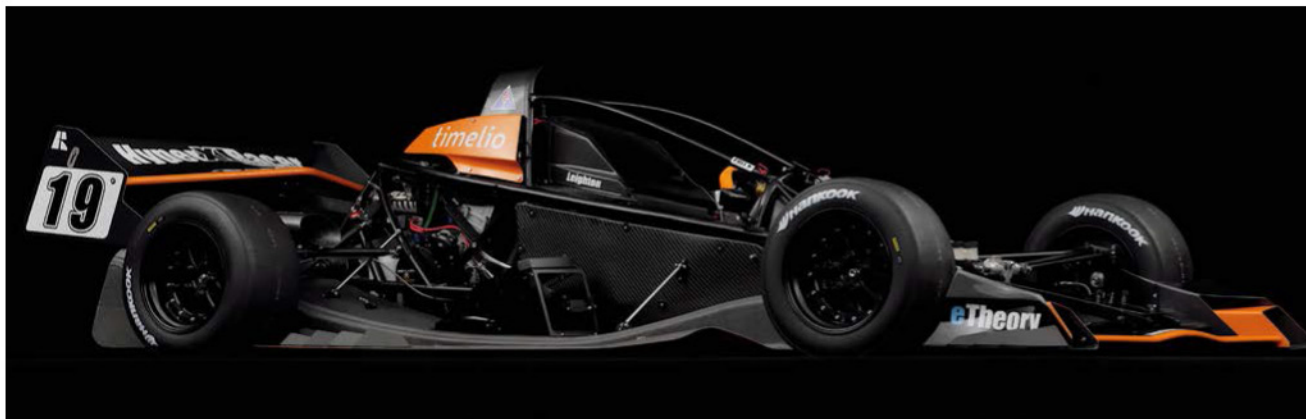
The FIA-spec Diolin side impact panels are visible here, as is the dramatically-shaped floor. Note the graceful 'Henry bars', an unusually attractive answer to cockpit protection
