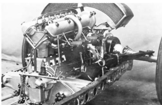
Installed engine image shows the linkages of the throttle and other controls. Coolant is fed directly from the water pump to the radically-shaped radiator and streamlined header tank
