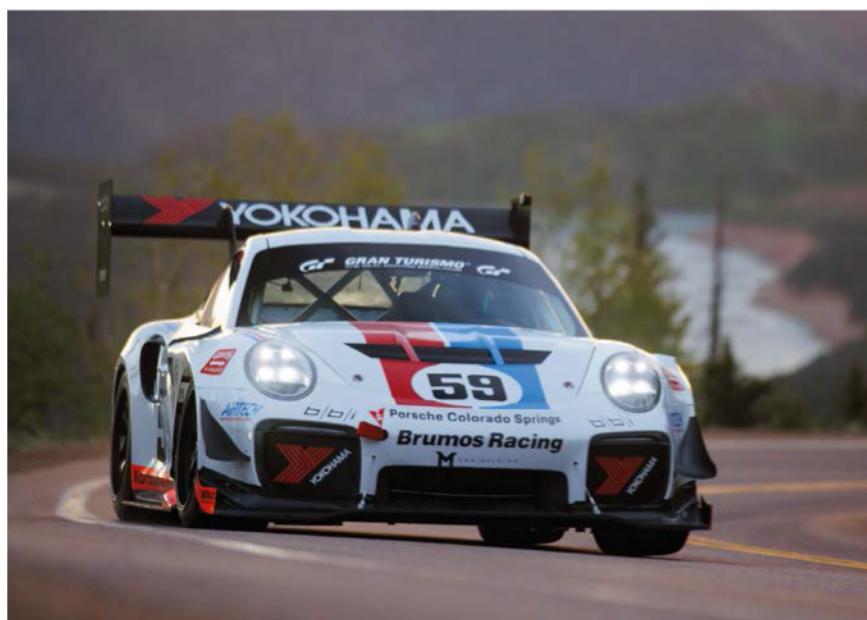
Changing from three radiators to one at the front enabled the team to re-purpose the bumper inlets into splitter tunnels
