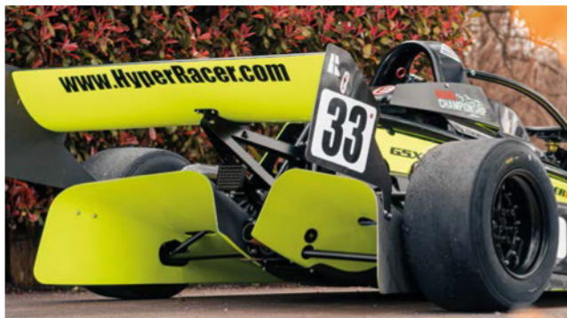
Tunnel exits and large wing and end plates seen from the rear of the X1. Hankook Formula 3 tyres have proved to be very durable, partly thanks to the car's light weight
