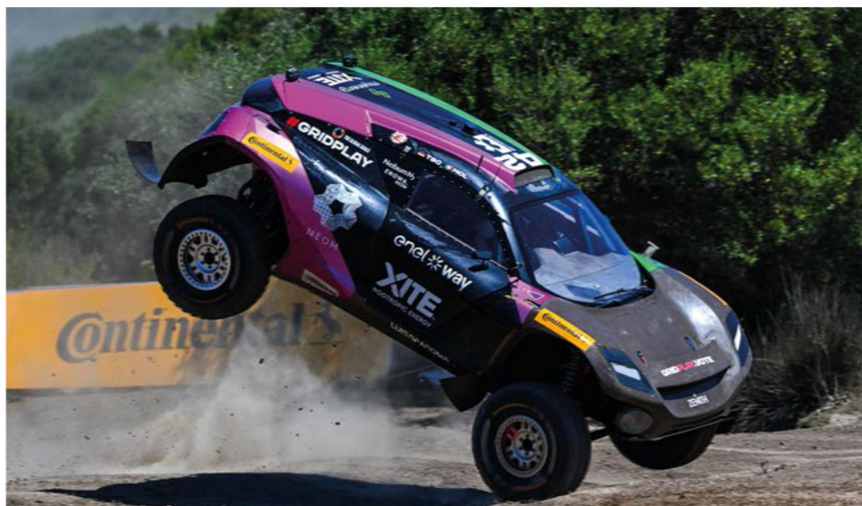
Sardinia 2022 was the first race for the new Fox dual suspension system that increased wheel travel and gave a more predictable ride
