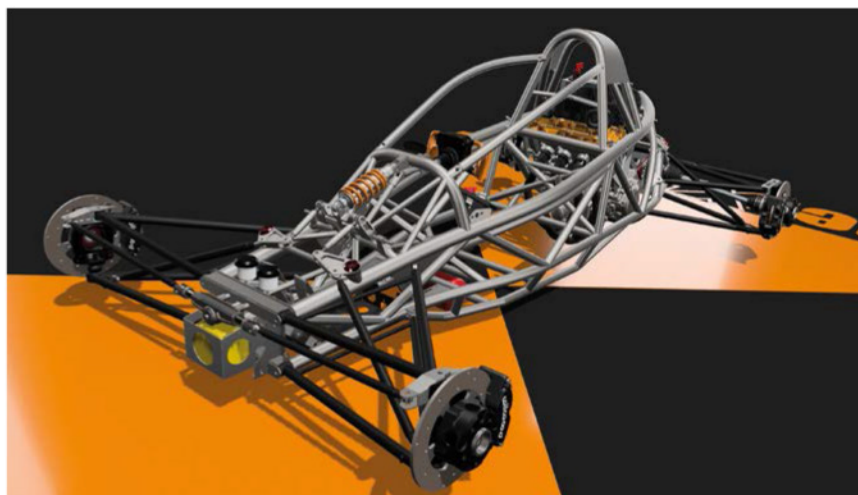
The X1's spaceframe is constructed from 4130 chromoly steel with curved main rails and a plethora of cross braces
