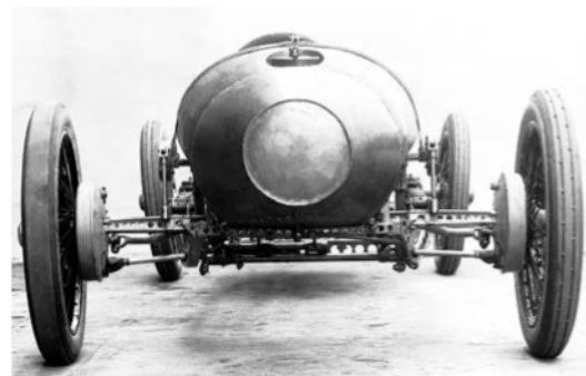
Front mechanical brakes of the RH Benz are well exposed for cooling, while damping at the front is by rotary friction drums
