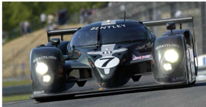
The flat-bottom cars exhibited low pressure areas front and rear, and Peter Elleray's 2003 Le Mans-winning Bentley increased the size of these areas to improve its 'operating window'
