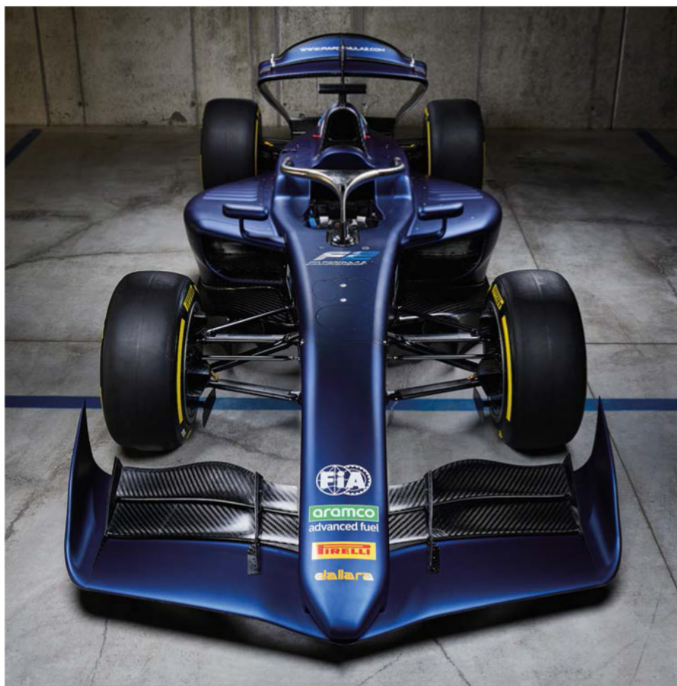
The new car's aero has been designed to promote close racing, while safety advances include the Halo now being a structural part
