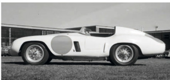
Tilp's 750 Monza displayed a new design of side scoop for rear brake cooling, and smaller rear tyres than were used on the first such car
