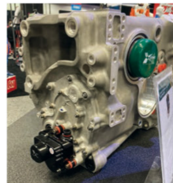
Xtrac's new electronic gearbox actuator, as used in the NASCAR Garage 56 entry at Le Mans
