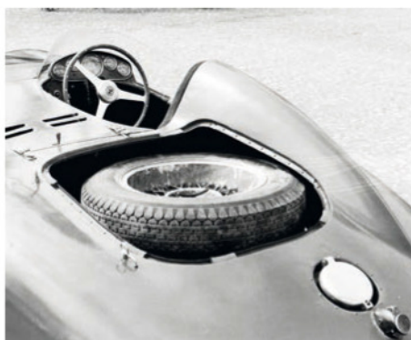
Room was saved above the 750 Monza's fuel tank for its mandatory spare wheel. Tyres are, naturally, Pirelli Corsa
