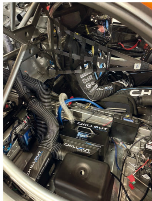
Example of how a shirt or helmet cooler can be fitted in a GT car's cockpit. Weight and space factors are important considerations
