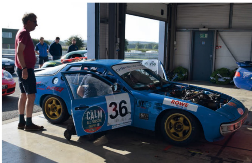
How the seat is fitted, and the quality of welds on a roll cage will be carefully examined, particularly if it's a selective scrutineering meeting where perhaps only 25 per cent of the cars racing are checked, the others being self-certified
