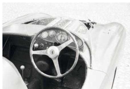
In what had become a Maranello tradition, the 750's instruments were gathered together neatly in an aerodynamic nacelle, easily scanned by a busy driver
