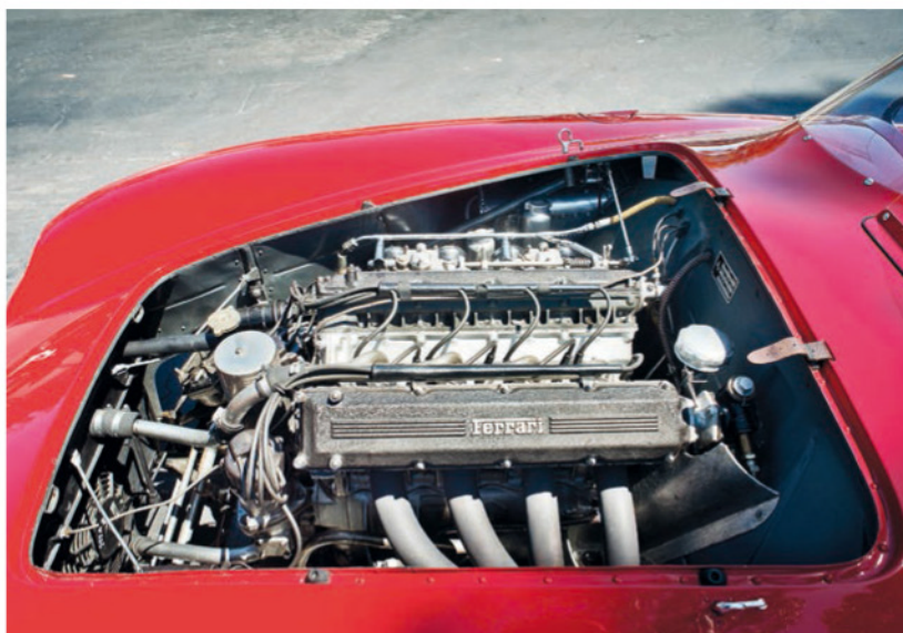
Embedded in its chassis, the Ferrari 750 Monza engine sat well back to provide racecar weight distribution
