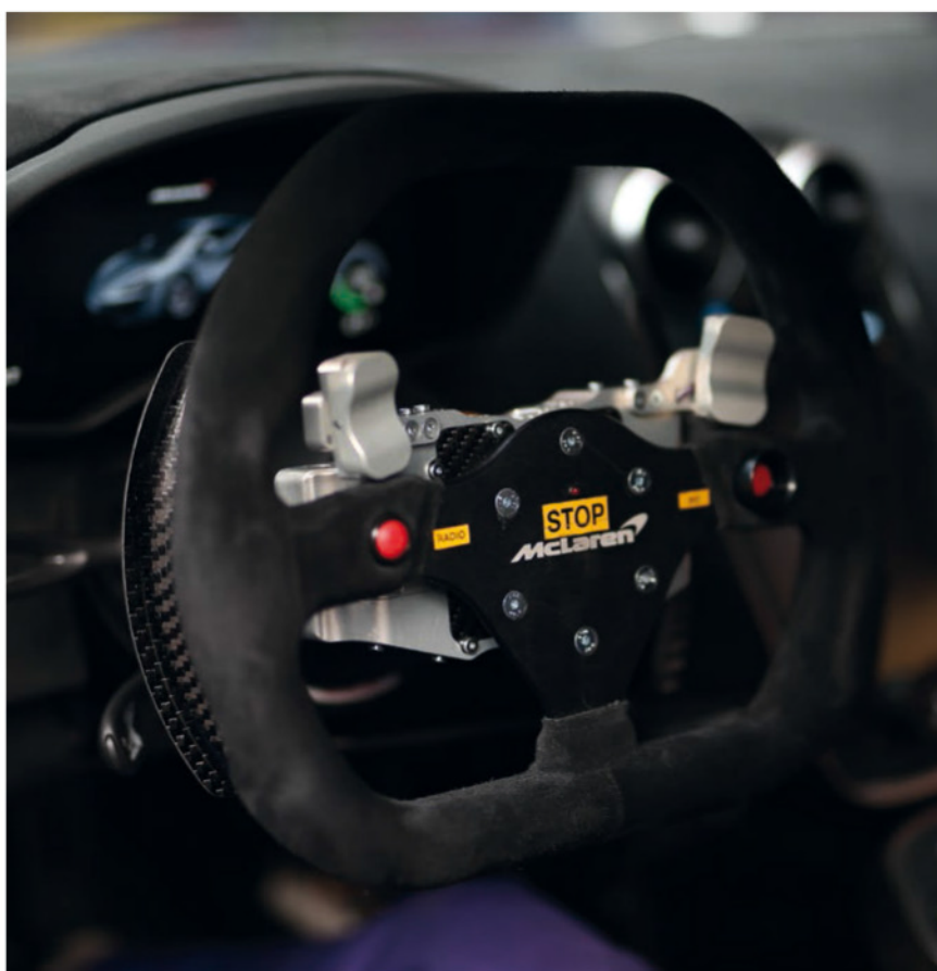
Team Brit's hand control system features paddles for throttle and brake and buttons for gearshift mounted on the wheel
