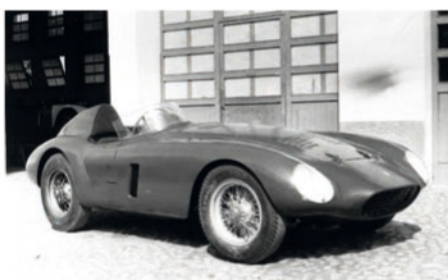
Nominally 6.00 x 16, the rear tyres of this first 750 look larger sectioned – a bold attempt to deliver its higher power output effectively to the road
