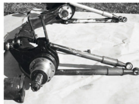
Robust radius rods (which sat parallel when under tension on the car) guided the 750 Monza's de Dion tube, with absorption taken care of by Houdaille rotary dampers
