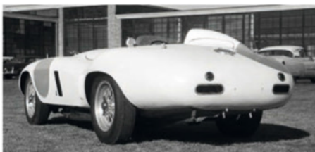
Changes from the 1954 prototype on Tilp's car were twin rear lamps instead of one in the centre and slots for cooling air
