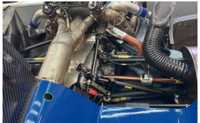
Suspension is double wishbone and torsion bar with integrated brake-by-wire system, carbon discs and a combination of six-piston (front) and four-piston (rear) calipers by Brembo
