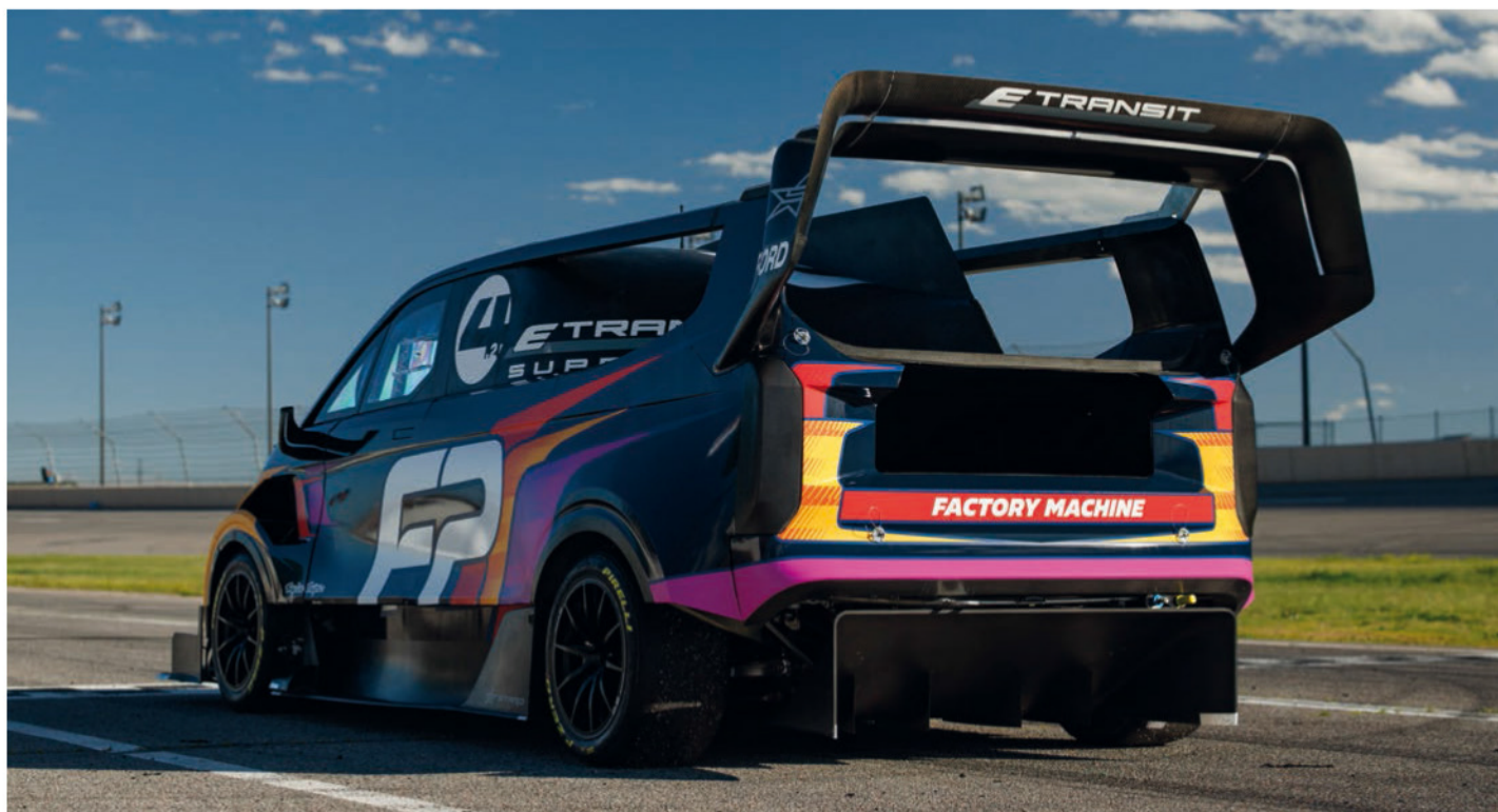
SuperVan 4.2 is the first in a long line of Ford SuperVans to feature an all-carbon fibre body. Aerodynamics have been significantly re-booted from the 4.0 version of 2022 that it is based upon
