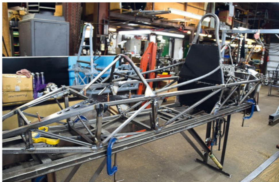
Chassis is of spaceframe construction, making it both strong and cheap to fix. Additional safety measures include anti-intrusion plates
