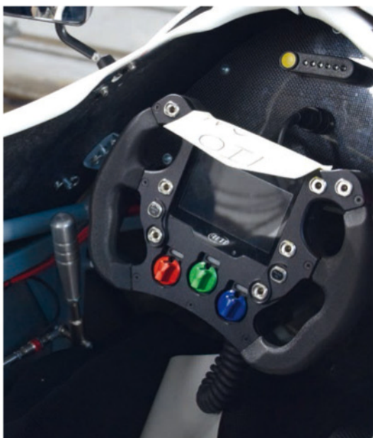
Jedi has resisted the temptation to go with a paddle gear shift mechanism to keep costs down in its one-make championship. The gearbox is a stock Suzuki six-speed sequential
