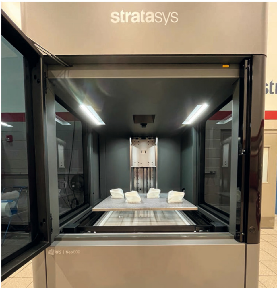
Penske's brake caliper ducts are 3D printed on Stratasys' Neo800 machine
