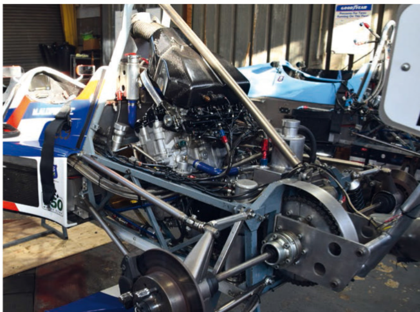
Most Jedis now pack a dry sumped Suzuki GSX-R1000 (K8) motorcycle engine, which produces 170bhp at the wheels
