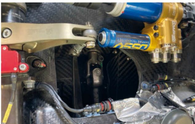
Steering is by way of electric steering rack, while the majority of the control systems onboard come from Bosch Motorsport, including the ECU, VCU and PowerBox
