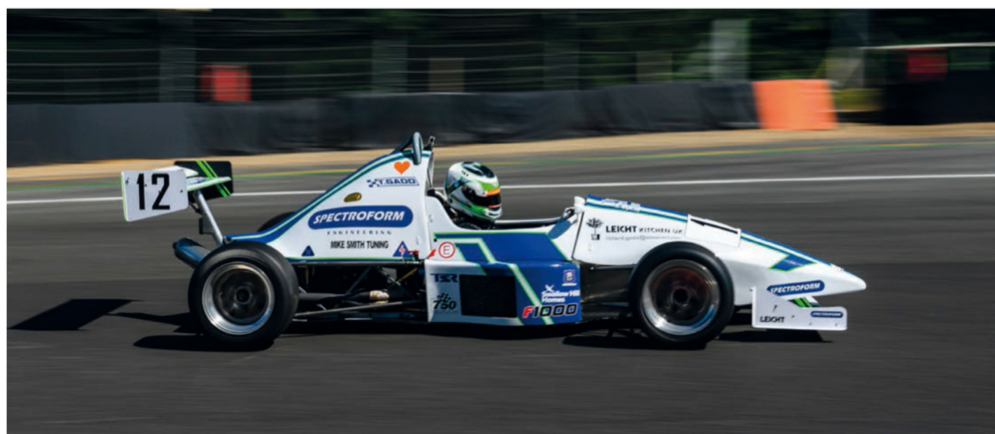
Bodywork is of a modular design and comes in seven separate pieces. This was a consideration right from the start, again to help keep potential (perhaps inevitable) crash damage costs down
