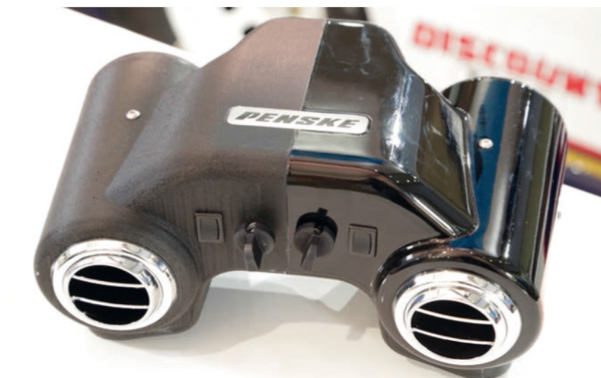
A 3D-printed fan used in IndyCar to cool the driver during practice sessions. The housing is printed in Nylon 12 CF on Stratasys' Fortus 900mc with a comparison between the bare surface finish (left) vs painted (right)
