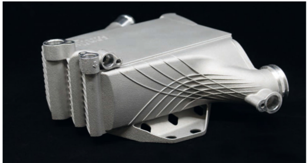
Conflux Technology uses Laser Powder Bed Fusion with metallic particles as small as 0.09mm to make its motorsport heat exchangers
