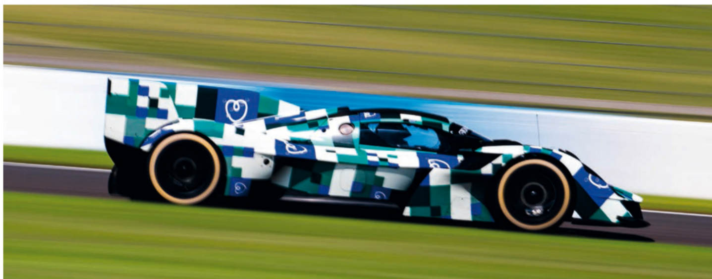
Developed from the impressive, carbon-tubbed Valkyrie AMR Pro, the LMH racing variant features revised aerodynamics and a de-tuned version of the production car's Cosworth V12 engine
