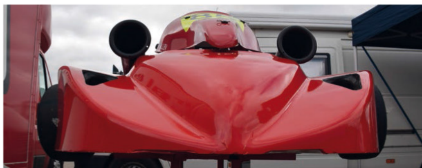
While the adjustable nose is designed with low drag in mind, it’s also a very effective downforce producing device. Note the ram-air snorkels either side of the driver compartment on this twin-engined Jade superkart
