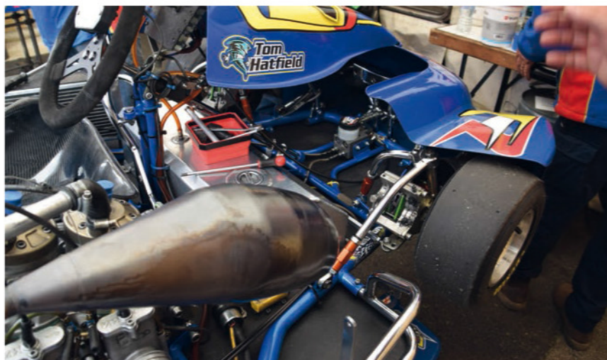
The frame is so much more than a chassis, as it must also provide the ‘give’ that would normally be the work of the suspension on a traditional racecar. Chassis tend to be made from high-grade steels such as T45; carbon is not allowed
