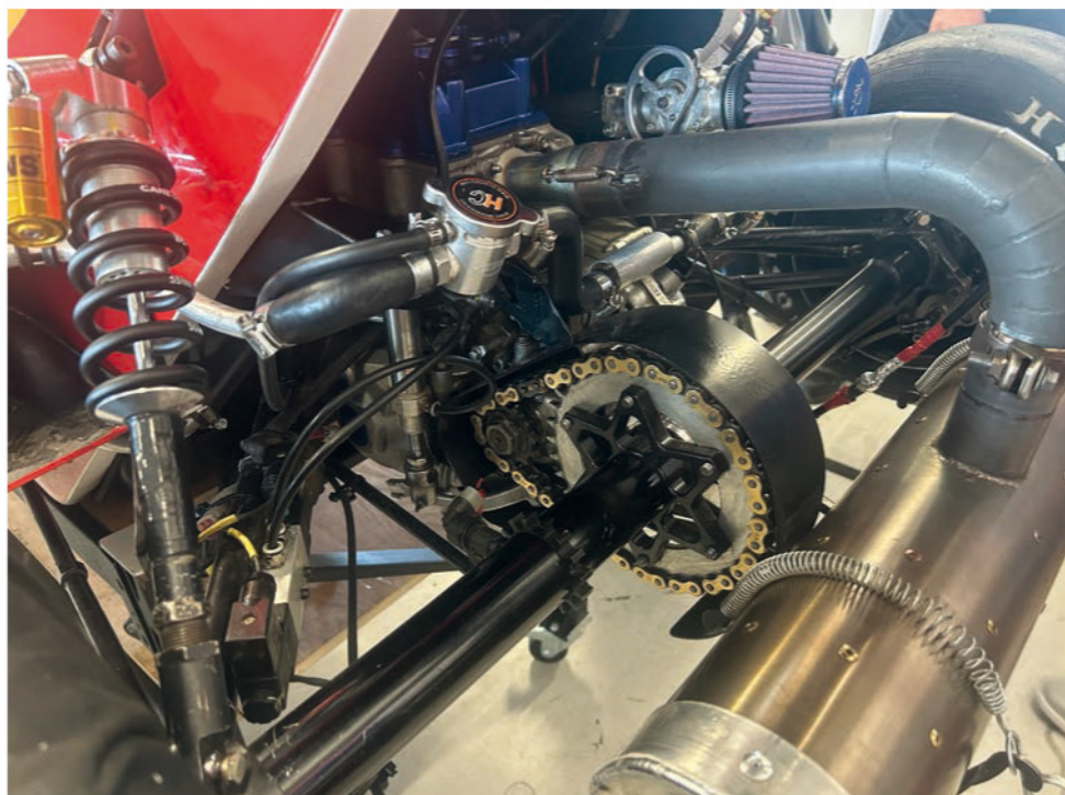
ECU's winning 'Integrated Powertrain Suspension' system had the powertrain connected to the rear axle, not the chassis
