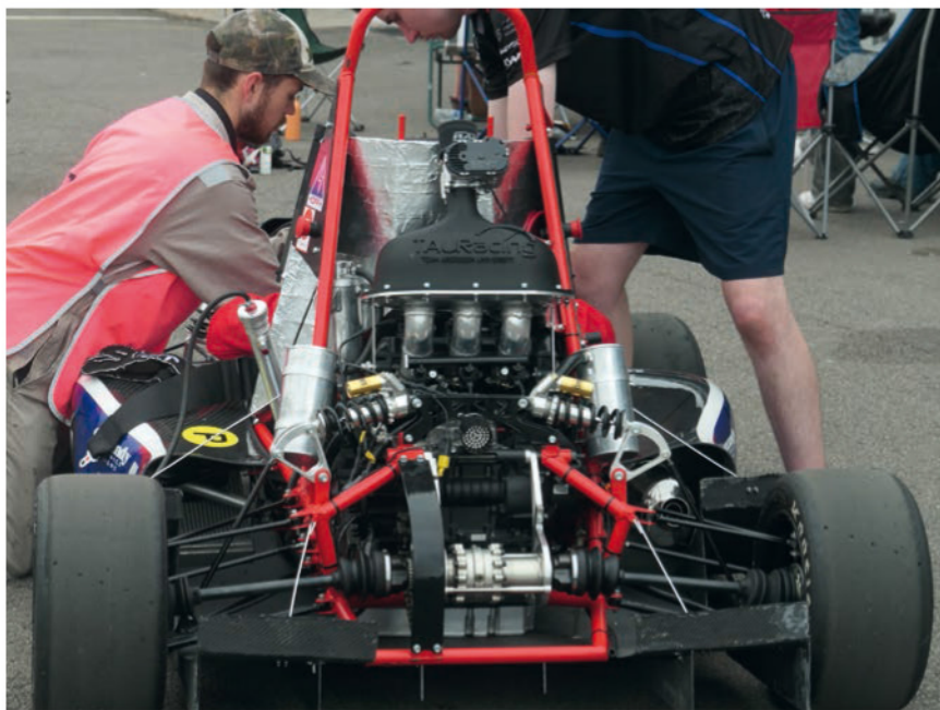
Aberdeen worked its chassis frame around the chain and developed a diffuser, but removed it for the dynamic events
