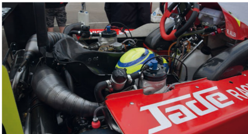
The Jade, on the other hand, uses two 125cc, 50bhp IAME engines, both of which rev to 15,000rpm. This approach means the seat does not need to be offset to counteract a single engine, which helps with chassis balance
