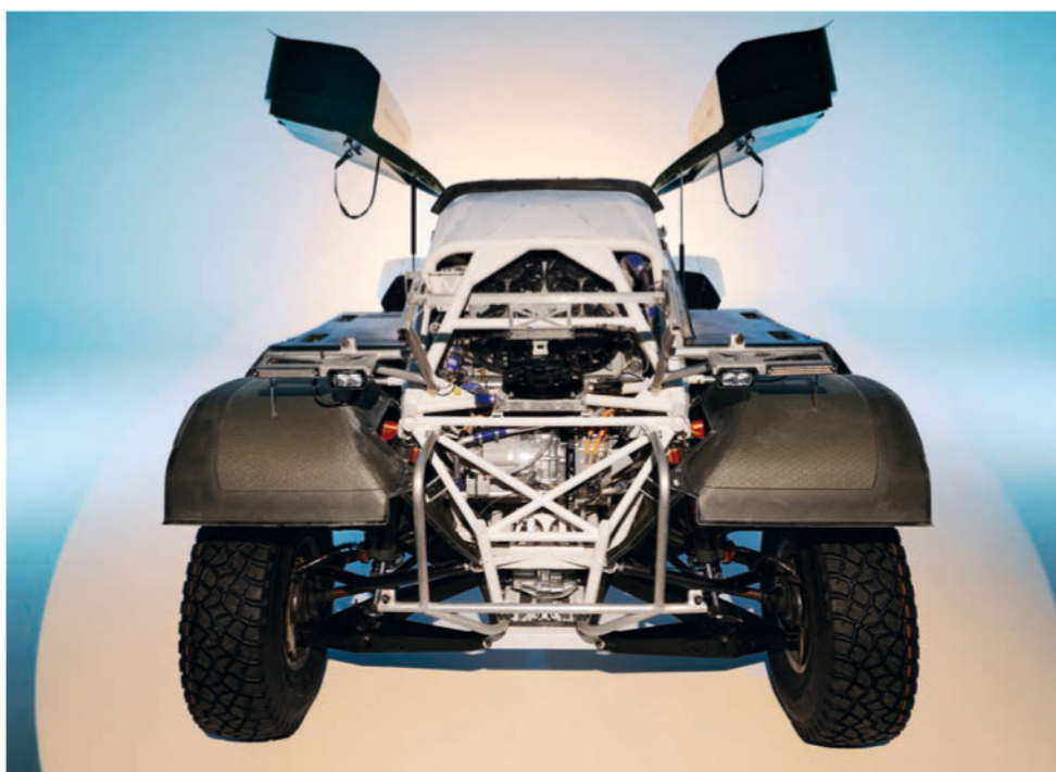
Neatly packaging the hydrogen components has been a priority. The Pioneer 25 is only four per cent longer and wider than Odyssey 21, despite being almost 15 per cent heavier. However, improvements in drivetrain efficiency make it as fast as its electric predecessor
