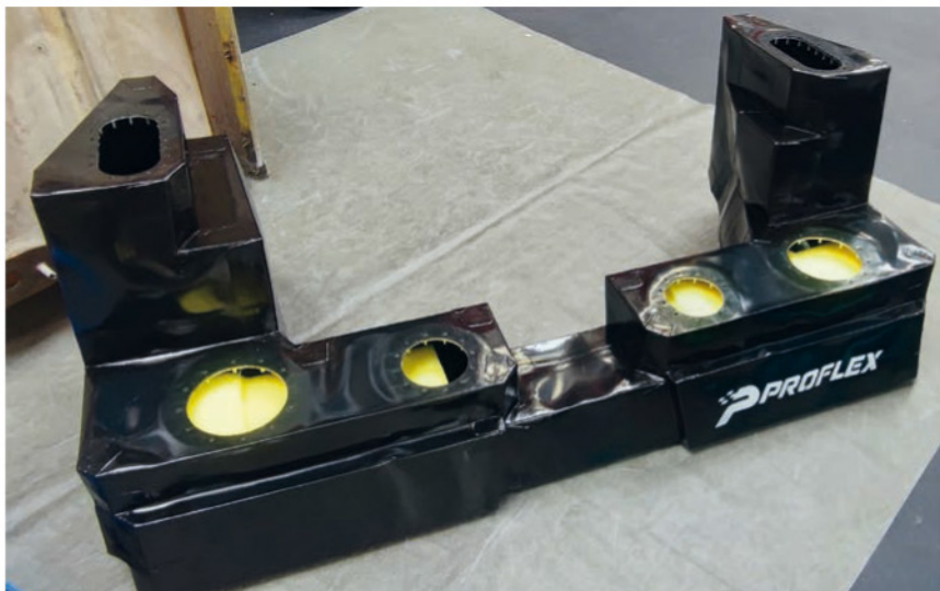
Modern racing fuel cells are largely bespoke items, produced for specific vehicles. This Proflex cell fits an Audi GT3 car
