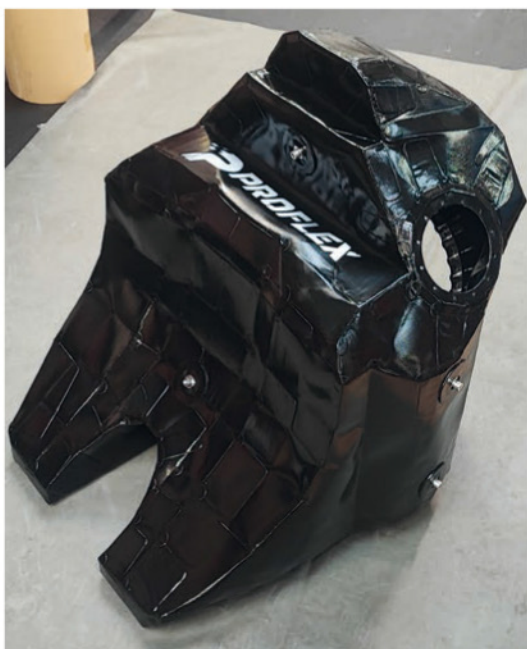
Above and below: two further examples of Proflex Formula 1 fuel cells, showing subtle modifications to the design to fit different chassis.
