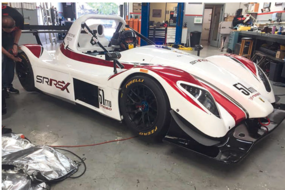
The second iteration of the SRe weighs 14.5kg more than the first, but has an additional 100bhp and a 12mph higher top speed
