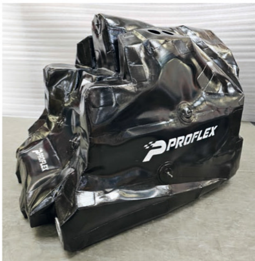
It may look like a crumpled bag, but this Proflex Formula 1 fuel tank is designed for maximum efficiency in the limited space available
