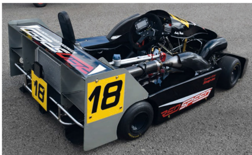
Bodywork material is free, with both carbon fibre and GRP used. Aerodynamic approaches differ, with a wide range of nose, rear wing and diffusers on show at any meeting, producing plenty of variety. A PVP superkart is shown here
