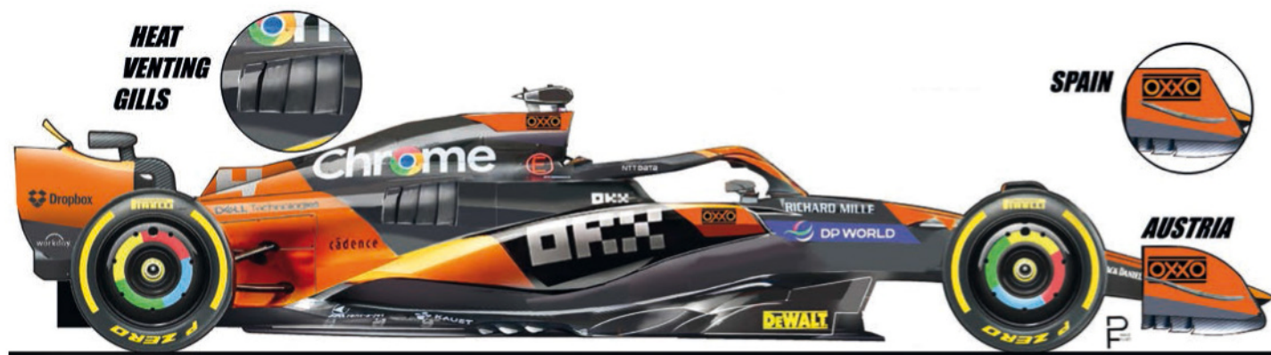
Subsequent updates during the European season built on the successful Miami package, and included new cooling layouts and revised aerodynamic features on the front wing end plates
