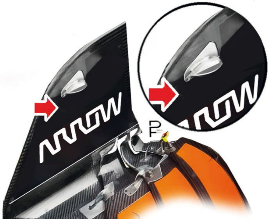
New front wing, sporting a smoother downward curve than before, was introduced in Austria to 'improve flow conditioning'
