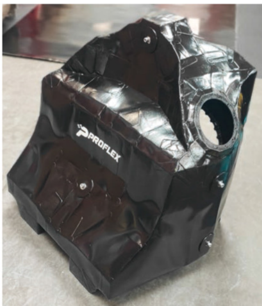
Above and below: two further examples of Proflex Formula 1 fuel cells, showing subtle modifications to the design to fit different chassis.
