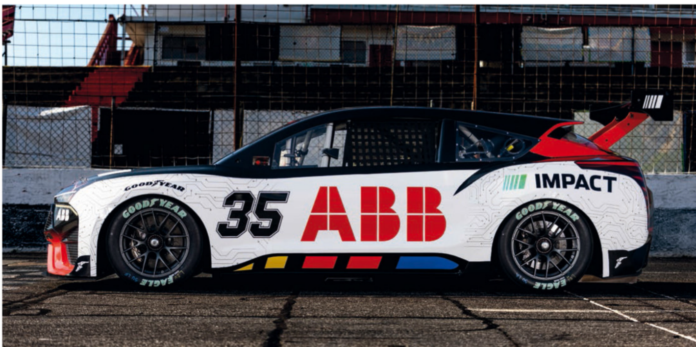
The design team says it reflected on current automotive purchasing trends in the US so, while the EV uses the Next Gen chassis, the body design is based on a generic Crossover Utility Vehicle
