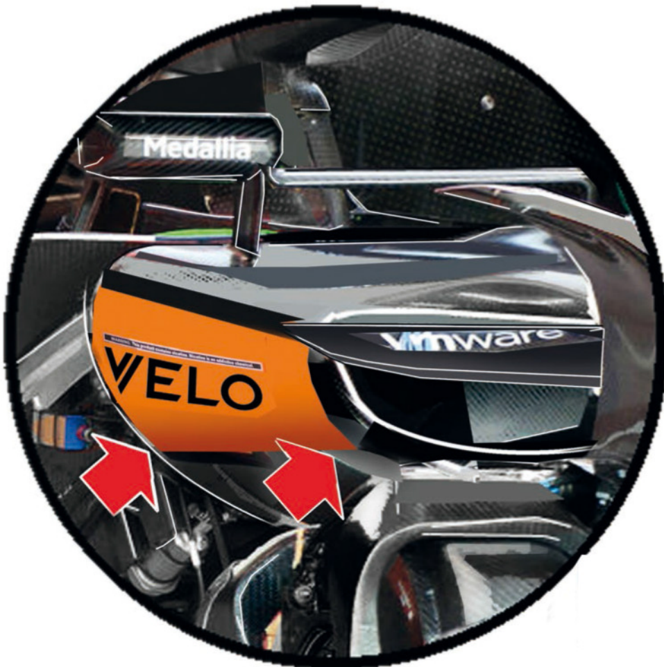
The upper section of the sidepod inlet had a much deeper undercut in the Miami upgrade package
