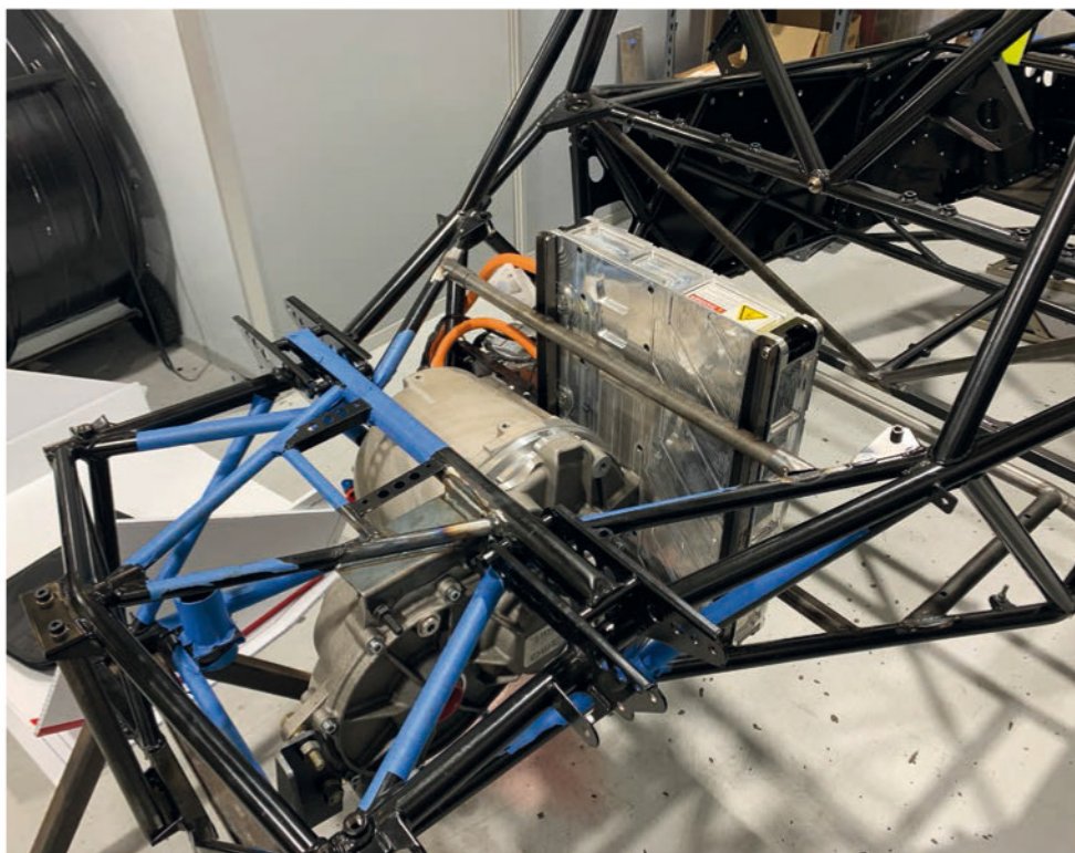
After the unfortunate incident at Sonoma, Hilleman rebuilt the car with a new chassis and improved powertrain with DC-DC converter
