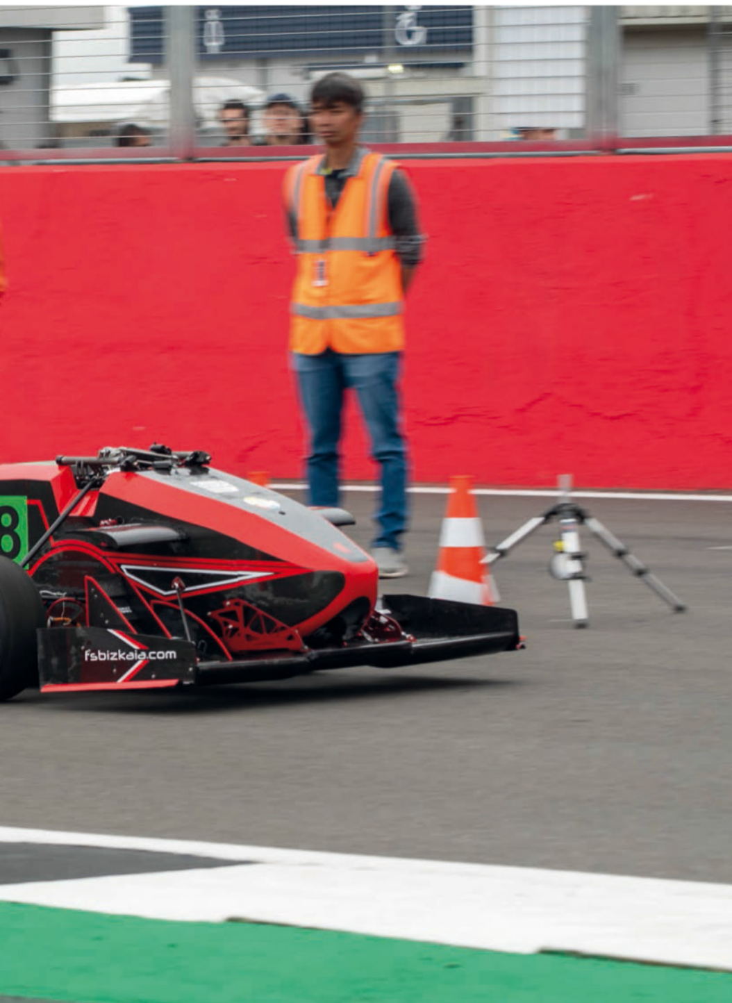
Coventry University opted to ditch its wings after it was unable to turbocharge its new, smaller Kawasaki 400cc unit
