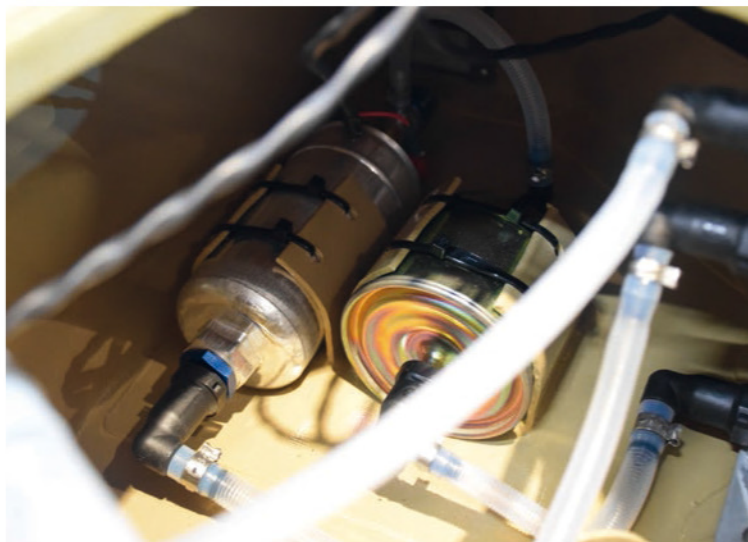
Almost all motorsport tanks now feature high volume, submersible lift pumps. This is a BTCC car unit
