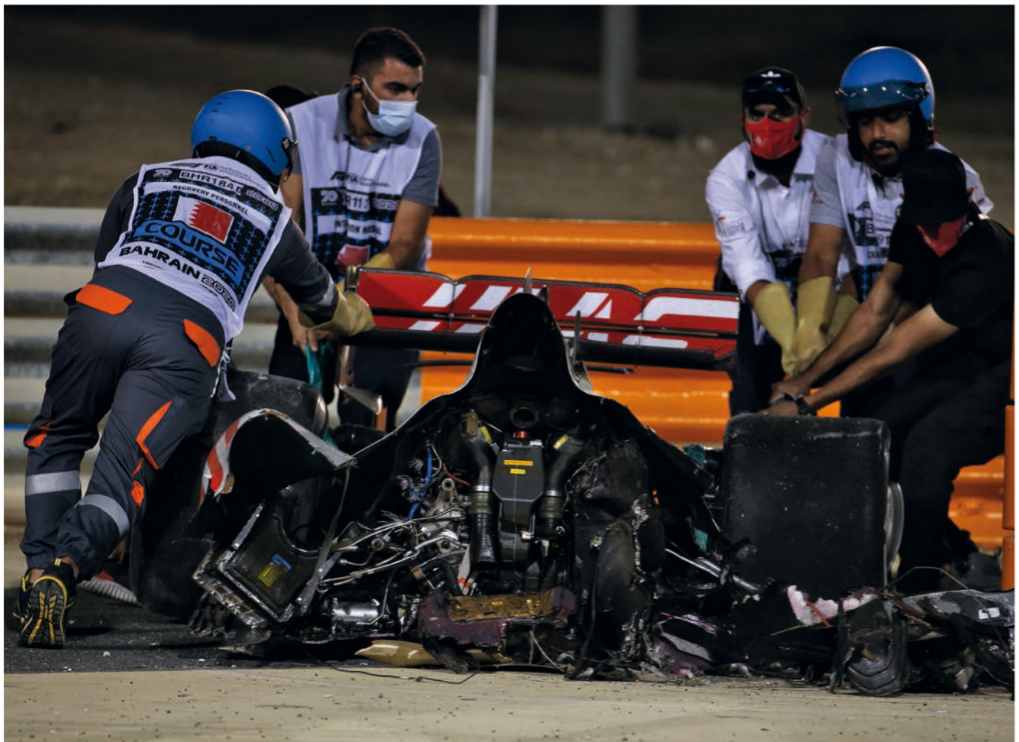
The investigation following Romain Grosjean's crash at the 2020 Bahrain GP concluded the impact ripped a fuel cell inspection hatch and supply fitting out of the tank, which led to the fire
