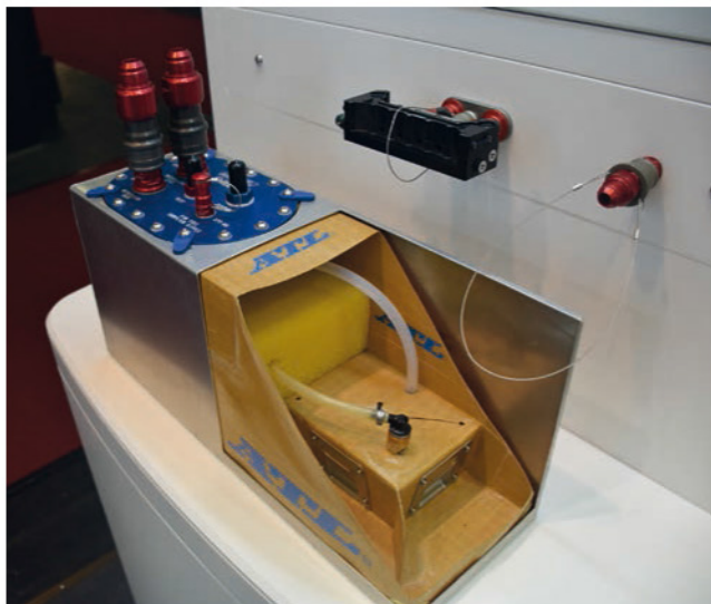
This cutaway of an ATL tank shows the inner compartments and reticulated foam filling
