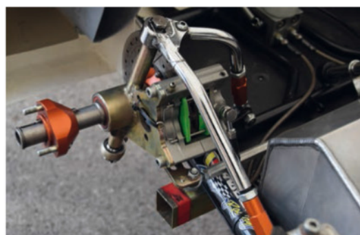
The frame is so much more than a chassis, as it must also provide the ‘give’ that would normally be the work of the suspension on a traditional racecar. Chassis tend to be made from high-grade steels such as T45; carbon is not allowed
