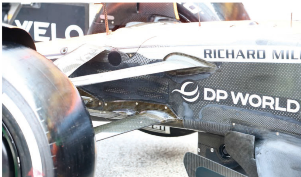
A comparison between the 2024 (above) and 2023 (below) front suspension clearly shows the change in position of the upper wishbone rear leg inboard mounting point, which has moved rearwards and down. The steering track rod was also moved rearward
