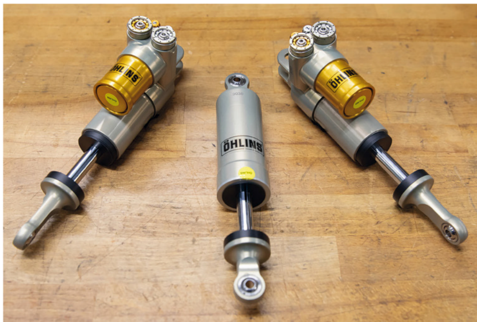
The main difference is the new front units, type number DR30, use both oil and gas for control, whereas the old TTR30s used only oil
