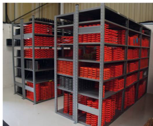
There are between 150 and 200 components in an R53 damper, and pretty much every one of them is made to the company's own design and specification, and that includes the coil springs
