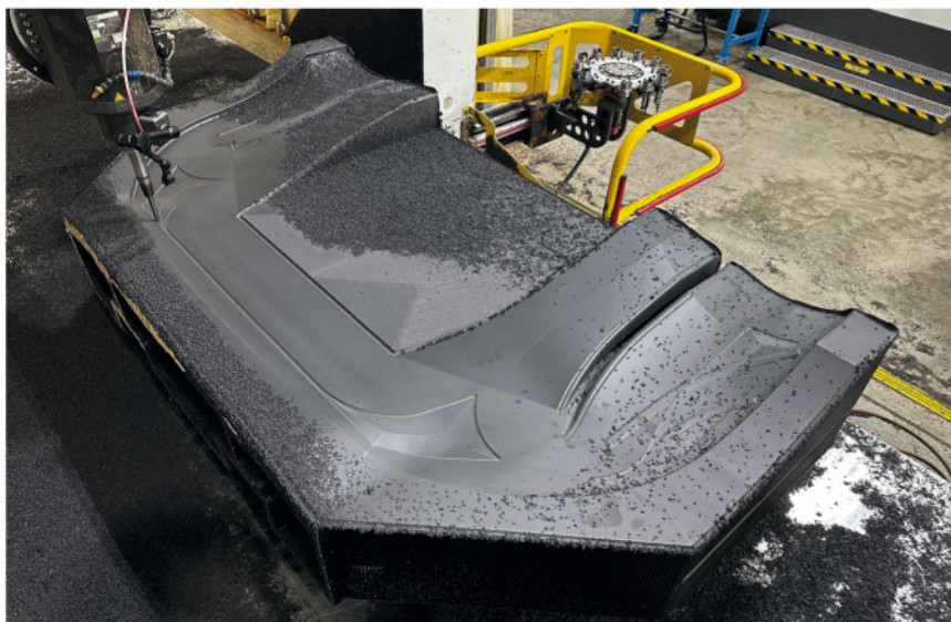
Airtech recycled, 3D-printed, composite mould tool
