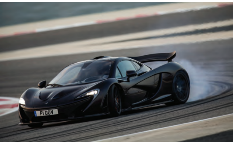
ABOVE & BELOW With active aero forbidden for so long in F1, road car technology outstripped it. The irony wasn’t lost on McLaren, whose P1 (above) features moveable front and rear wings and a Drag Reduction System. Porsche’s 918 Spyder (below) includes an adjustable front diffuser in an armoury of moveable devices
