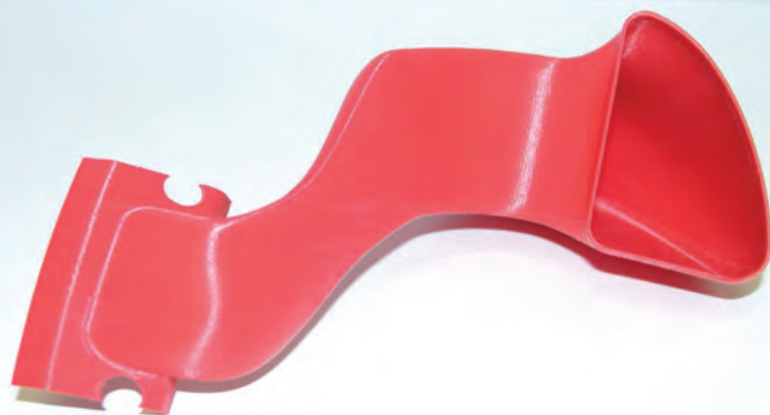
ABOVE & BELOW A brake duct (above) and dive plane, both 3D printed in thermoplastic material, used for track testing
