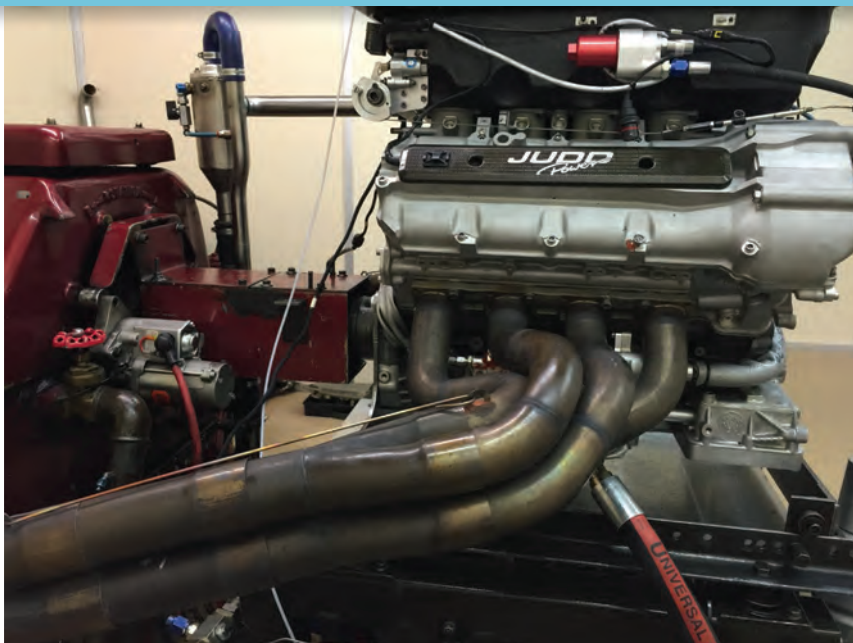
ABOVE & BELOW Judd's HK V8 LMP2 engine on the dyno (above) and being worked on in CAD
