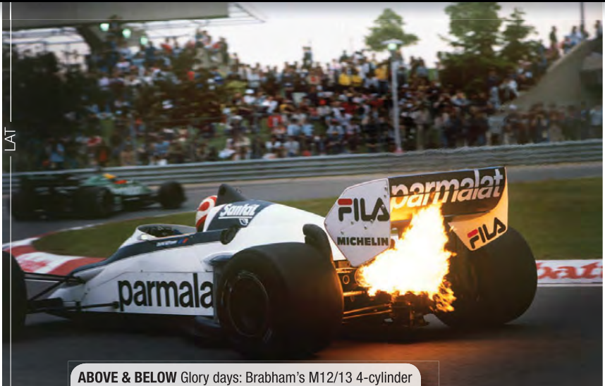
ABOVE & BELOW Glory days: Brabham's M12/13 4-cylinder inline turbo boasted up to 1,300 bhp in qualifying trim
