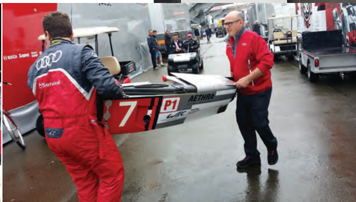
ABOVE & BELOW Audi's ability to get a damaged car back on the track quickly is a feature of its Le Mans success. This sidepod, complete with radiators for a quick change, highlights its approach
