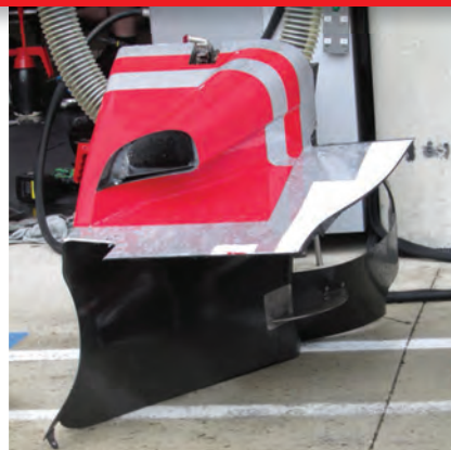
ABOVE Audi's front fender with integrated mirror and turning vane
