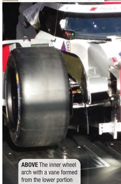
ABOVE Audi's front fender with integrated mirror and turning vane
