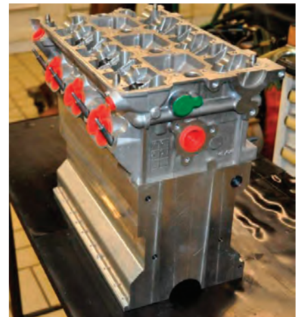
ABOVE & BELOW The 1.6-litre, three-cylinder, turbocharged engine is a bespoke WR unit. The only production-derived component is a modified cylinder head from the PSA Group
