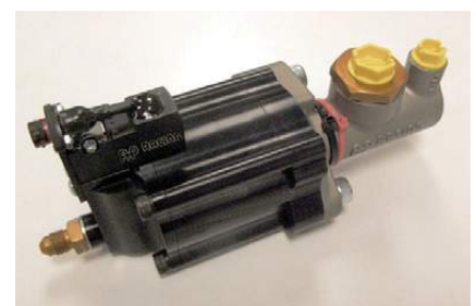
ABOVE AP Racing's external clutch release system that aids race marshals when moving stricken cars
