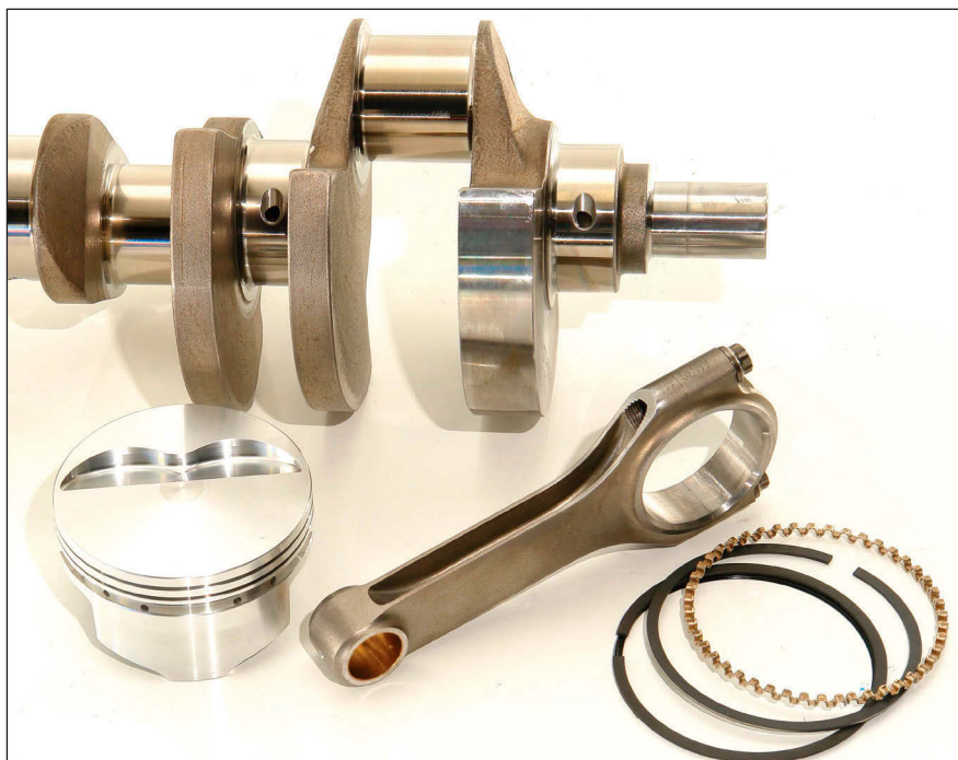
ABOVE Increasing the engine's displacement by virtue of a longer stroke (stroker) crank is a popular way to increase torque output. Unfortunately it is often the case that as little as 50% of the increased displacement is fully utilised because the cam selected does not reflect the engine's new gas dynamics characteristics. Matching the cam's event timing to the engine's new requirements can easily double the torque gains of a stroker crank
