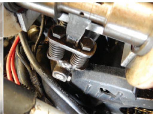
ABOVE & BELOW The University of Moratuwa car featured a home-made solenoid shift mechanism, above left, designed and built without the help of CAD, FEA or automated machining. Above right, the actuator connecting solenoid to gear shifter
