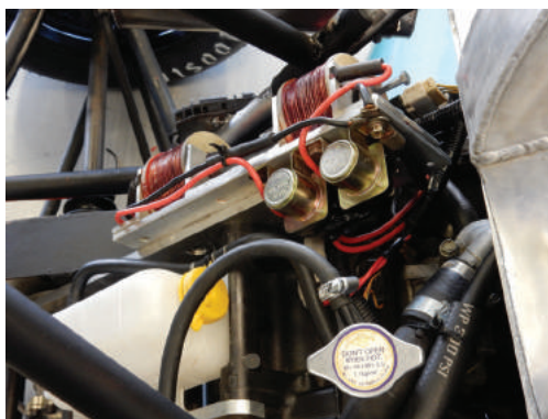
ABOVE & BELOW The University of Moratuwa car featured a home-made solenoid shift mechanism, above left, designed and built without the help of CAD, FEA or automated machining. Above right, the actuator connecting solenoid to gear shifter
