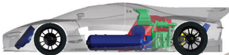
ABOVE & BELOW The H2 SPEED, seen here in both CAD and CFD, features an electric engine powered by a fuel cell fed by three hydrogen tanks
