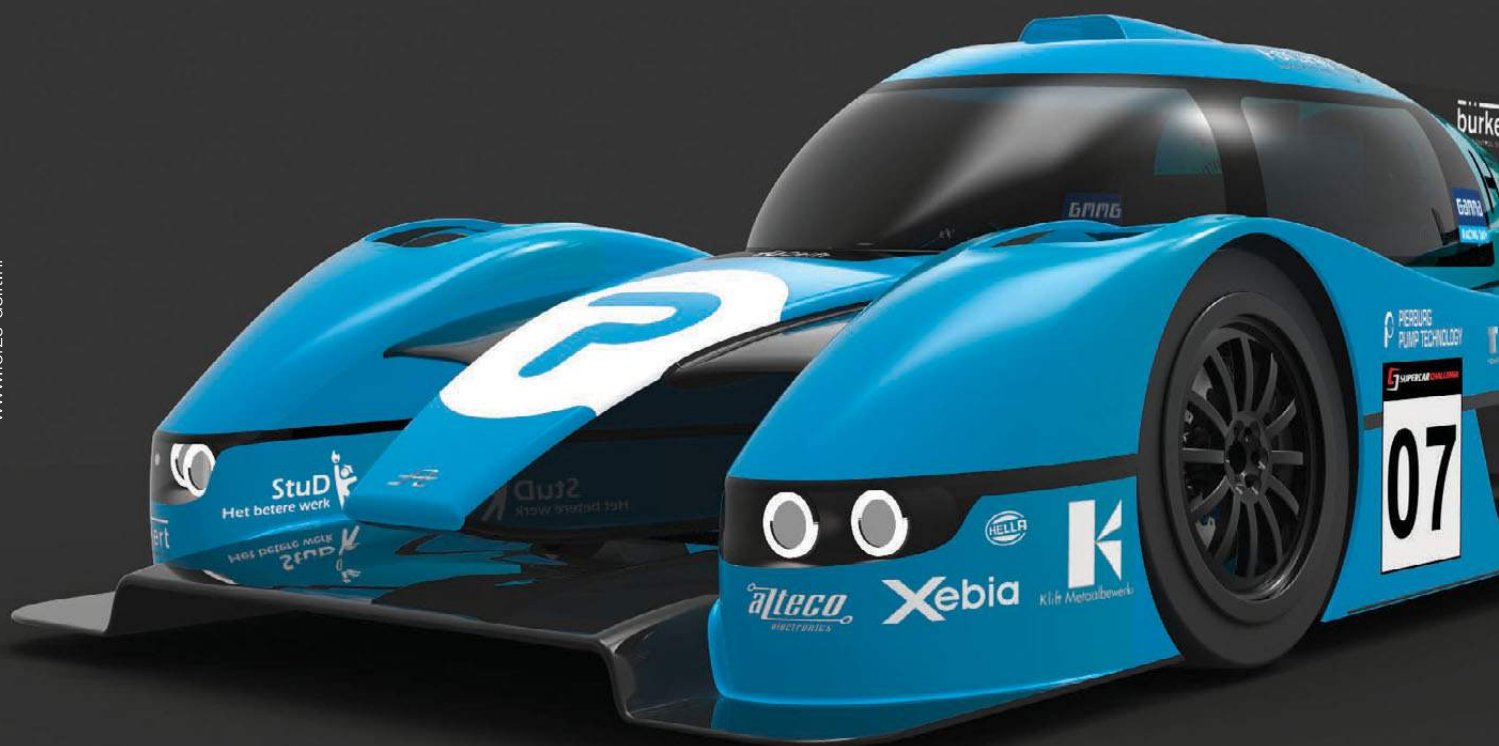
ABOVE Forze VII takes its carbon fibre monocoque from an Adess LMP3 car, enabling the students to focus on the powertrain
