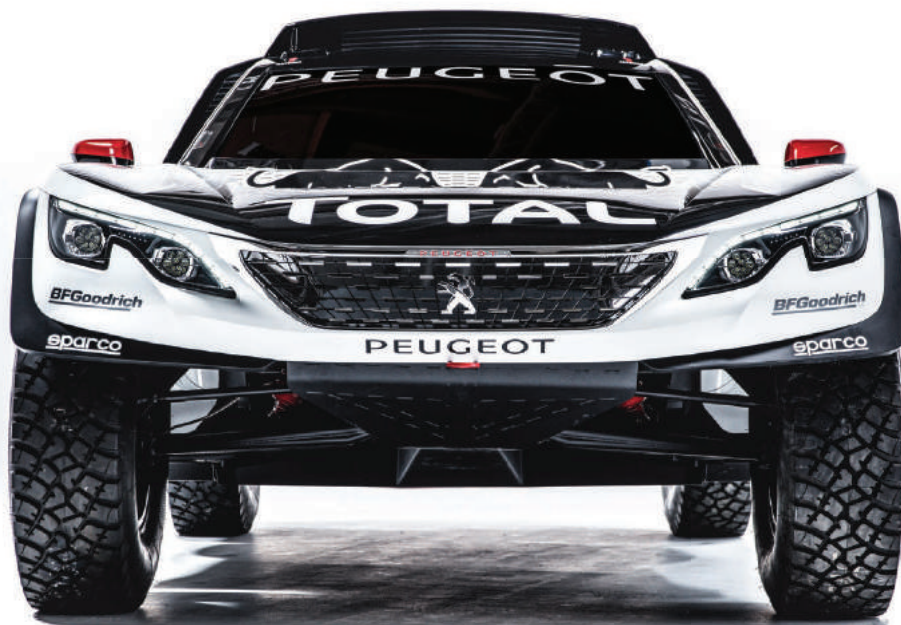
ABOVE The car maintains its predecessor's short front overhang, aiding the ability to climb steep inclines
