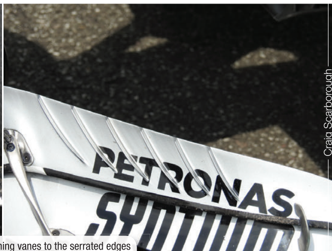
ABOVE & BELOW From its turning vanes to the serrated edges of its wings, Merc's W07 was more complex than its rivals
