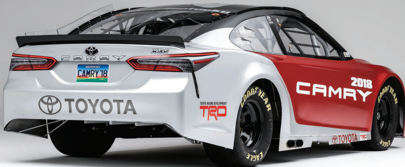
ABOVE & TOP Studio views of the new 2017 NASCAR Toyota Camry, painstakingly designed to be well positioned in the performance 'box' dictated by the rules. Note in particular the more dramatic nose treatment and also the more prominent wheelarches
