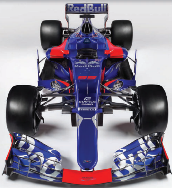
ABOVE & BELOW Both Toro Rosso and Mercedes have adopted solutions that have the top outboard wishbone mounted above the wheel rim and alongside the inner tyre sidewall
