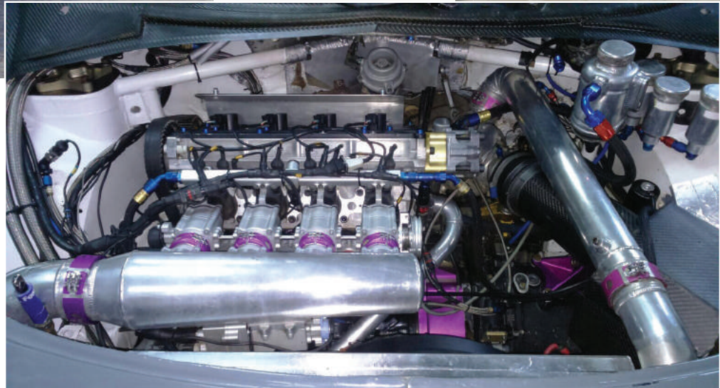
ABOVE & BELOW The engine for the Citroën DS3s of a battling Petter Solberg and Liam Doran started with a cast iron cylinder block from PSA's diesel range
