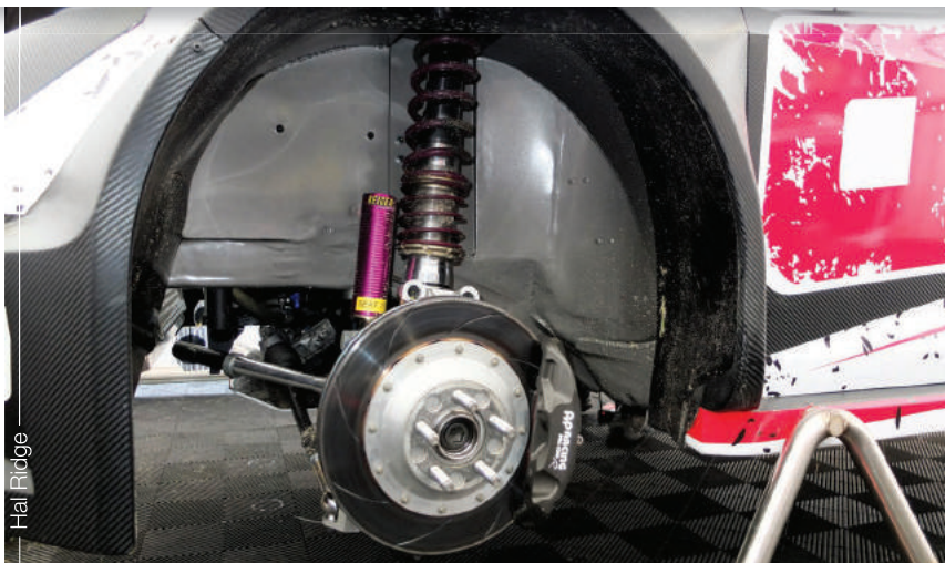
ABOVE & BELOW Engineering opinion is split over suspension choice. One team, Münnich Motorsport, even went so far as to run a MacPherson front and double-wishbone rear
