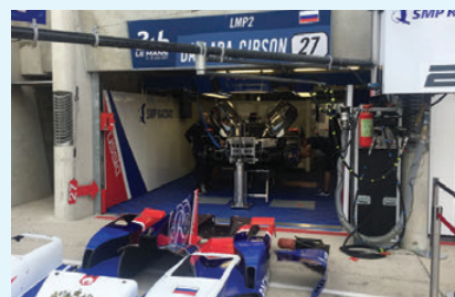
ABOVE The Breda Racing air jack was much in evidence and this shot captures part of the set up equipment (zimmer) specially manufactured for the Dallara LMP2 2017 car
