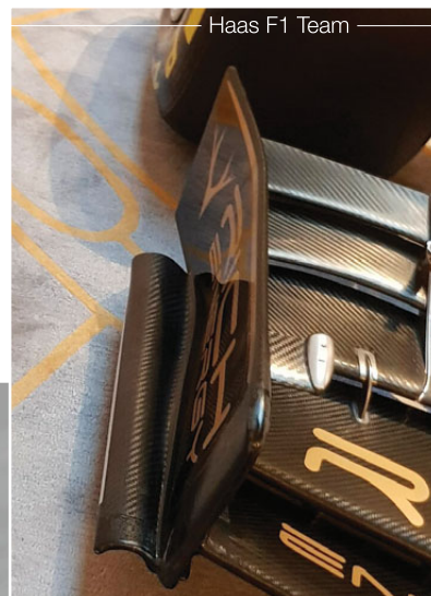
ABOVE Haas, like some others, stops the rolled footplate short of the end of the endplate
