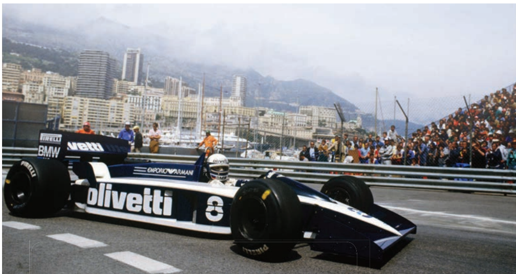
ABOVE & BELOW The Brabham BT55 was labelled a flop in 1986, with its lowline concept handicapped by the packaging of BMW's four-cylinder engine
