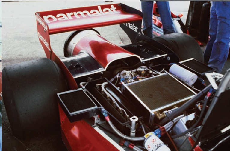
ABOVE & BELOW The BT46B 'fan car' took ground effects to new extremes. It was never actually banned, insists its creator, although paddock pressure led to its withdrawal after a dominant victory in the 1978 Swedish GP
