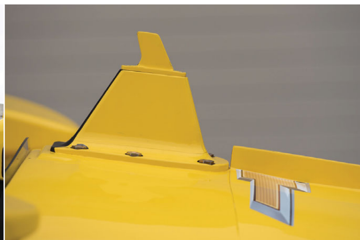
ABOVE & BELOW The AFP device, a 3-inch-tall titanium component manufactured by Dallara that is positioned in front of the cockpit along the chassis centreline, will be utilized by all teams for the remainder of the 2019 season
