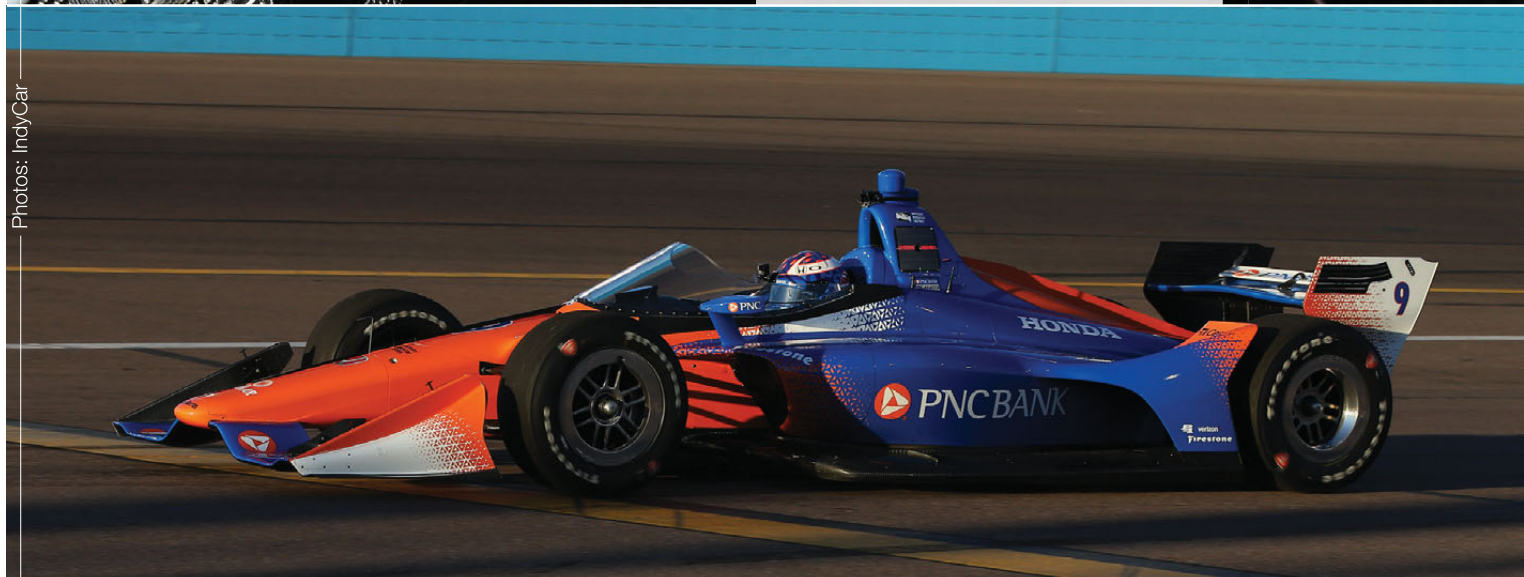
ABOVE & BELOW An experimental windscreen constructed by PPG was tested both at Indianapolis by Josef Newgarden (above) and at Phoenix by Scott Dixon (below). Cooling and buffeting issues were reported
