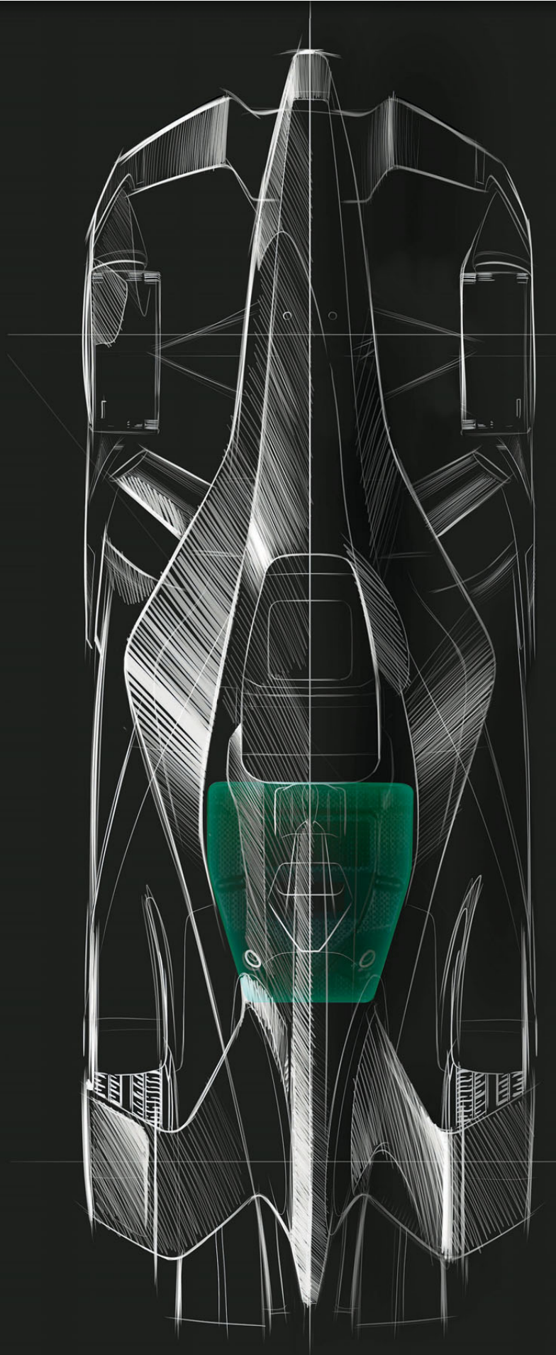
ABOVE How the trapezium battery pack fits into the Formula E racecar
