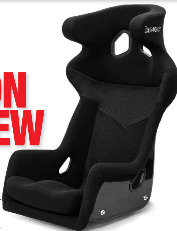
ABOVE Racetech's new RT4100 seats are able to safely accommodate broader drivers, while remaining narrow enough for most cockpits
