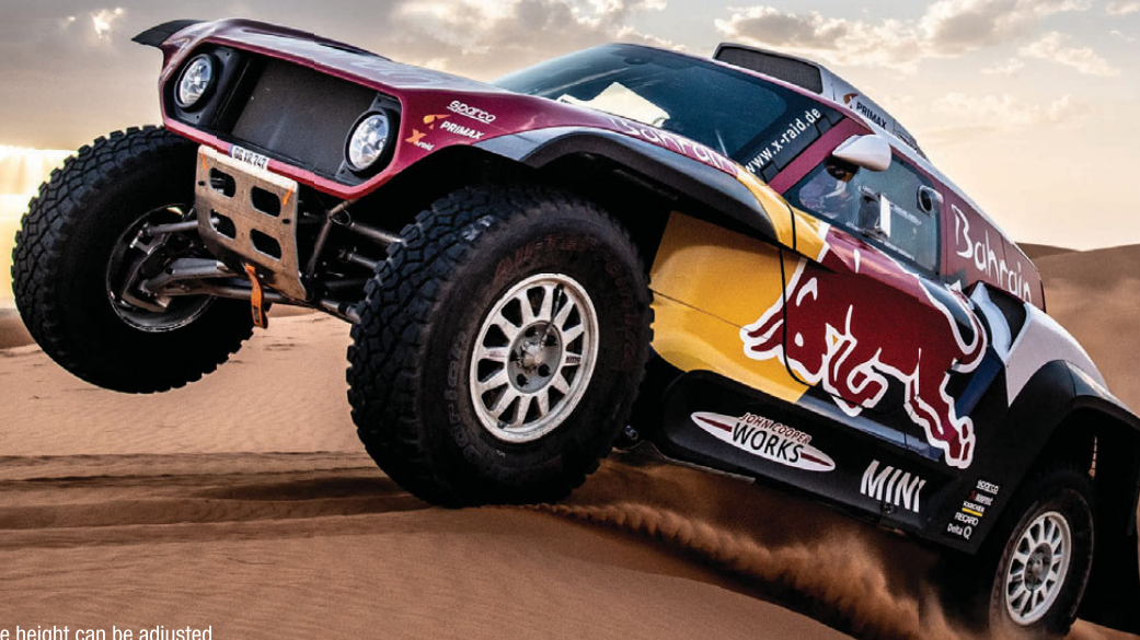
ABOVE Ride height can be adjusted over a range of nearly 50 mm, offering a low-slung setup or extra clearance
