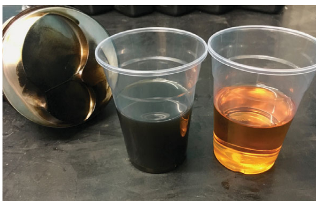
LEFT Combustion blow-by gases contaminate and chemically degrade motor oil
