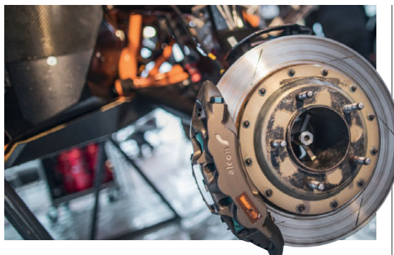
LEFT The current car features Alcon four-piston callipers and 355 mm vented discs all round
