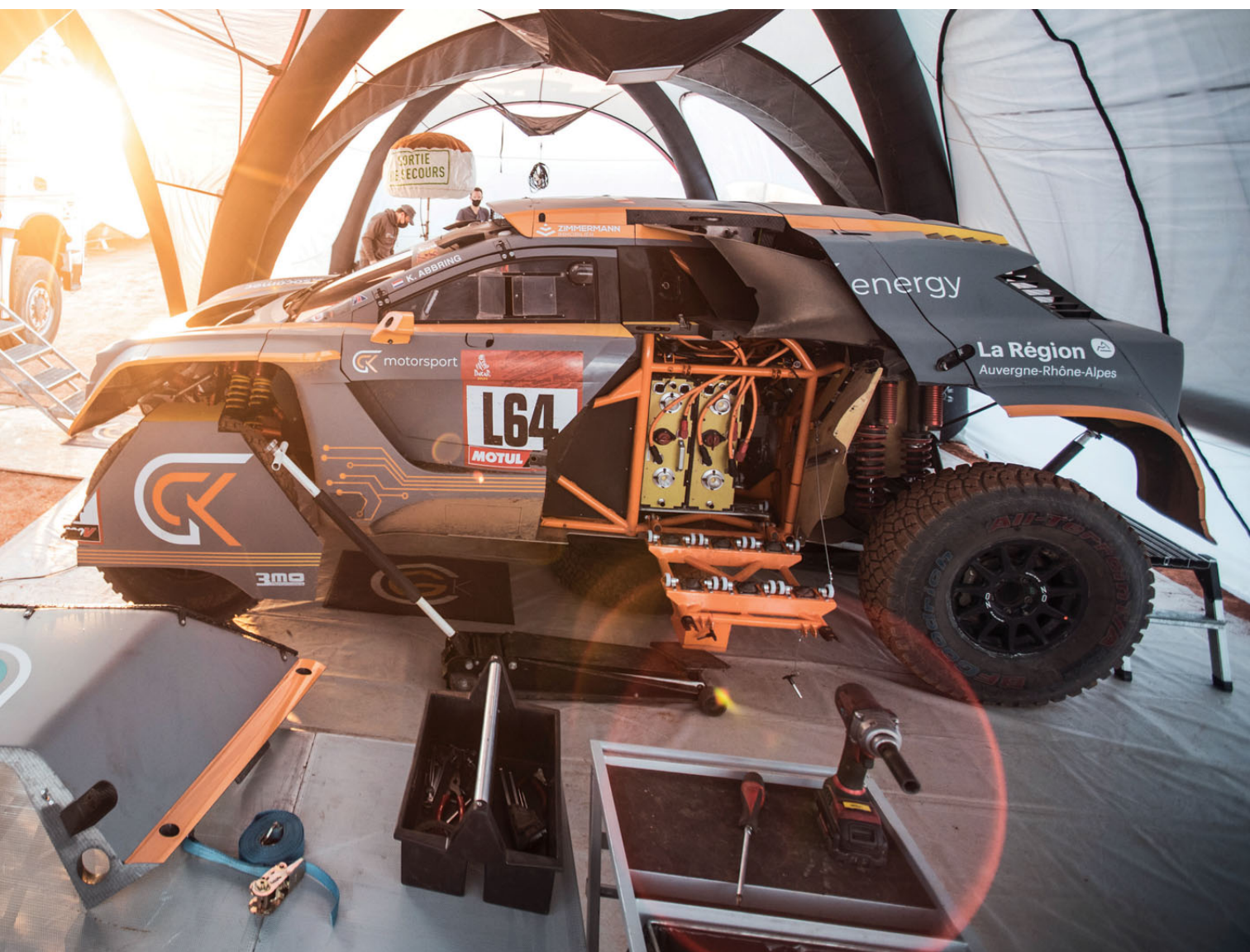
BELOW The rear of the Peugeot chassis has been redeveloped and redesigned to accept the motor, battery and gearbox
