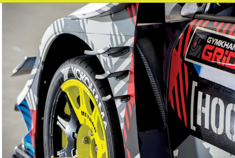
ABOVE The aero detail was validated in wind tunnel testing
