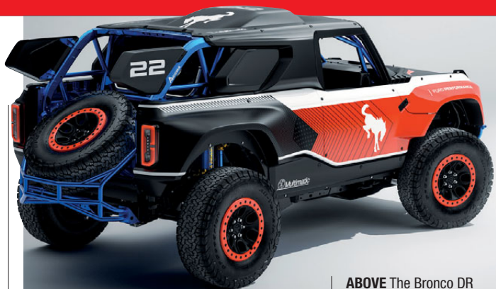
ABOVE The Bronco DR features the first application of Multimatic's Positional Selective Damping technology
