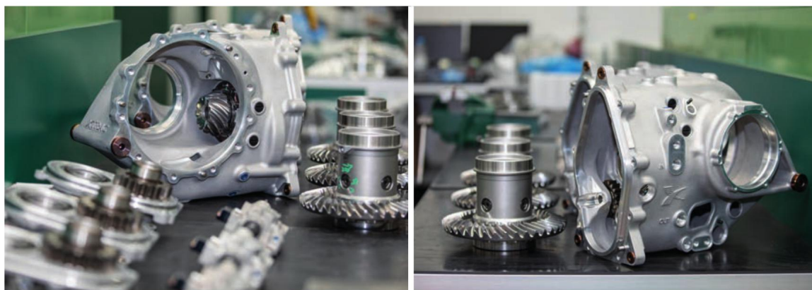
LEFT The transaxle includes Xtrac's own Salisbury-type torque biasing differential
