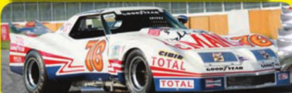
Greenwood "Spirit of 76" LeMans Corvette. Ran Kinsler crossram manifold with Lucas mechanical metering.
