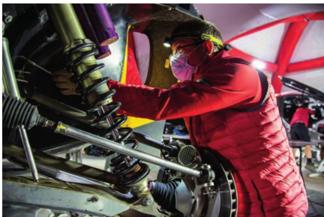
LEFT & BELOW Suspension travel was a key change over the car's predecessor, with wheel articulation up from 280 mm to 350 mm
