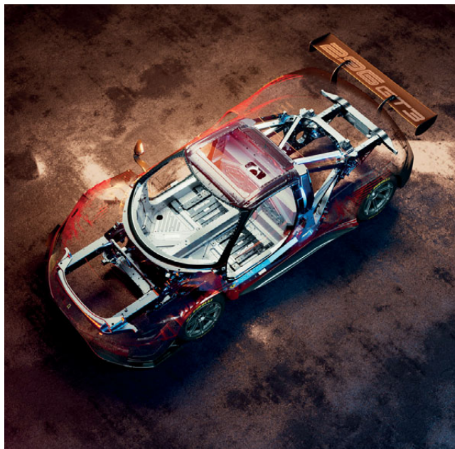
LEFT Both ends of the car are built up on detachable subframes for ease of maintenance
