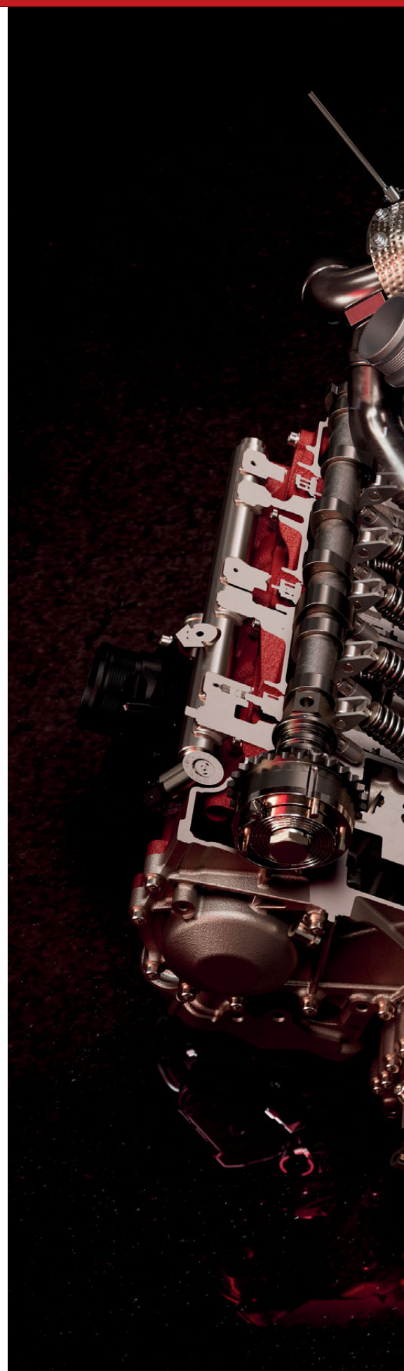
RIGHT The wide-angle configuration of the engine will allow the turbos to be housed inside the vee for more effective packaging
