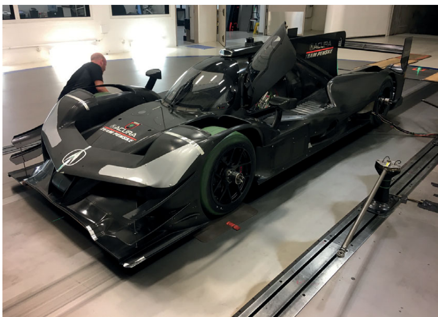
BELOW Aero development of Acura's styling vision resulted in the distinctive hammerhead seen here on the DPi car
