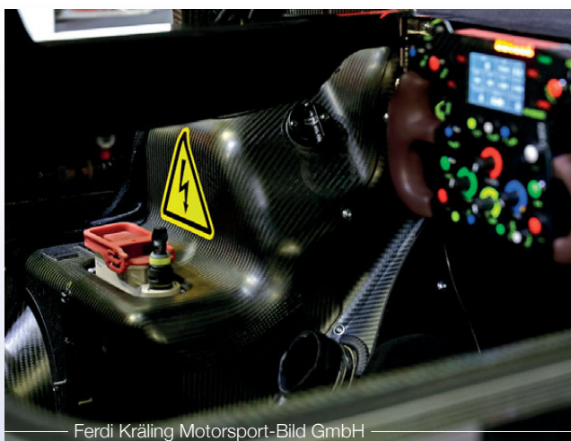
LEFT The Audi R18's hybrid system battery, seen in 2016
