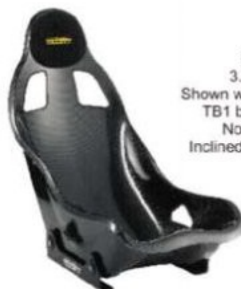
B5 Narrow and can be used with road belts. Shown with optional Dinamica suede pads. Non FIA
